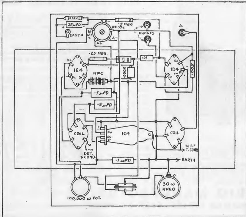
right-angle bracket for mounting the r.f. valve under the chassis can be bolted in place next, followed by the audio choke.
