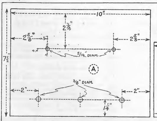
Sketch A (left) shows dimensions for preparing the front panel, B and C, for the aluminium shield partitions, while D gives details of the bracket for mounting the r.f. valve under the chassis. All flanges shown should be 3/8 in. wide. The chassis layout is shown elsewhere.
