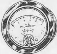
TRIPLETT 1M/A meters, suitable for inclusion in the 9 range assembly, 3½ in. bakelite case, 2½ in. dial face. Special, 36/-
