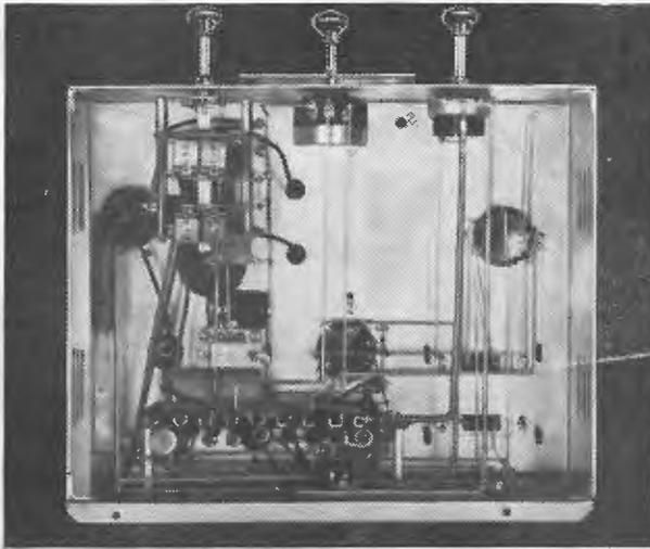
Above: An under-chassis view of the completed kit, showing the simplicity of the assembly and wiring.
