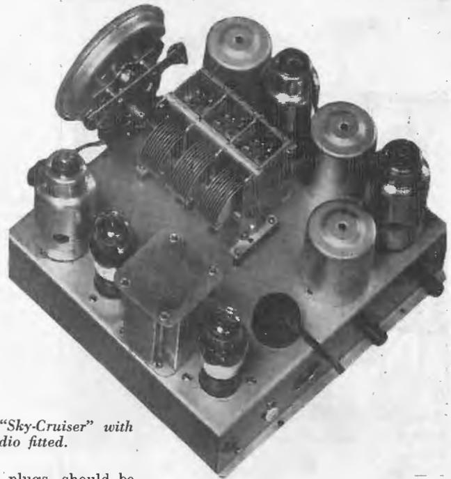
A rear view of the "Sky-Cruiser" with class "B" audio fitted.
