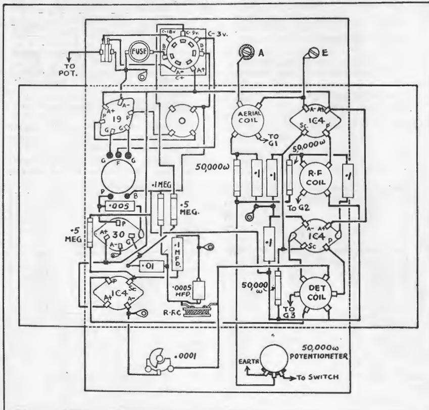
The complete wiring of the five-valve model is shown in this sketch.
