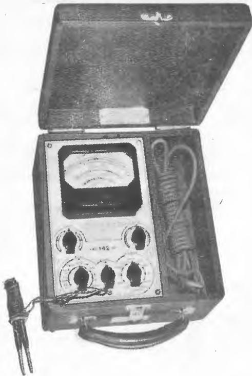
This new Model 142 Calstan Uni-Tester is an a.c./d.c. multi-meter that as well as covering the usual current, voltage and resistance ranges, also gives direct measurements of impedance, inductance, capacity and output (in decibels). Provision is also made for checking electrolytic condensers of all types.
