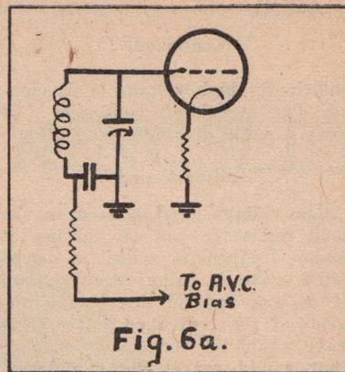
constant following the same laws as previously explained. It is desirable to include the resistances in the circuit to prevent undesirable coupling between the R.F. and I.F. stages which may produce instability.
