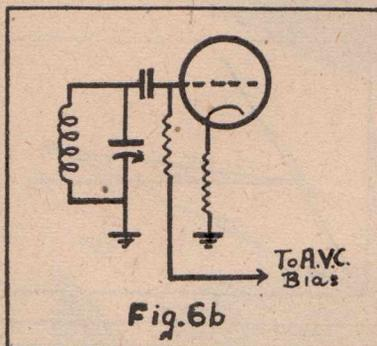
duced by feeding the final I.F. amplifier with a reduced A.V.C. voltage tapped off the A.V.C. load resistance.
