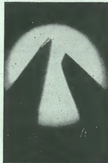
This micro-photograph shows how a gramophone needle looks after playing through one recording. On the left is a new needle for comparison.
