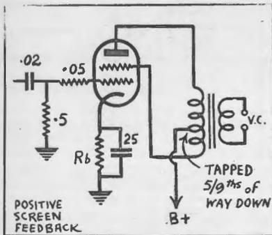
It is to be noted that the negative feedback used is quite independent of any feedback over the output stage. In fact there must be part of the circuit over which there is no feedback and the volume control is connected in this section. If feedback were applied over the volume control, the amount of feedback would be varied and the control would act only over a small portion of its range.
