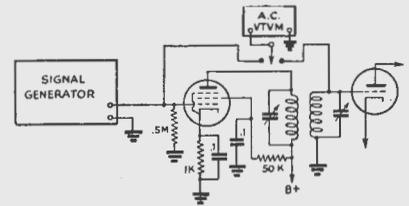
Fig. 3—A simple single-stage test circuit for measuring selectivity. The values shown are not critical. Normal receiver voltages should be employed.
