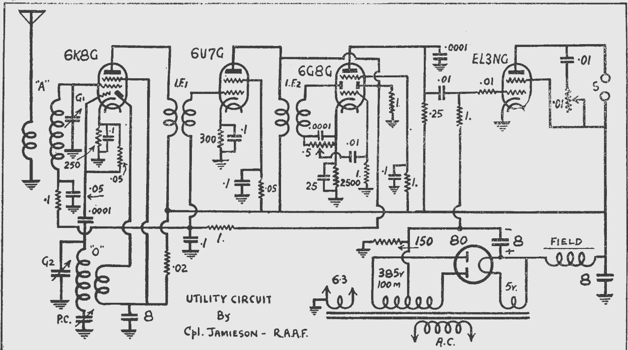
put on weak stations. Where in sets using say a 6F6G the output would hardly fill a good sized room on a weak signal, the EL3NG would make good room level possible.
