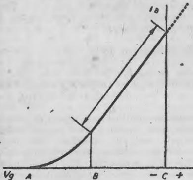
Fig. 4.—A typical anode current grid coil curve.
