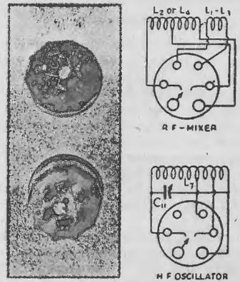
Fig. 2 — Pin connections for the r.f. and h.f.o. plug-in coils. The bottom views of the coil forms in the photograph show the bandspread switching arrangement. The screw head completes the connection between either pair of pins, depending upon its position.
