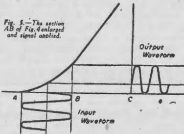
Fig. 5.—The section AB of Fig. 4 enlarged and signal applied.
