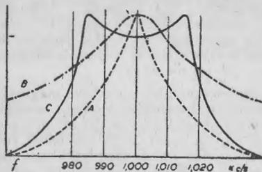
Fig. 1.—Shows the effect of selectivity on L.F. frequency response
