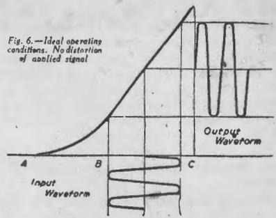
Fig. 6.—Ideal operating conditions. No distortion of amplified signal.
