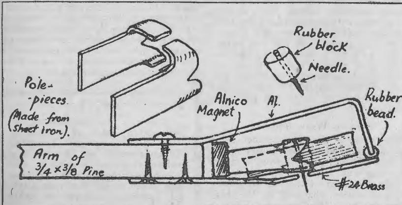
A rough sketch of the pick-up assembly, with illustrations of the pole pieces and the suggested needle mounting.
