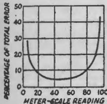
Fig. 7—Curve showing resulting inaccuracies in resistance measurement when an error of as little as one per cent is made in the meter reading.
