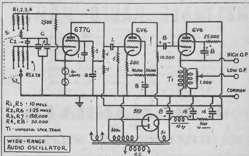
Circuit schematic for the handy audio oscillator.
