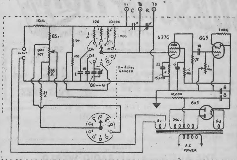
Schematic of the bridge for testing resistances and condensers
