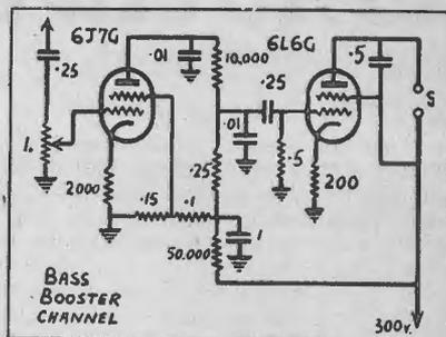
Circuit for an amplifier to handle only the lower audio frequencies.
