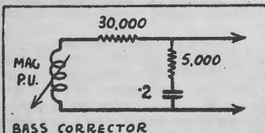
Suggested circuit arrangements for a suitable bass corrector and a scratch filter to allow worn records to be played.
