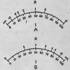
Fig. 3 - Typical ohmmeter scales applied to a milliammeter. The reversed scale at A occurs when the unknown resistance is connected in series, while the scale at B is of the type which results when the unknown resistance is connected in parallel with the meter.
