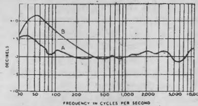
Fig. 4. Response curves of pick-up and amplifier: Curve A, amplifier with restricted negative feedback in the bass; Curve B, amplifier with tone-correcting stage.
