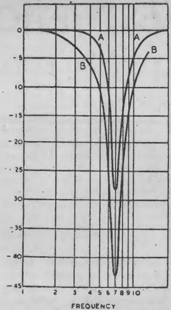
Fig. 2. Response curves of rejector circuit. Frequencies are marked in kilocycles.
