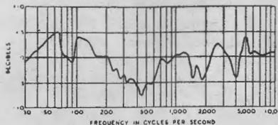
Fig. 5. Response curve of pick-up, amplifier and speaker.
