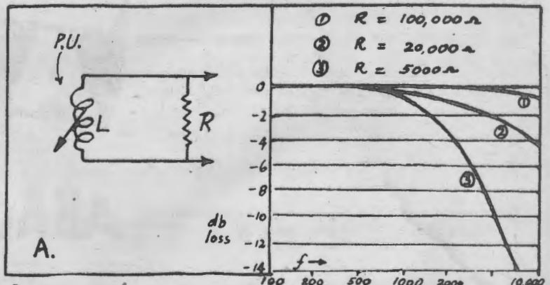
Attenuation of "Highs" by Resistor Shunt.
