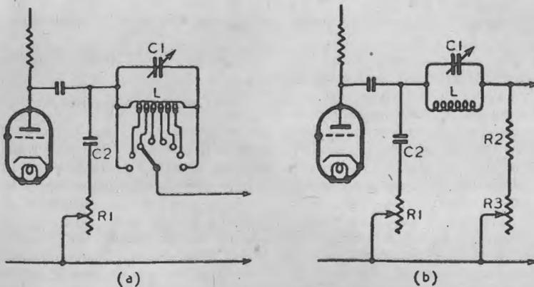
Fig. 1. Two forms of rejector circuit for introducing a variable sharp dip in the response curve of the amplifier.
