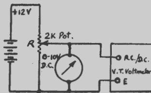
FIGURE (7) D.C. Calibration
