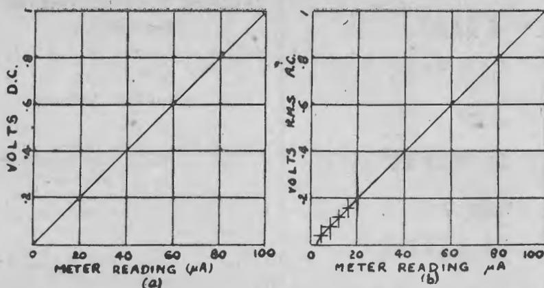
FIGURE (5) Calibration Curves (a) D.C., (b) A.C.
