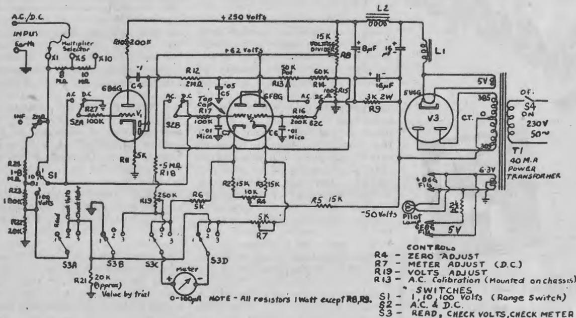
FIGURE (4) Circuit Diagram of Linear A.C./D.C. V.T. Voltmeter.
