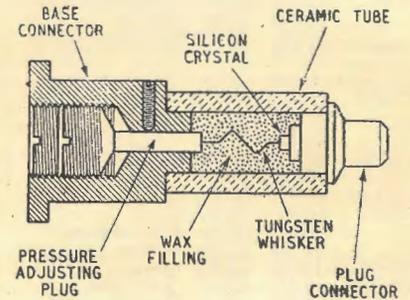
its early prototypes. As the sectional drawing in Fig. 1 shows the crystal and tungsten catswhisker are contained in a small ceramic tube closed at each end by brass plugs and completely filled with wax. This form of construction results in a mechanically robust device in which the contact is quite undisturbed by normal shocks.
