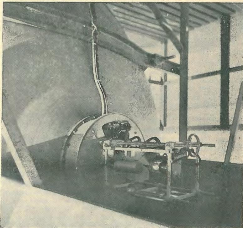
This might appear to be a modern example of application of a Magnetron oscillator and parabolic reflector for UHF's, but it isn't. This picture was taken at Lympne, (England) in 1936, and was the English end of a 60 centimetre telephone link with France. In Wellsian fashion it was truly a forerunner or "things to come."
