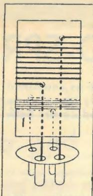
This sketch illustrates how the windings are put on the three plug-in coils that are needed to cover from 19 to 90 metres. Details of the number of turns for each coil are given elsewhere.
