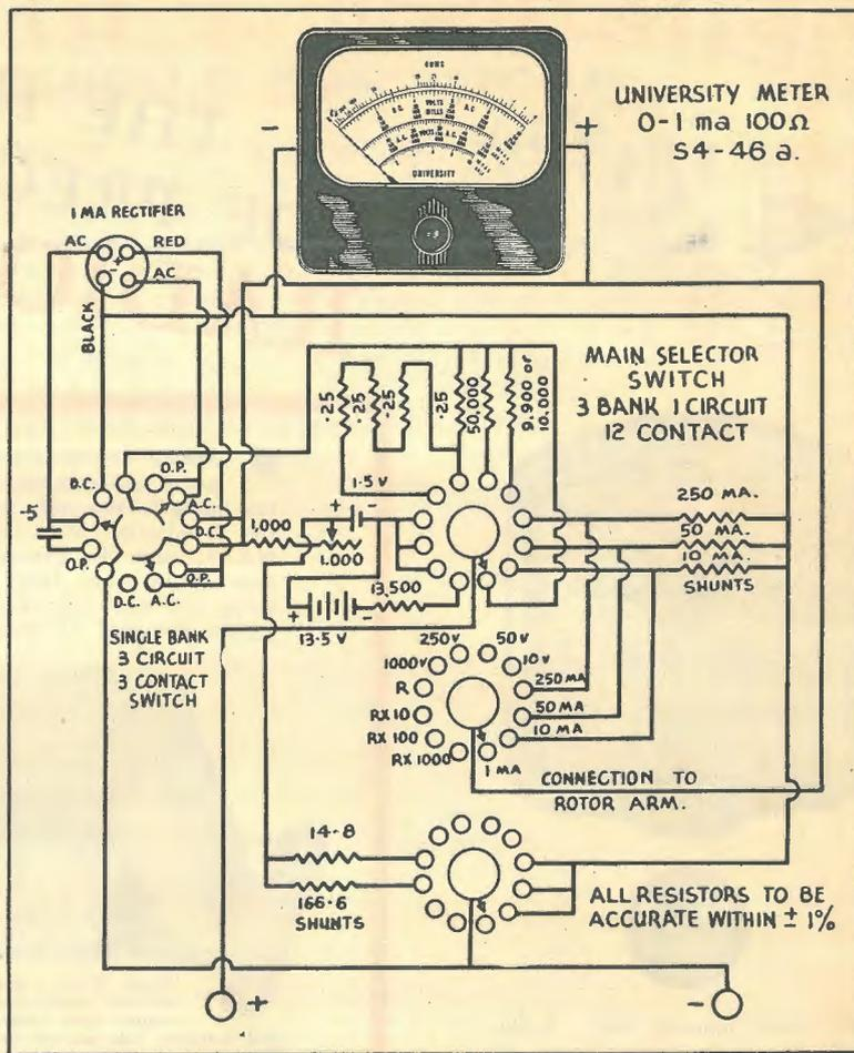
Circuit of the meter, showing the switching arrangements.
