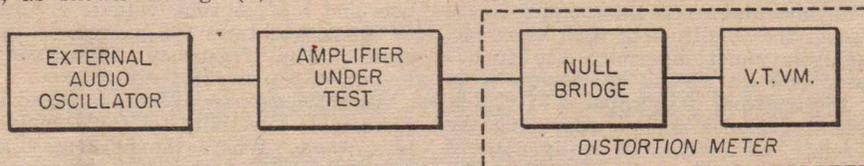
TEST SET-UP USING DISTORTION METER
