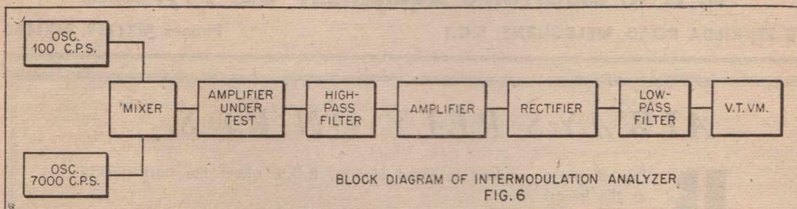
BLOCK DIAGRAM OF INTERMODULATION ANALYZER
