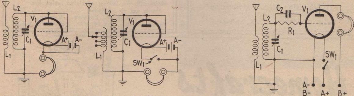
These two circuits show how a crystal detector can be replaced by a triode valve connected as a diode. All that is needed is a battery to light the filament, and a valve socket. For old-fashioned 2-volt valves a 1½ volt torch cell can be used, and for 4-volt valves a 4½-volt torch battery. The left-hand circuit shows Crystal set No. 3 altered to use the valve, and the right-hand one, crystal set No. 2. In the latter a switch has been added to turn the valve filament on and off.
