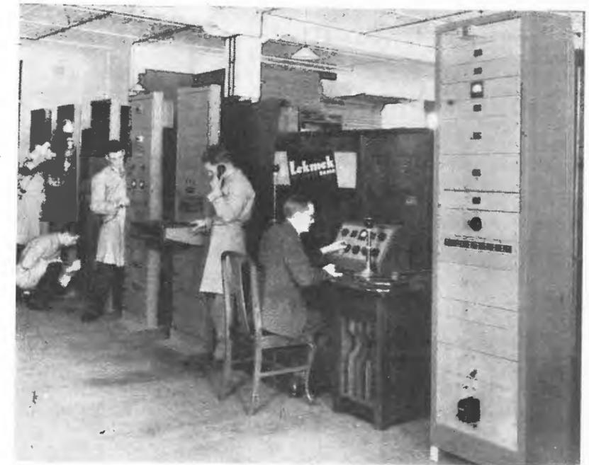
Almost ready for shipment. Some of the racks for new "A" Class Station on the left of photograph, and complete Amplifier Cabinet and Announcer's Control and Desk for new Mudjee Commercial Station on the right.
