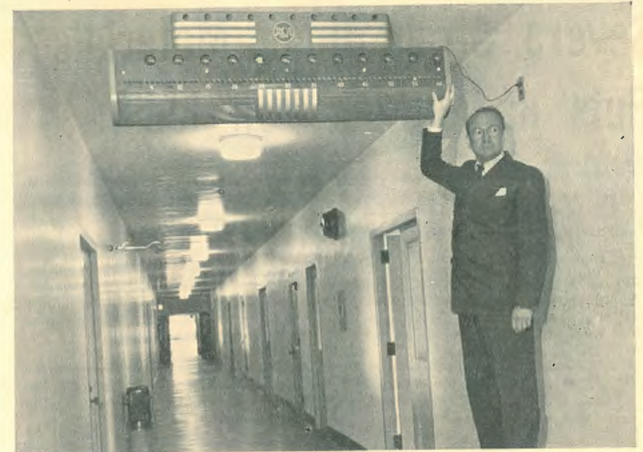
A novel electronic clock is installed in the new R.C.A. Laboratories. This ultra modern timepiece equipped with more than 170 electronic tubes counts the 60 cycle pulsations of electric current, and indicates that count in terms of the seconds, minutes and hours by means of lights. It has no moving parts, no motors, wheels, main spring or hands. Scientists say it may form the basis of the household clock of the future. Blinking lights "tick off" the minutes on the line shown from 1 to 60, while other lights denote the seconds and hours. Pictured here with the clock, which shows the time to be 5:55, is Dr. V. K. Zworykin, Association Director of Laboratories, who with his staff developed it.
