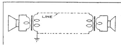
A simple intercom. system can be wired up using two modern permag. speakers.
