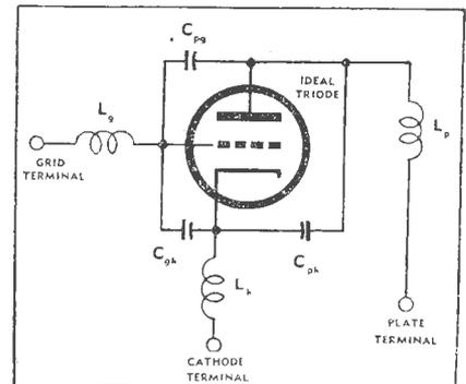
Fig. 1.—Equivalent circuit of a triode at U.H.F.
