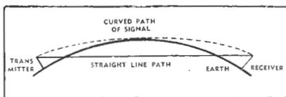
Fig. 2.—This diagram shows the refraction path of an F-M signal.
