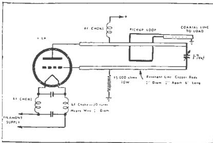
Fig. 4.—The ultra-audion oscillator circuit.
