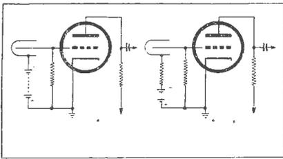
Fig. 4.—Two types of quenching circuits—on the left the Neher-Pickering circuit and on the right the Neher-Harper circuit.
