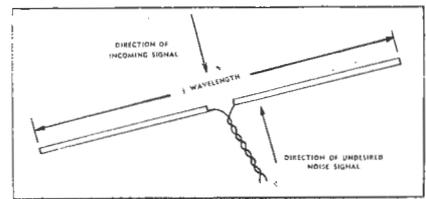
Fig. 5.—Signal response of a half-wave dipole.
