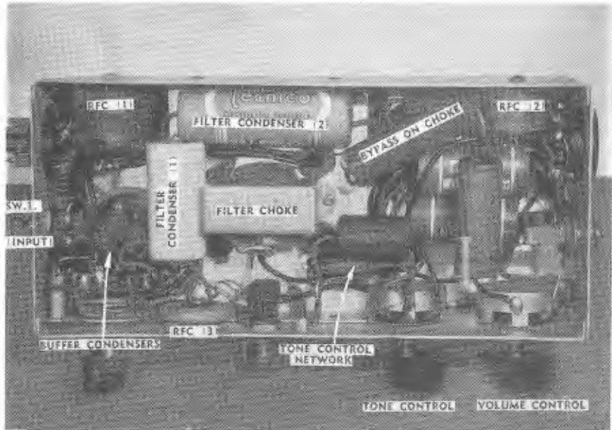
This underchassis photograph shows how most components were fitted in. This layout keeps all leads to a minimum, thus reducing one potential source of interference.
