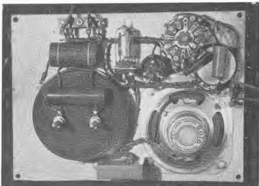
A close-up of the completed wiring. The various leads are tied together for neatness, and are made as short and direct as possible.
