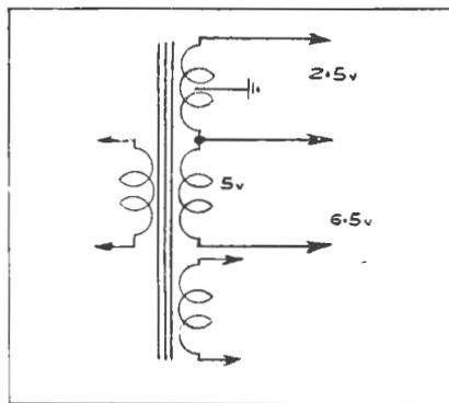
This is the method of connecting the 5.0 and 2.5 volt windings to obtain 6.3 volt output.
