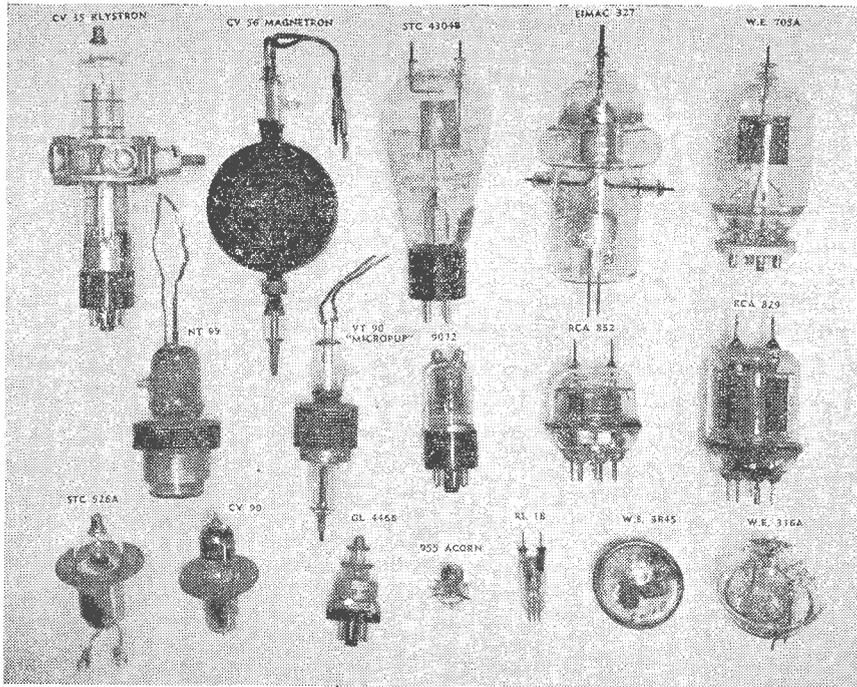
Fig. 2.—A representative group of valves used in U.H.F. equipment.
