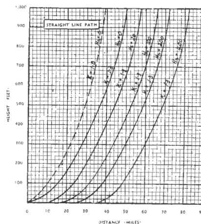
Fig. 3.—These curves show the effect of antenna heights and atmospheric refractions upon the line-of-sight transmission.
