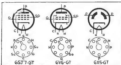
This diagram shows the connections for the three valves. The socket is viewed from the underneath.
