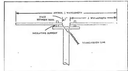
Fig. 1.—A half-wave dipole antenna used for F-M reception.
