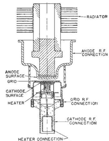
Fig. 3.—A sectional drawing of the 2C39.
