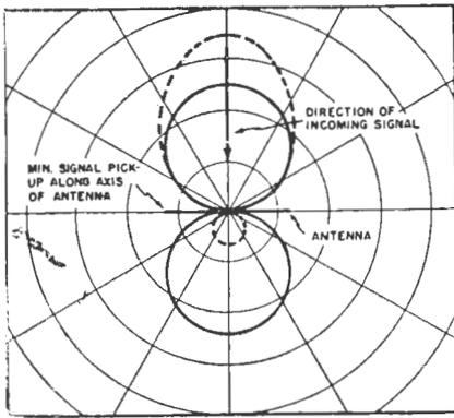
Fig. 4.—Horizontal radiation pattern of a dipole.
