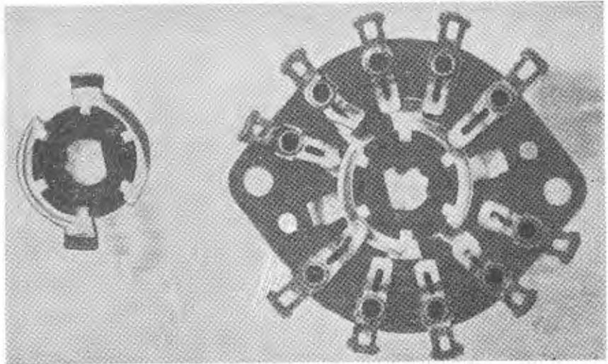
Photograph of a typical wafer switch, subjected to mechanical life test after cleaning with carbon tetrachloride.
