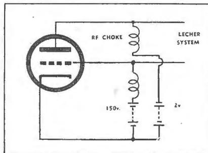
Fig. 11.—The Barkhausen and Kurz positive grid oscillator circuit.
