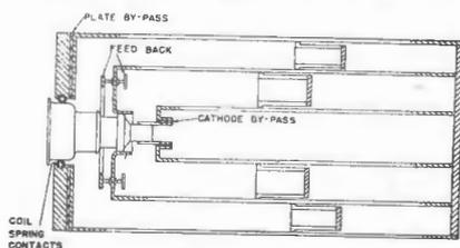
Fig. 8.—A cross-section layout of the 2C39 co-axial line oscillator.
