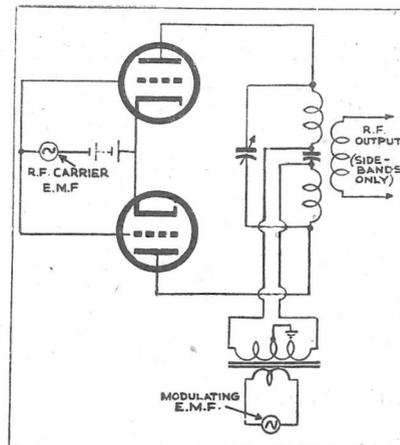
Fig. 6.—Basic arrangement of balanced modulator.
