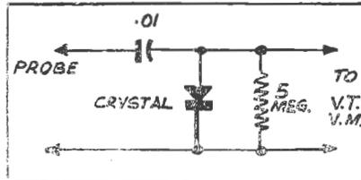
Circuit of the simple diode probe using a germanium crystal.
