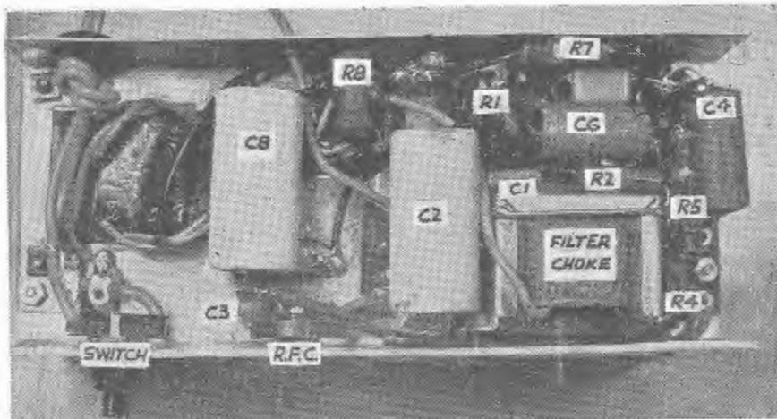
This underneath chassis shows the location of most components and should be used as a guide when wiring up. The numbered components refer to those shown in the circuit diagram.
