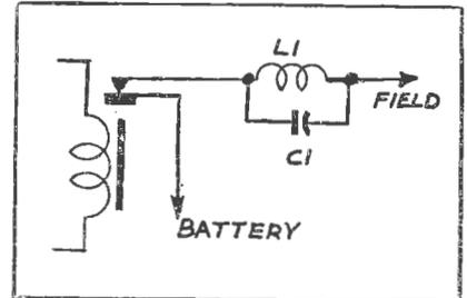
Details of the regulator filter. The coil, L1 consists of 25 turns, 22 SWG enam. wire, 3/8 inch dia., 3/4 inch long. The condenser C1, is a standard 455 kc. padder.
