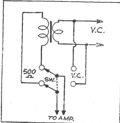
The use of a double pole-double throw switch enables the speaker connections to be changed.
