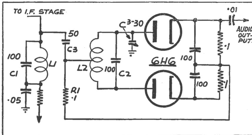
This diagram shows the changes necessary to add a discriminator section permitting narrow band F-M reception.
