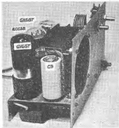
This photograph clearly shows the mounting of the second filter condenser (C9) alongside the speaker.
