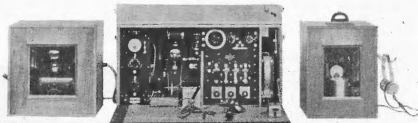
Portable Wireless Telephone-Telegraph Station, fitted with Marconi Wireless Call Bell. Centre: Instrument Box, Main Transmitter and Receiver. Right: Wireless "Call" Receiver. Left: Wireless Call Transmitter.
