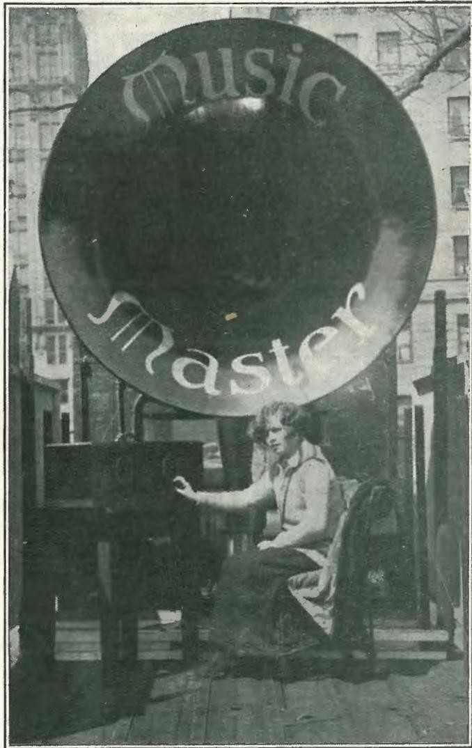
What is claimed to be the world's greatest loud-speaker was recently used at the New York Radio Show. It stands 11ft. 6ins. from the base and the opening of the horn is 6ft. in diameter. The wooden bell is made of 4,000 pieces of mahogany, the base and goose-neck being of aluminium. It weighs 1,000 lbs. and took six weeks to build. It is operated by a super-heterodyne receiving set and can be heard a considerable distance away.
