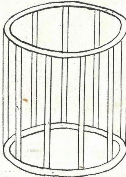
of two hard rubber rings with eight hard rubber strips connected to them, as shown in the drawings. Bare wire may be used, and in fact is preferable to insulated wire, as there is distributed capacity between turns. Number 18 or 20 copper wire may be used and should be annealed so as to be handled very easily.
