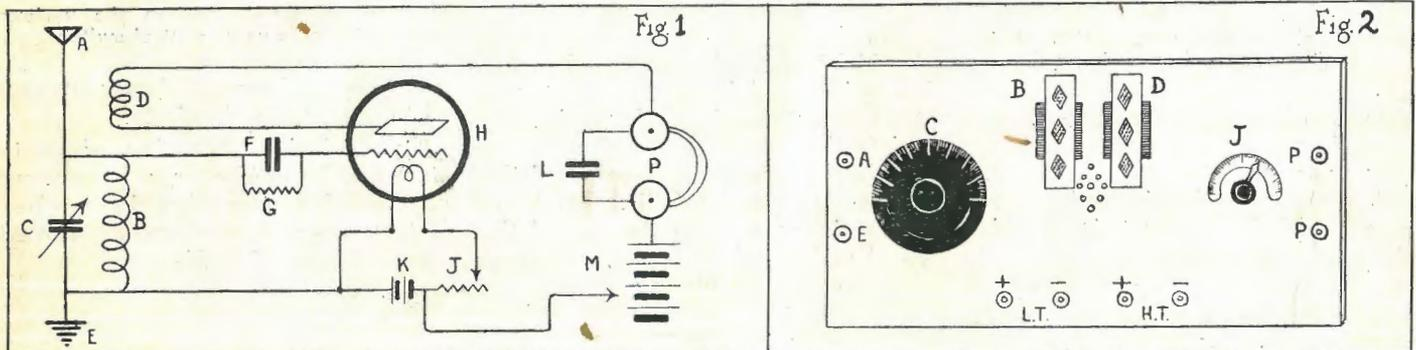
Index to Figures 1, 2 and 3. A: Aerial. B: Grid Coil. C: Twenty-three Plate Variable Condenser. D: Reaction Coil. E: Earth. F: Grid Condenser. G: Grid Leak. H: Valve. I: Valve Holder. J: Filament Rheostat. K: Low Tension (A) Battery. L: Fixed Condenser across 'phones. M: High Tension (B) Battery. P: Telephone Receivers.
