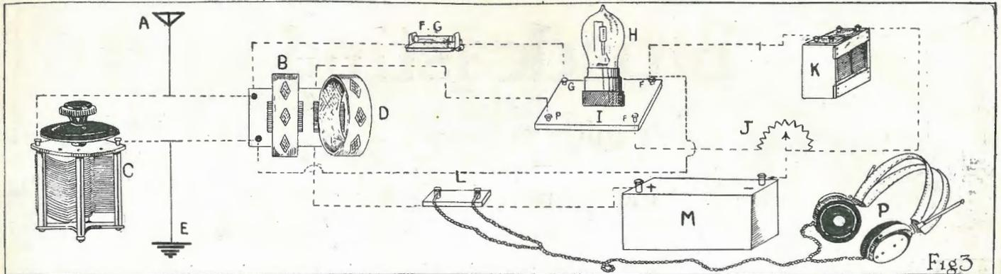
Figure 3: Illustrates the various component parts of receiver and how same are connected. The dotted lines indicate connecting wires.
