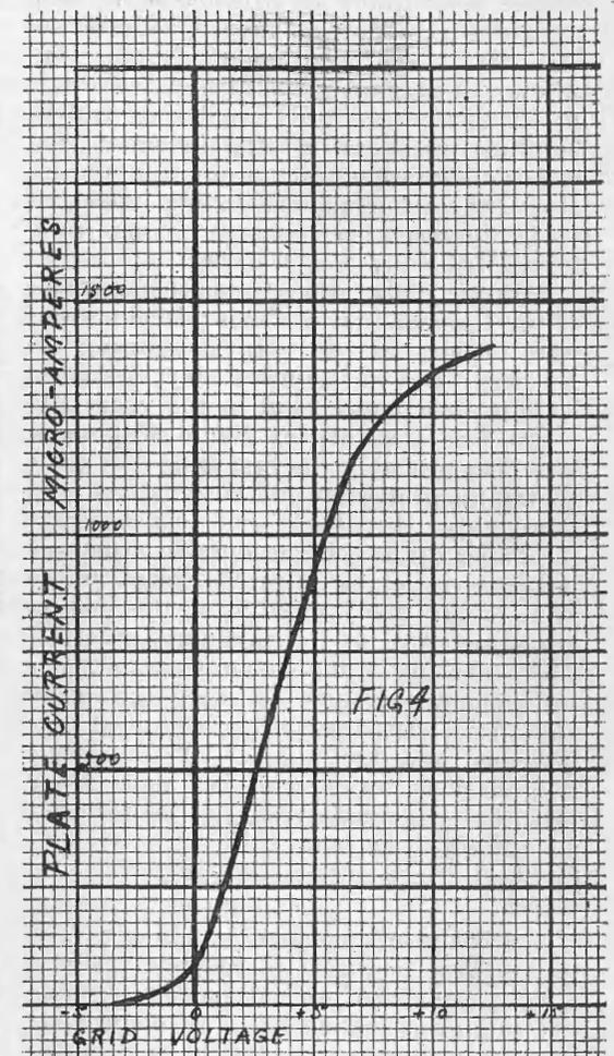
Characteristic Grid Voltage, Plate Current Curve of a Valve Showing Bend With Zero Potential on the Grid.
