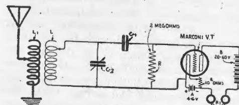
Diagram Illustrating Application of Grid Condenser "C<sub>1</sub>" and Grid Leak "R" to Three Electrode Valve to Obtain Maximum Rectification.
