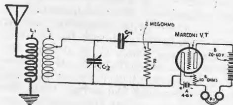
Diagram Illustrating Application of Grid Condenser "C" and Grid Leak "R" to Three Electrode Valve to Obtain Maximum Rectification.
