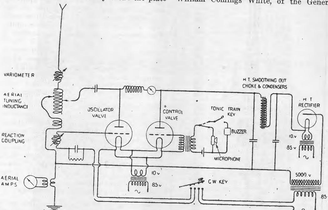
Diagram of Wireless Telephone Apparatus showing William Comings White's Principle of Modulating Carrier Wave by Control Valve.
