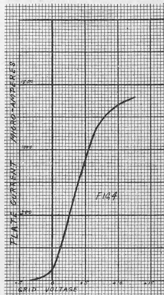
Characteristic Grid Voltage, Plate Current Curve of a Valve Showing Bend With Zero Potential on the Grid.
