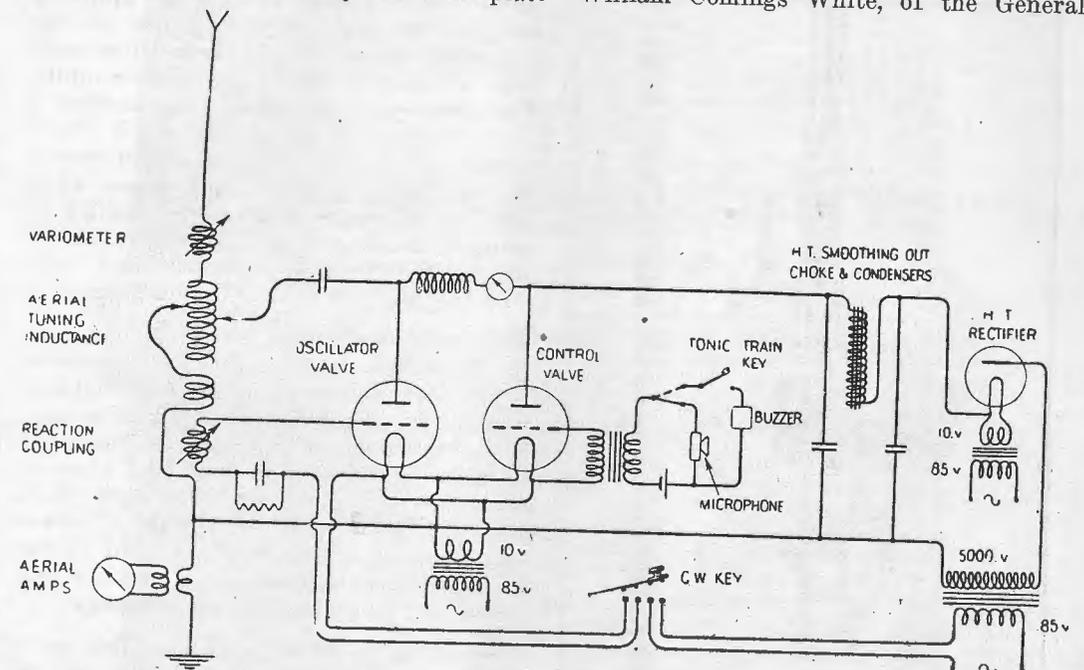
Diagram of Wireless Telephone Apparatus showing William Comings White's Principle of Modulating Carrier Wave by Control Valve.
