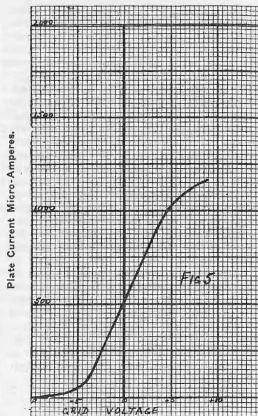
Characteristic Grid Voltage, Plate Current Curve of a Valve Requiring a Negative Grid Potential so as to Operate the Valve as a Detector at a Lower Point on the Curve.
