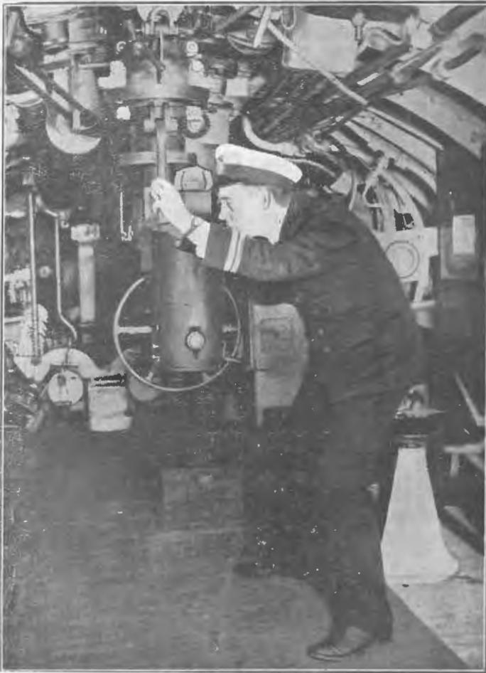
ASCERTAINING THE VESSEL'S POSITION AT THE PERISCOPE OF A SUBMARINE.
