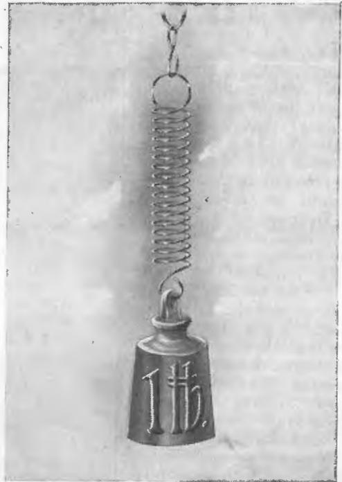
Coiled Spring and Weight, for Producing Mechanical Oscillations.
