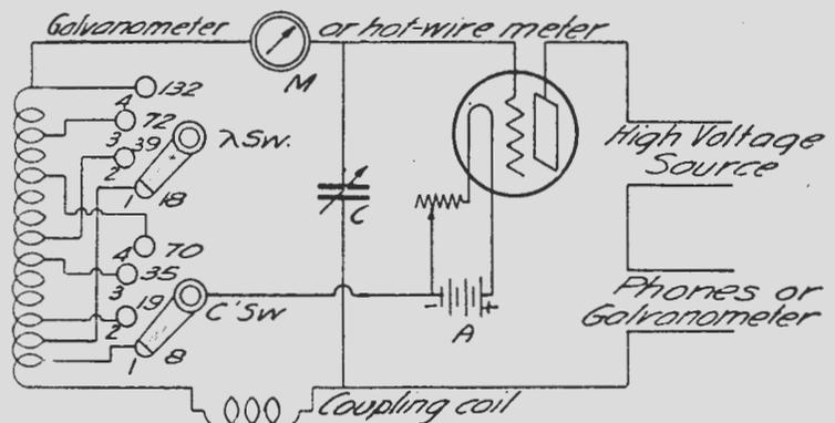
Fig 1 Wavemeter Wiring Diagram
