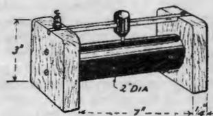
Fig. 2.—The finished potentiometer.
