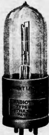
**W.D. 12.** The W.D. 12 operates with 1.5 volts, on the filament with current consumption of only .25 amps. The special oxide coated filament gives a high electron emission at low filament temperature. A single 1.5 volt dry cell may thus be used for filament heating, and these valves are noted for their economical operation, uniform performance, and long life.
