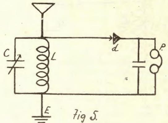
sumed that this circuit arrangement will give any greater selectivity, for this cannot be obtained with single coil tuners, owing to the fact as before mentioned, of the circuit being so tightly coupled. This is the reason why so many have found that one of
