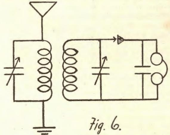
about a 75 turn for 2FC. In this circuit there are no losses due to end turns owing to the large coil not being in electrical connection to the small one when not in use. The variable condenser tunes the coils irrespective of which are in use, thereby providing the finest tuning. It must not be as-
