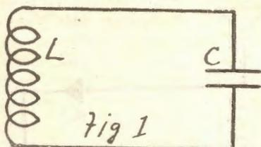
Both these components, L and C, may exist in different forms and degrees; for instance we may have an arrangement such as Fig. 2, where A is a large aerial which possesses inductance and C the condenser. In this it will be seen that the total capacity is very much greater than the inductance, for the aerial also possesses capacity. It is therefore evident that the arrangement is of little use because it is very much unbalanced or both components are a long way out of proportion.
