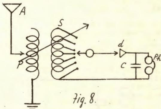
as far as operation is concerned. The first thing noticed is that it contains one of the faults of a single coil tuner, that is, end turn losses, and also as it has to be put into certain positions, it has to be wound with fairly fine wire, hereby increasing the damping or making it more broadly tuned.
