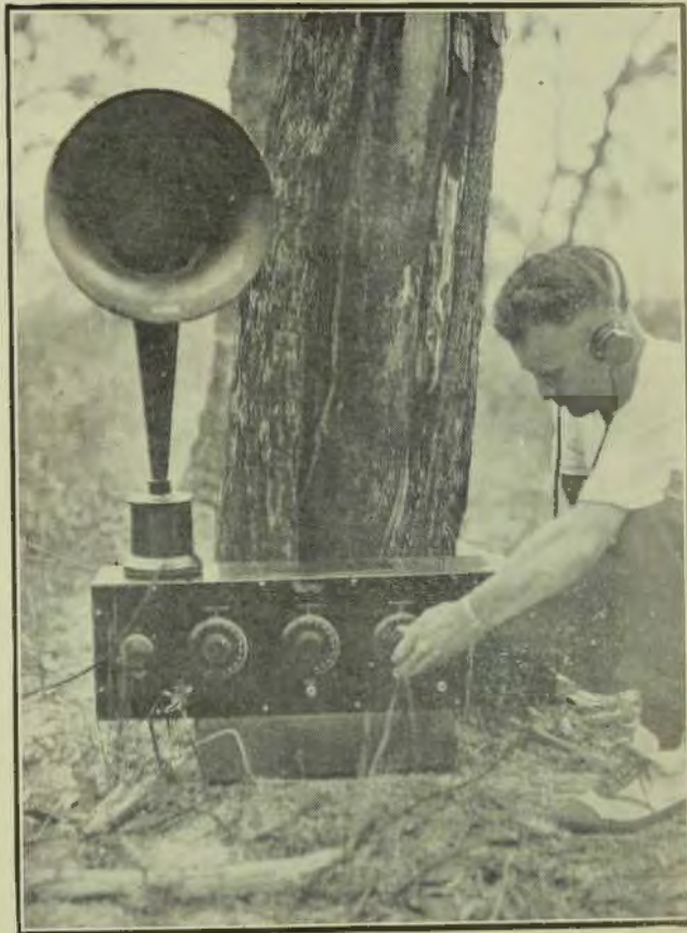
Photographs taken 72 miles north of Sydney on Newcastle Road. Using 20 ft. insulated wire for aerial and 10 ft bare wire for ground. Broadcasters could be heard on loud-speaker 50 yards away. 2JM and 2ZG came in very loud and clear.
