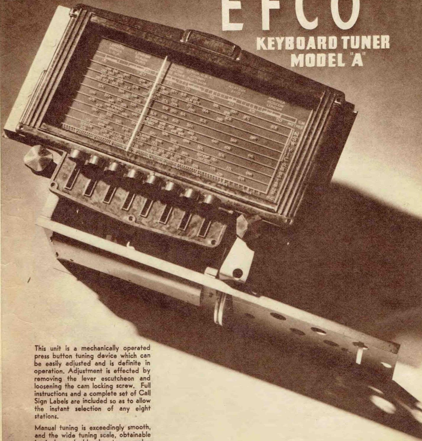
This unit is a mechanically operated press button tuning device which can be easily adjusted and is definite in operation. Adjustment is effected by removing the lever escutcheon and loosening the cam locking screw. Full instructions and a complete set of Call Sign Labels are included so as to allow the instant selection of any eight stations.
