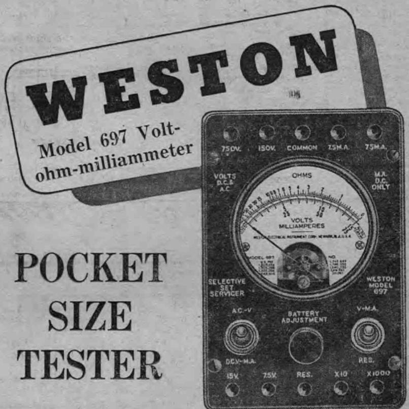
This unit is proving very popular as a pocket size tester, because it is an A.C.-D.C. instrument, with 10 convenient ranges as under:—
