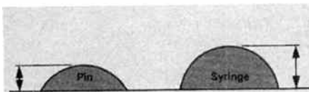
Fig. 10. Adhesive dot height determined by type of adhesive and application method.
