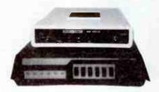
A brace of modems! On top is the Sendata, which comes with quite a sophisticated software package and costs \$399. (A 'Mini Cooper S' machine). Beneath is the four-speed auto-dial DPX224 Hayes-compatible modem. It costs \$1872, tax paid. (A 'BMW').
