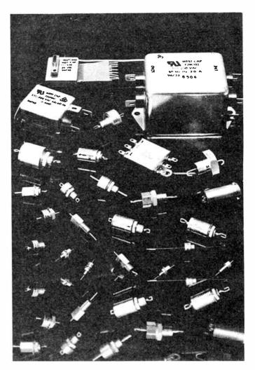
0.015 and at 10 kHz around 0.025. Their temperature coefficient is normally around + 600 ppm per degree. These capacitors have a good pulse handling capability within their voltage ratings. MKL capacitors can be considered an "exotic" type as they are expensive and normally used in professional and military equipment. Quality assessed versions are available for military and aerospace applications — but they also make excellent coupling capacitors in very high quality audio equipment.
