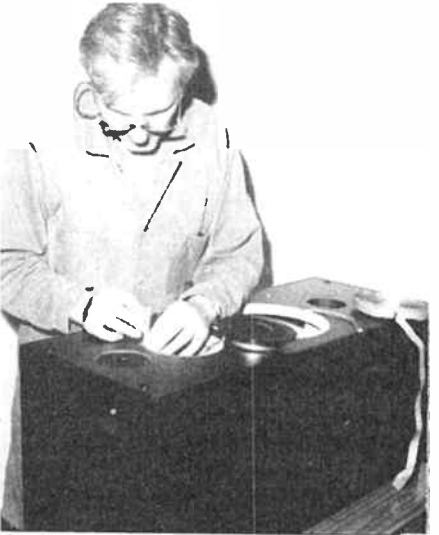
The drive units are sealed and set flush with the front panel by making gaskets from 12 mm wide Body Moulding Tape. Take care when mounting the tweeter and mid-range.
