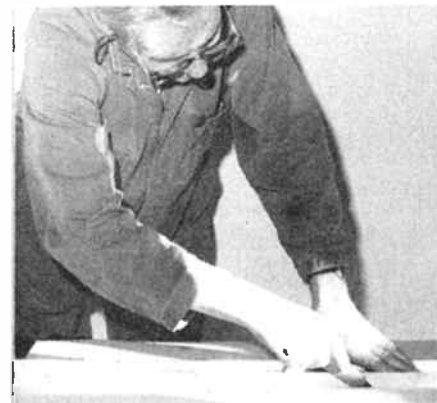
Cut the high density foam to size before lining the cabinet with it. Don't forget the strategic holes in the rear pieces to allow for bracing and wires to the rear spring terminal connector.
