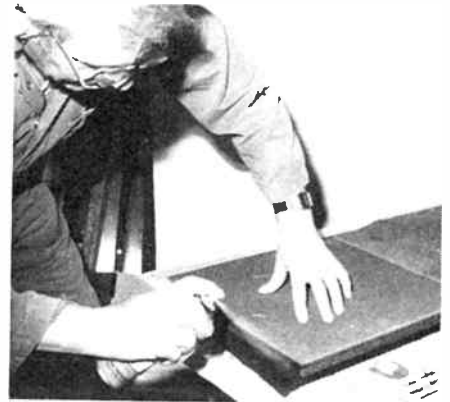
Place the frame on top of the grille cloth and spray part of the frame and the part of the grille cloth that sticks out past the frame with spray adhesive.
