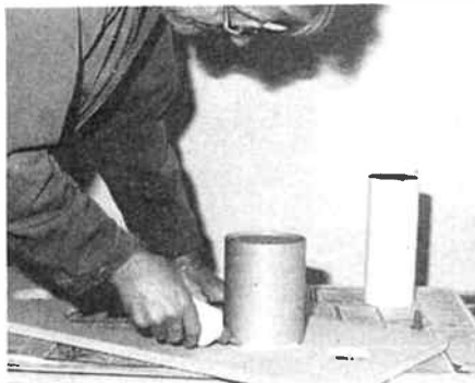
Apply PVA glue around the outside of the mid-range chamber, right on the inside surface of the front panel, to effectively seal the joint.
