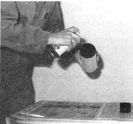
Spray the bass reflex port tubes black inside.
