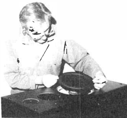
The woofer is fitted last of all.
