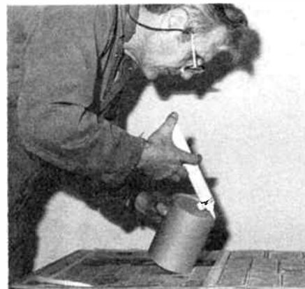
Apply liquid nails to the end of the mid-range chamber.
