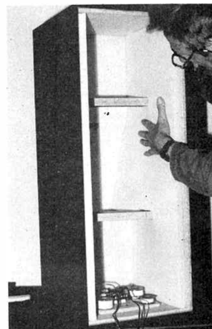
The foam is fitted in the cabinet, held in place with glue.
