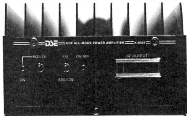
View of the front panel (above) and internal view of the completed project (below). Input socket is on the left, output on the right. Note the RF output meter at top right.
