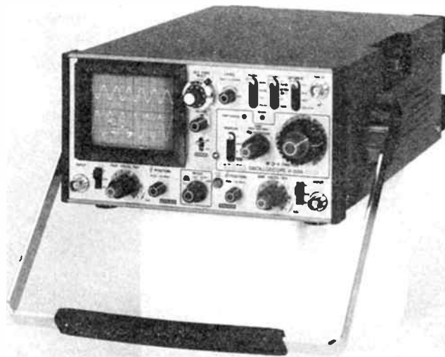
This portable Hitachi CRO, the V-509, is a 50 MHz dual-trace, twin-timebase instrument featuring vertical sensitivity of 5 mV/div., sweep speeds from 100 us/div. to 200 ms/div. and video (TV) triggering facilities.
