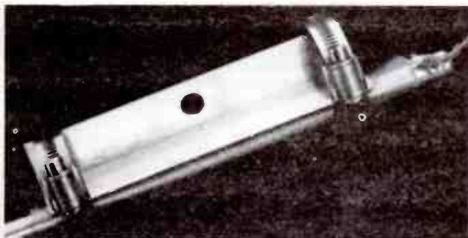
The mounting brackets are assembled to each dipole half as shown here.
