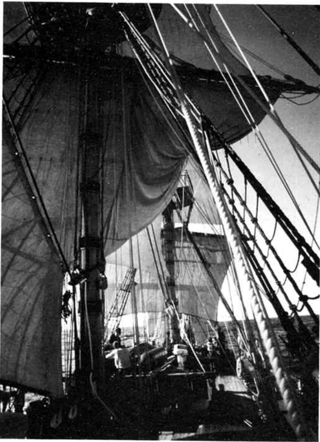
At sea, with the weather clew and mainsail raised to get better airflow over the foresail. The ceramic aerial insulators for the HF SSB transceiver can be seen at the base of the mast in the foreground.
