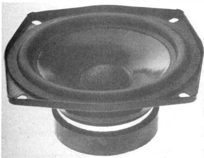
The two Vifa drivers used. At left is the 125 mm C13WG bass/mid-range unit which features a long-throw voice coil and very wide frequency response. At right is the D19TD tweeter featuring a ferro-fluid cooled and damped voice coil.
