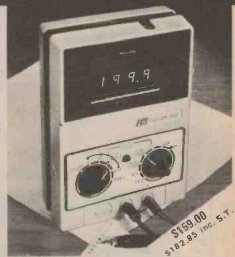
The B&K-PRECISION Model 2810 has a combination of features uncommon in a portable digital VOM. Basic DC accuracy is 0.5% with a 3½ digit display. Auto zeroing on all but the 10Ω range minimizes set-up time while the 100% overranging capability reduces the need for frequent range changes.
