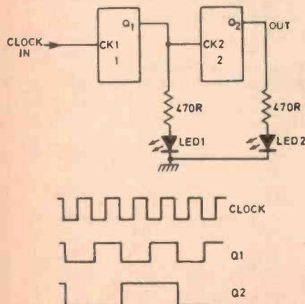
Fig. 1. Cascading 7476 flip-flops.
