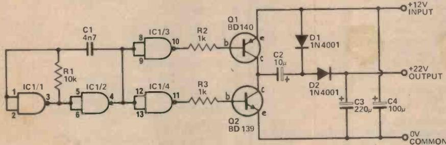
Fig. 4. The circuit diagram of the +22V version.
