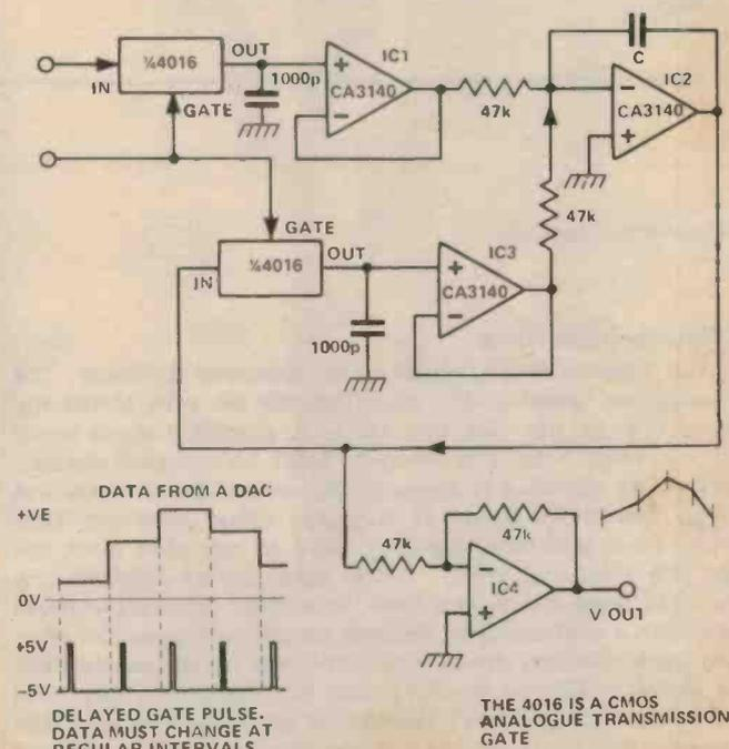
integrator's capacitor C should be chosen to suit the clock speed of the dac. An inverter, IC4 has been included to correct the inversion caused by the integrator.
