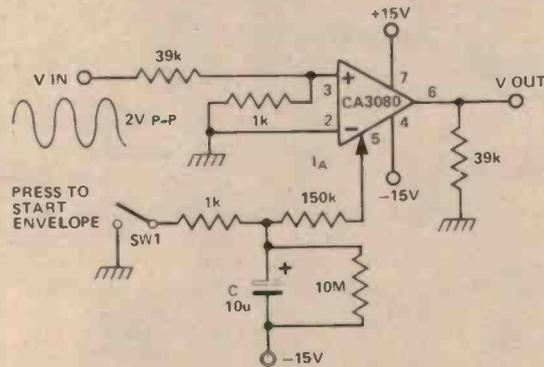
an exponential envelope is generated. Breakthrough after the decay is very good, better than  $-80$  dB.
