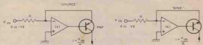
so the base current loss is not a fixed percentage. However, a precise voltage to current converter can be made using an op-amp with a FET input so that the bias current is low. Also, an input balance can be used to zero out the input offset voltage, and if a FET is used to replace the bipolar transistor, then the base current problem can be removed.
