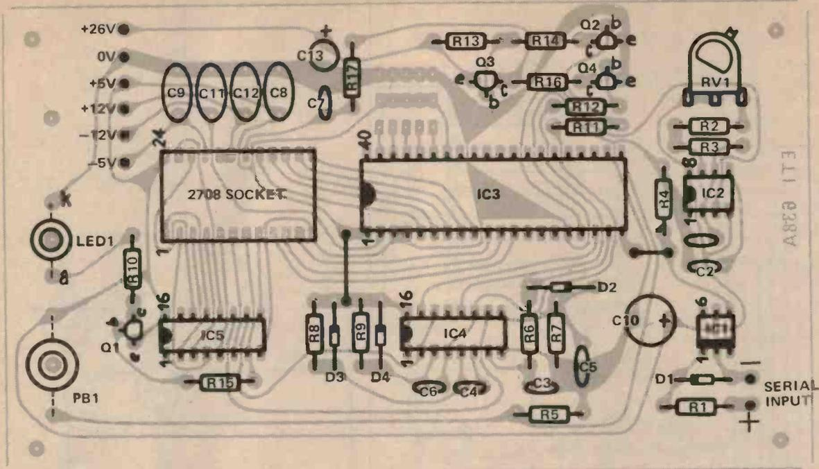
Fig. 1 The component overlay of the main board.
