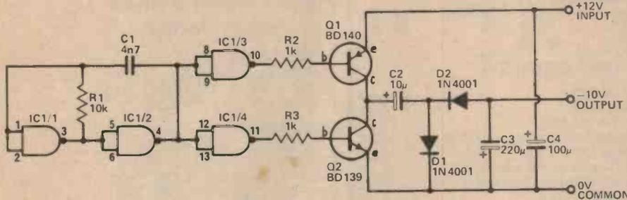
Fig. 3. The circuit diagram of the -10V version.
