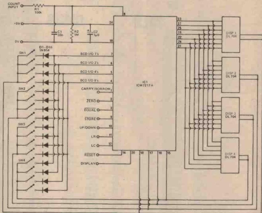
Fig. 3. The circuit diagram for the counter board.
