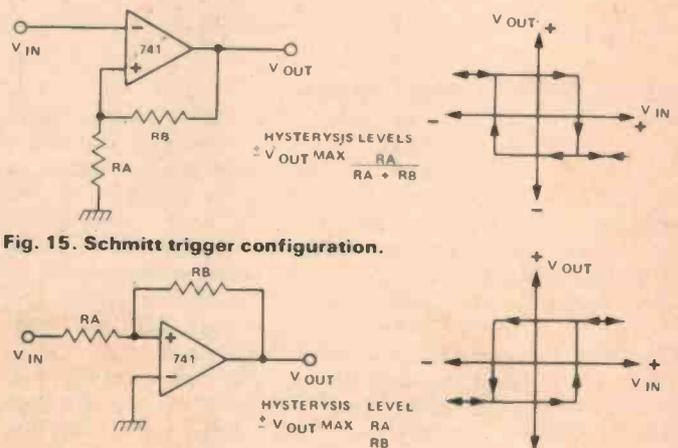
Fig. 15. Schmitt trigger configuration.
