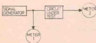
The ratio of the reading of meter 1 to the reading of meter 2 is called the response of the circuit. If the generator frequency is varied, the output reading on meter 2 varies because the circuit behaves differently when fed with different frequencies. If this ratio of input to output voltage is plotted against frequency, the resulting graph is called a Frequency Response Curve.
