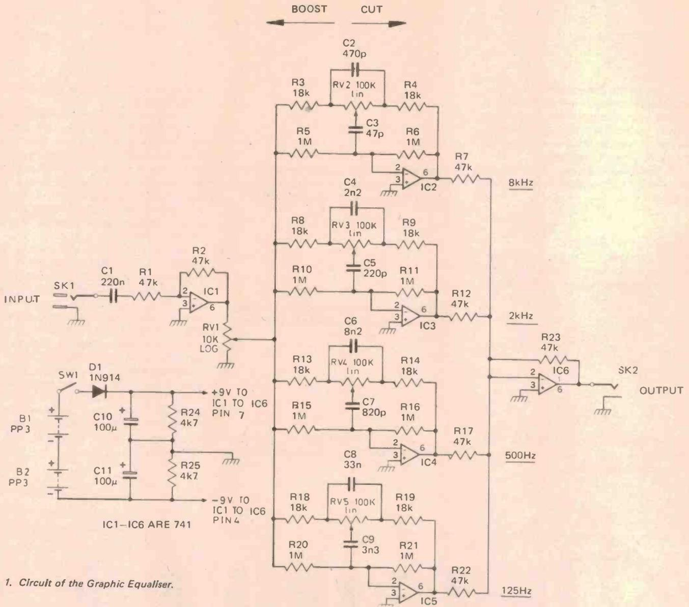
Fig. 1. Circuit of the Graphic Equaliser.
