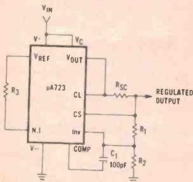
Note:  $R_3 = \frac{R_1 R_2}{R_1 + R_2}$  for minimum temperature drift.
