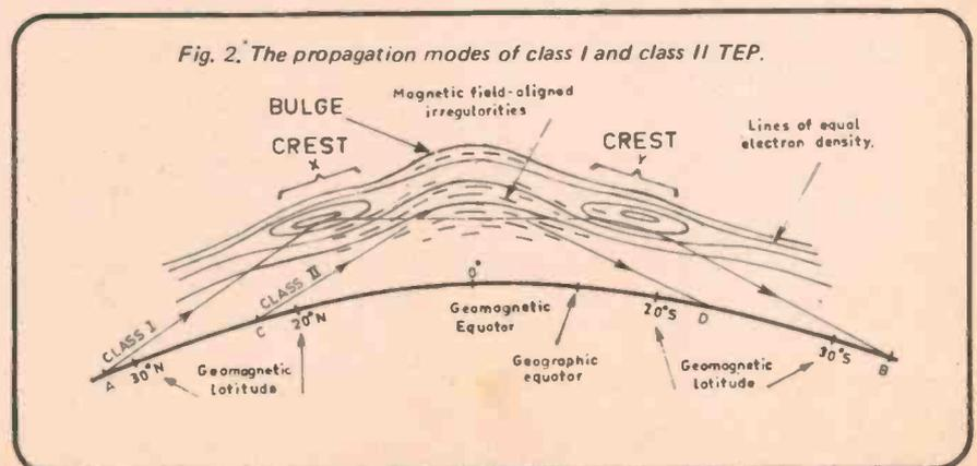
Fig. 2. The propagation modes of class I and class II TEP.
