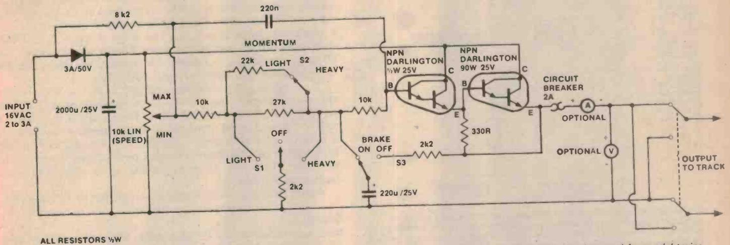
Fig. 1. An electronic speed control for model trains.
