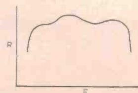
This will be further modified by the response of the room where the hi-fi is — even your curtains have a response curve! By the time the signal finally reaches your ears the overall response will be fairly well mangled.
