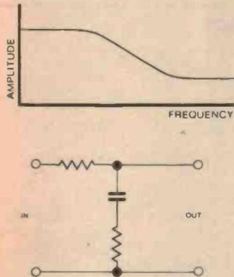
Fig. 4a. Low boost circuit and response curve.
