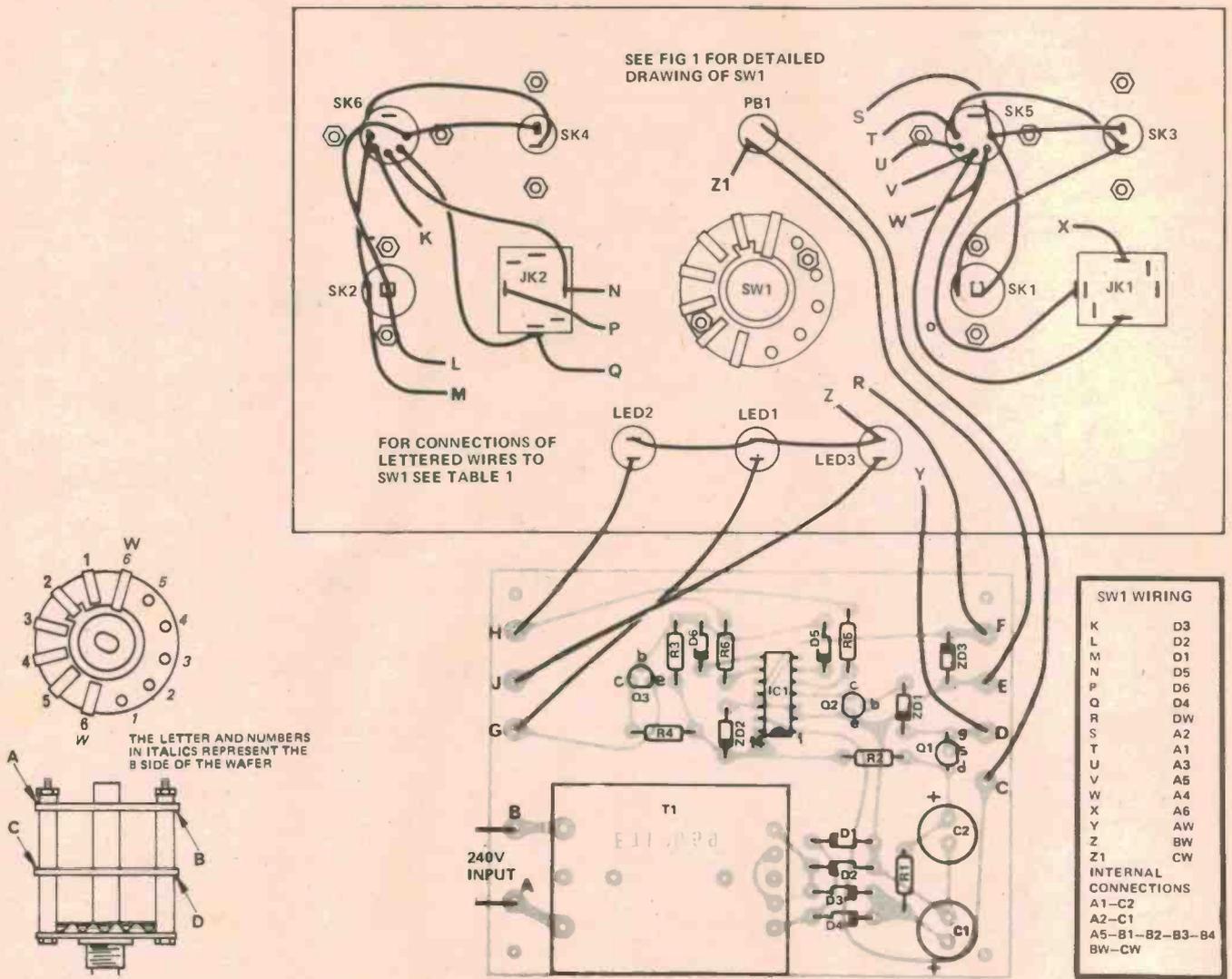
Fig. 3. Component overlay and front panel connections.
