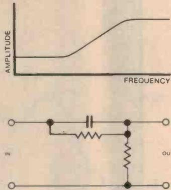
Fig. 4b. High boost circuit and response curve.
