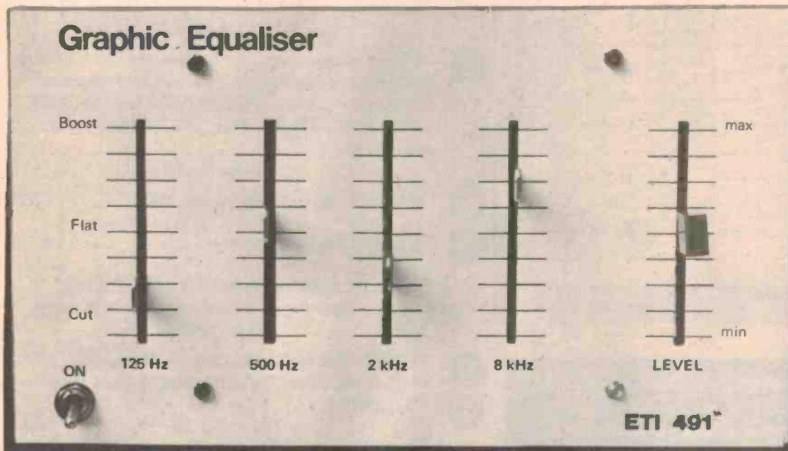
A GRAPHIC WHAT, you ask? A graphic equaliser is a complex form of tone control. It can be used to smooth out the frequency response of a hi-fi, or as a guitar effects unit. In fact, it will prove useful in any audio application.
