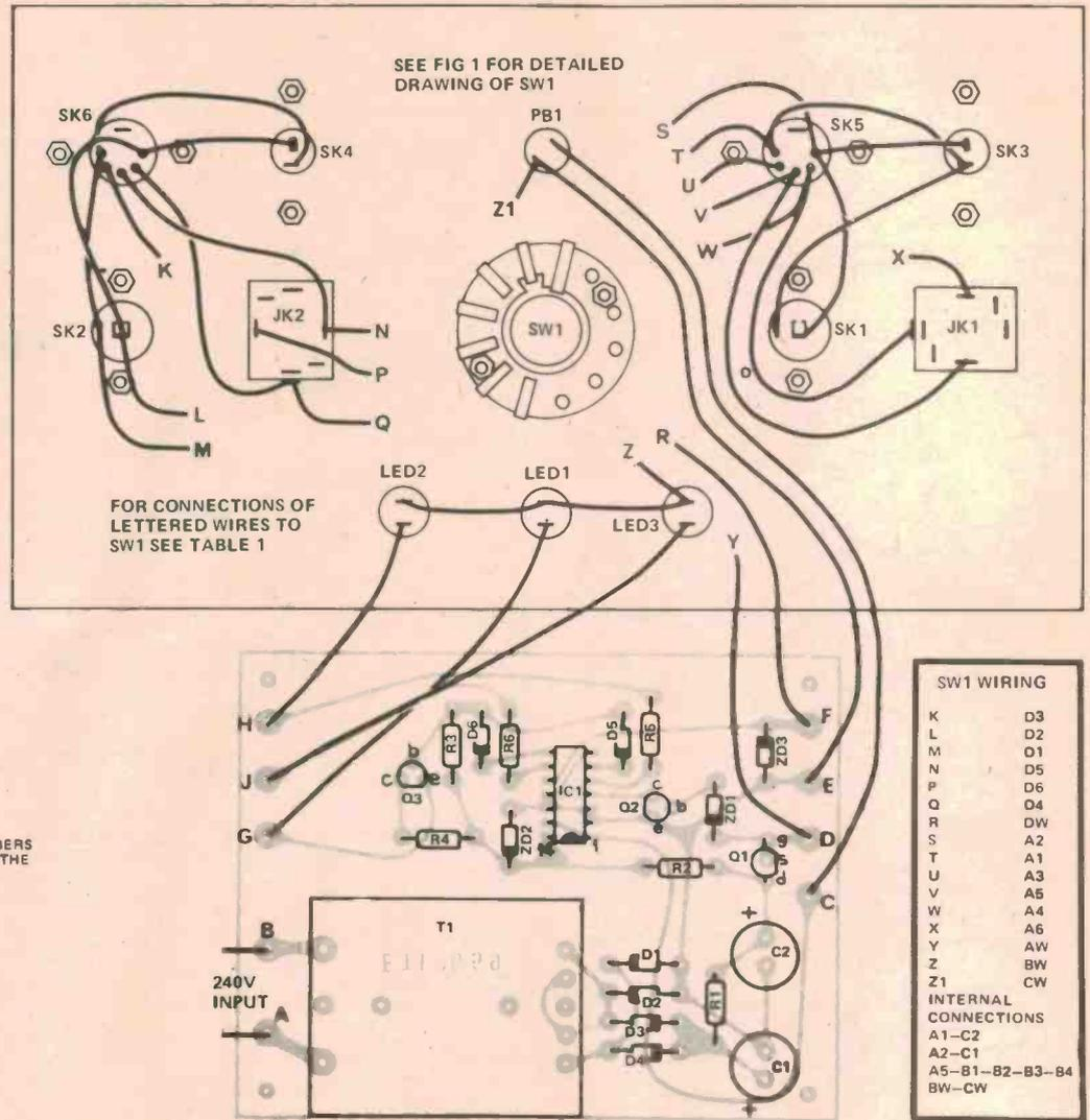
Fig. 3. Component overlay and front panel connections.
