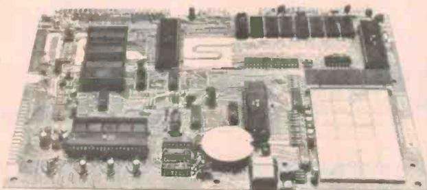
A sure starter in performance. In quality. In availability. OEMs, educators, engineers, hobbyists, students, industrial users: Our Versatile Interface Module, SYM-1, is a fully assembled, true tested and warranted microcomputer board that's a single-board computer, complete with keyboard and display. All you do is provide a +5V power supply and SYM-1 gives you the rest.
