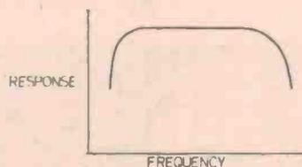
The central section of the curve is fairly 'flat' but when it comes to the very high or very low frequencies it rolls off as the circuit under test finds it difficult to maintain its output at these frequencies, reducing the reading on meter 2.
