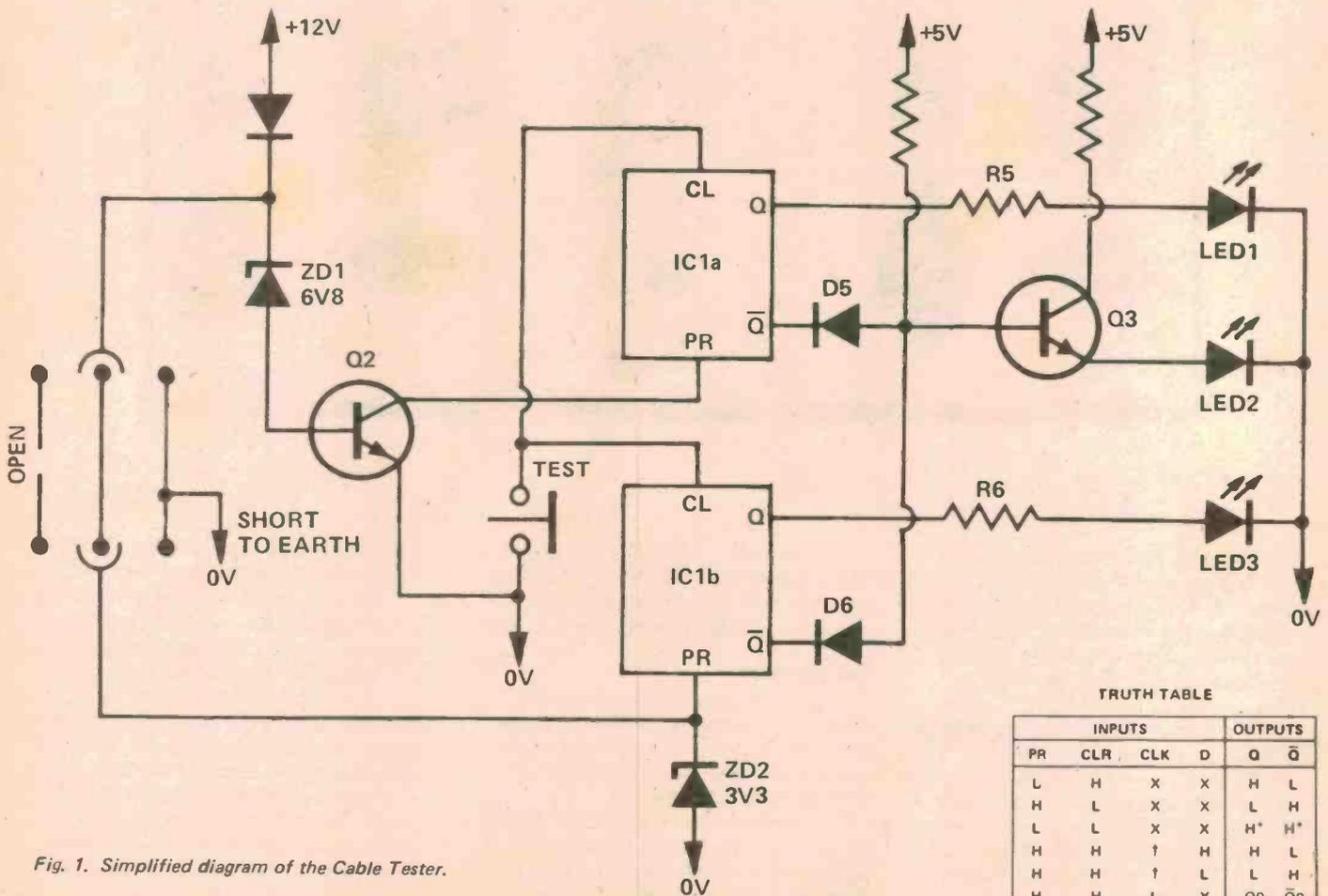
Fig. 1. Simplified diagram of the Cable Tester.
