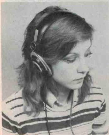
THE HV-3000R HEADPHONES come in a glossy box with no separate technical data except for a statement that the frequency response extends from 8 Hz to 28 kHz. The description on the box and the engraving on the headphones claim that these are 'studio monitor' 'phones. The difference between ordinary and studio monitor headphones may be a little hard to define but we will try.
