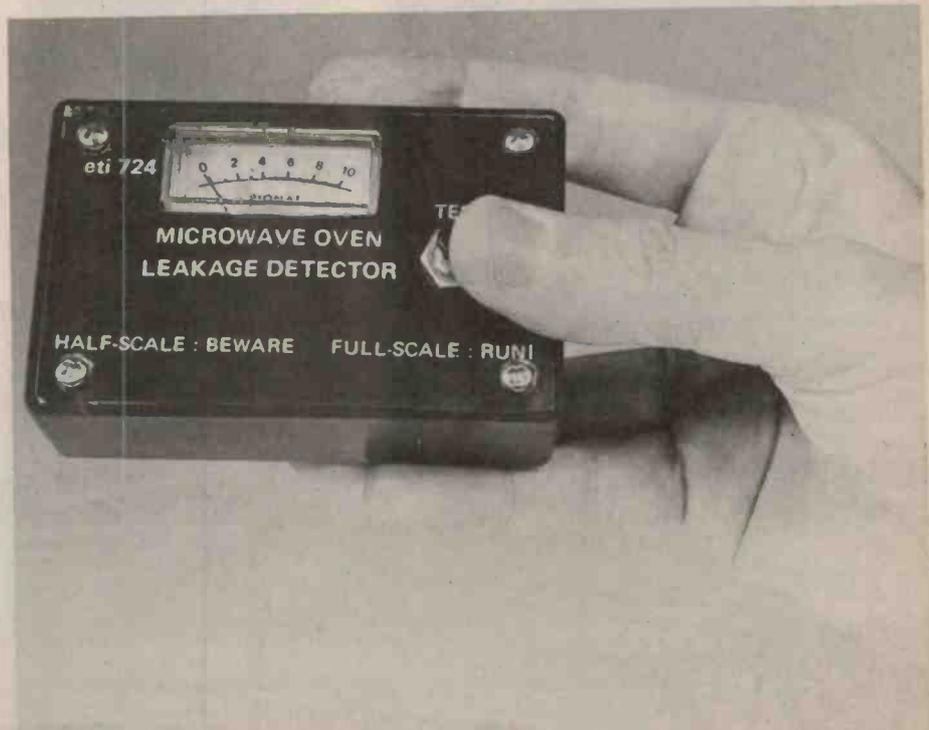
The device is housed in a 'zippy' box, everything being attached to the front panel, held in place by the four screws. Our prototypes were calibrated through the kind assistance of the Electrical Engineering Department of Sydney University.
