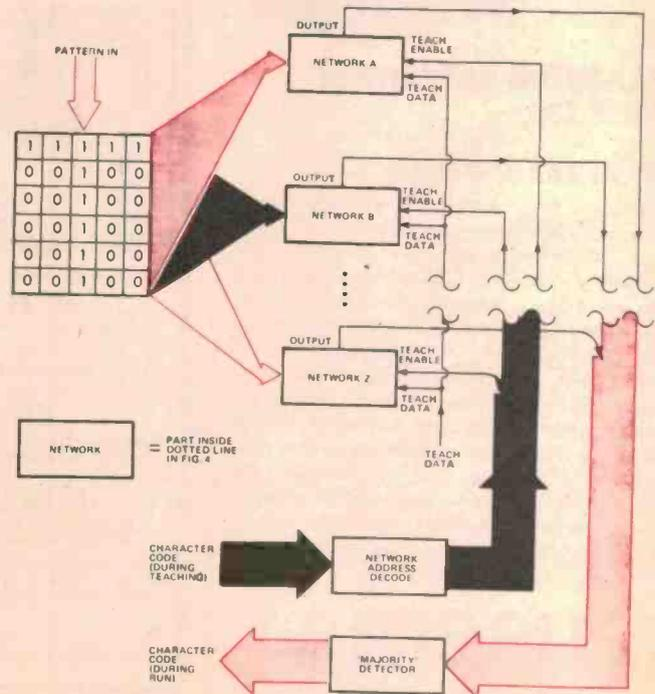
Figure 5: Several networks connected to recognize a character.
