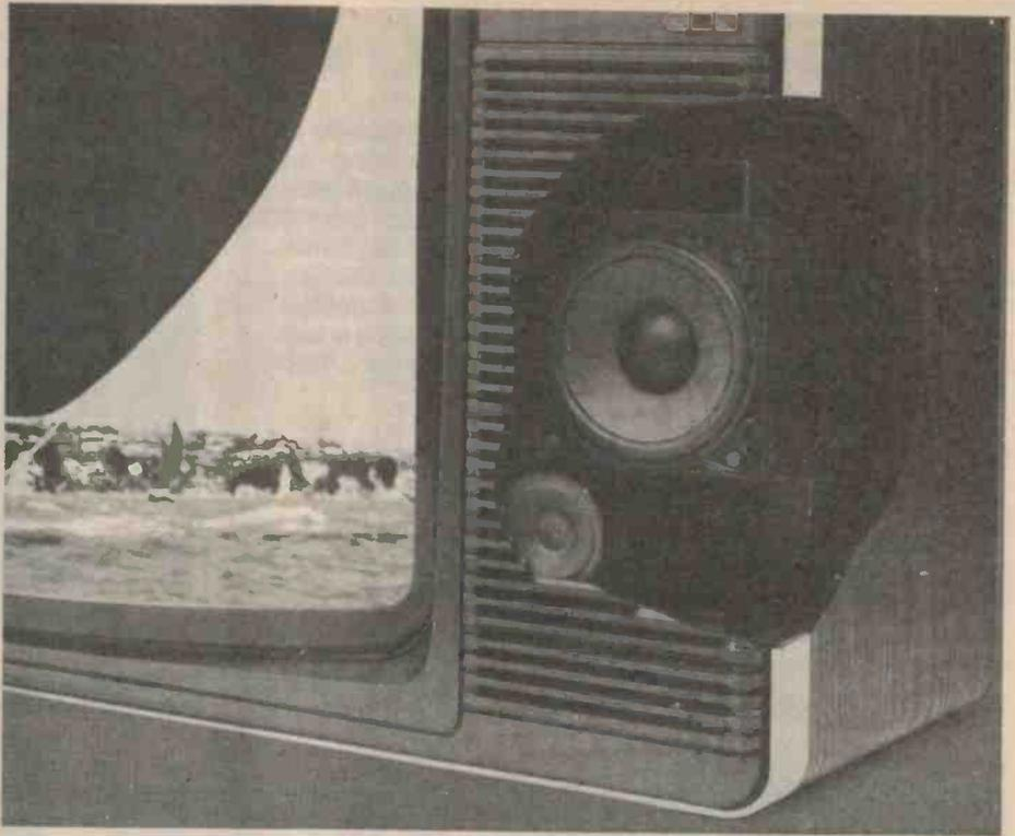
While stereo TV sound is not yet a reality (except for simulcasts), Philips have realised that the fidelity of TV sound is just as important as the fidelity of the picture. Their 'hi-fi sound' receiver, released just before the show, features a two-way speaker system plus bass and treble controls. We wonder who'll be next?
