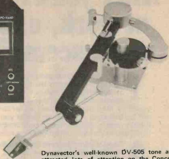
Dynavector's well-known DV-505 tone arm attracted lots of attention on the Concept Audio stand as did their new range of DV-30 series moving-coil cartridges. A DV-30 is mounted on the arm above.
