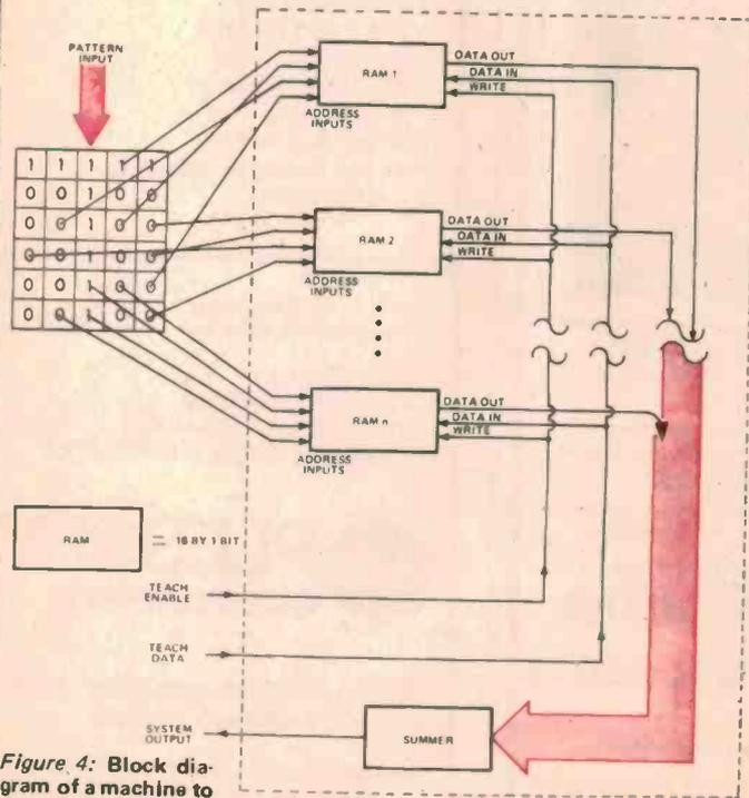
Figure 4: Block diagram of a machine to simulate a network.
