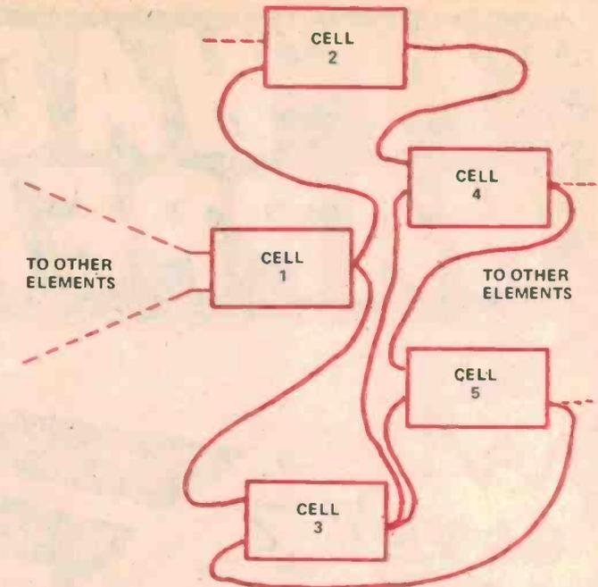
Figure 1: A network of interconnected electronic cells. Each can receive and generate binary signals.
