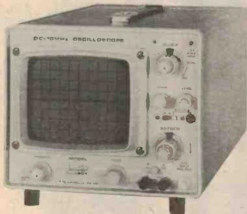
One useful feature mentioned in the literature is the isolated ground which allows the measurement of voltages referenced to a floating point.
