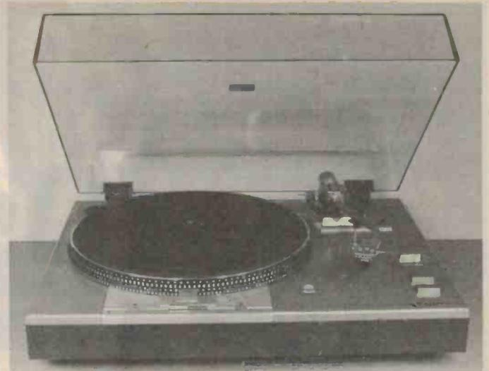
Direct-drive was clearly the trend in turntables this year. Sanyo's TP-1030 deck uses separate motors for platter and arm drive. For a full review, see August ETI.
