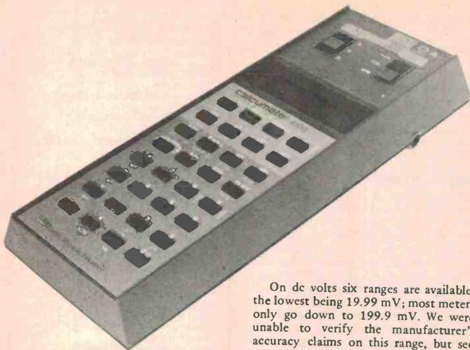
On dc volts six ranges are available, the lowest being 19.99 mV; most meters only go down to 199.9 mV. We were unable to verify the manufacturer's accuracy claims on this range, but see no reason to doubt them.
