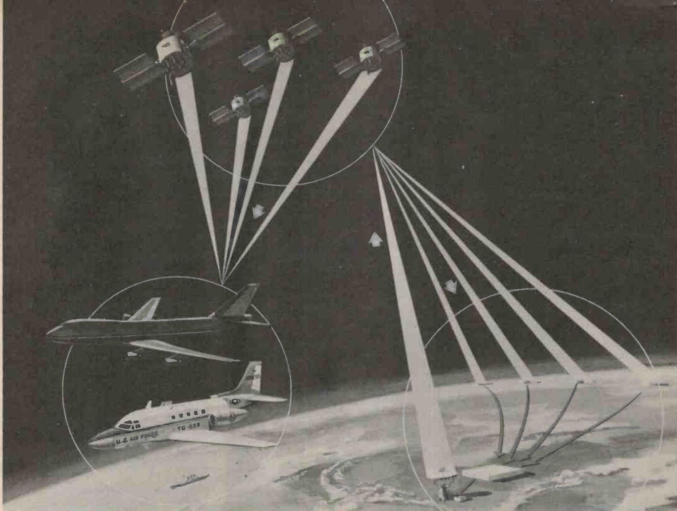
A master control station transmits command and time correction signals to the Navstar satellites. The satellites send signals to four monitor stations in Alaska, Vandenberg Air Force Base, Guam and
