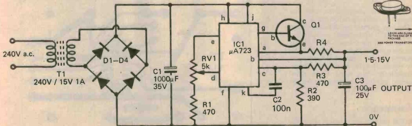
Pin numbers are not shown on the circuit diagram for the regulator IC as either DIL or CAN type packages can be used. A table for pin connections is shown on page 70.
