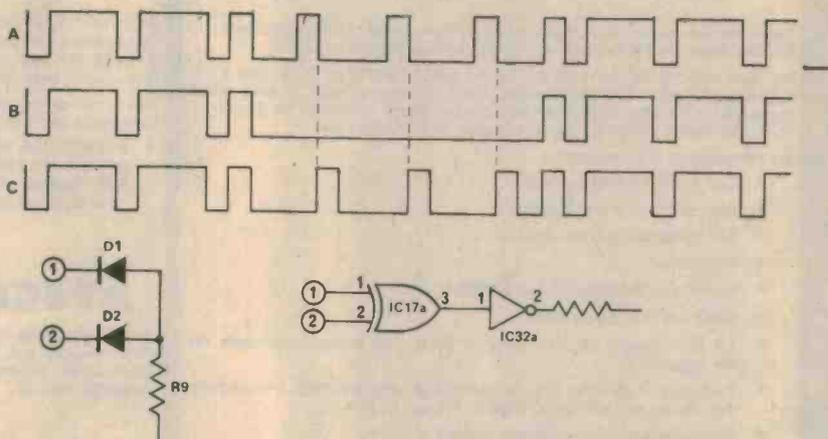
exclusive -OR gate, followed by an inverter. As both the ex-OR and the inverter are available spare in packages on the VDU board, this modification can be made without extra parts or cost!
