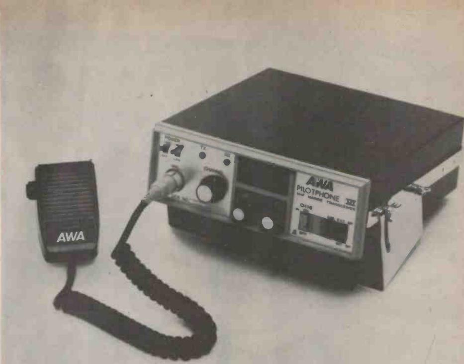
The AWA Pilotphone 6 is a 24 channel, 25 watt VHF/FM transceiver which will operate on the Seaphone channels.
