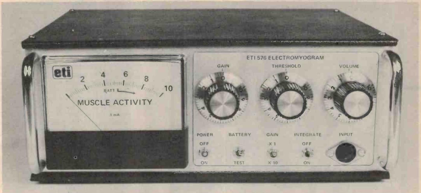
OUR PROTOTYPE was housed in a Horwood instrument case measuring 254 mm wide by 203 mm deep by 102 mm high. These are available from quite a few component suppliers but any box with similar dimensions should suffice. The advantage of this particular case is that it is supplied with steel top, bottom and side panels which provide better shielding from stray hum fields than does aluminium.
