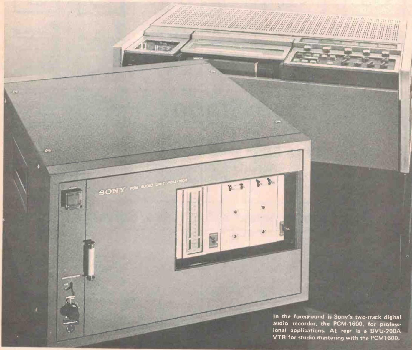
In the foreground is Sony's two-track digital audio recorder, the PCM-1600, for professional applications. At rear is a BVU-200A VTR for studio mastering with the PCM1600.
