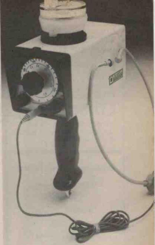
The Seafix hand-held RDF incorporates a compass to give true bearings to 1° but only covers 'long wave' for shipping weather forecasts and the beacon band.
