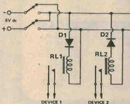
The problem of how to operate two relays independantly from just two wires always produces a lot of head scratching — and not just with beginners! This circuit, from the ETI files, shows how it's done.
