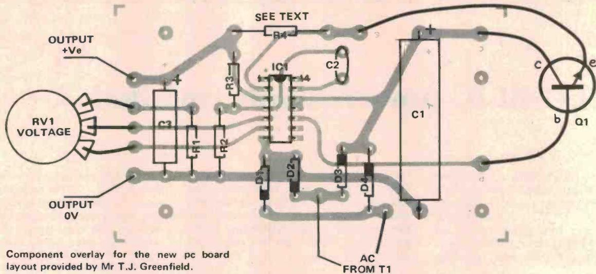
Component overlay for the new pc board layout provided by Mr T.J. Greenfield.
