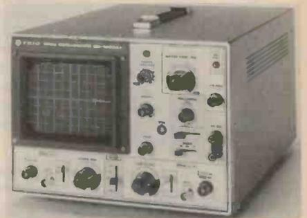
**PARAMETERS PTY LTD**, 68 Alexander St, Crows Nest, NSW 2065. (02) 439 3288. They handle Trio oscilloscopes which are among the most popular general-purpose and service types. Currently the most popular in the range is the CS-1560AII, a 15 MHz dual-trace model with easy TV sync triggering facilities. It has a sensitivity range of 10 mV/div to 20 V/div.
