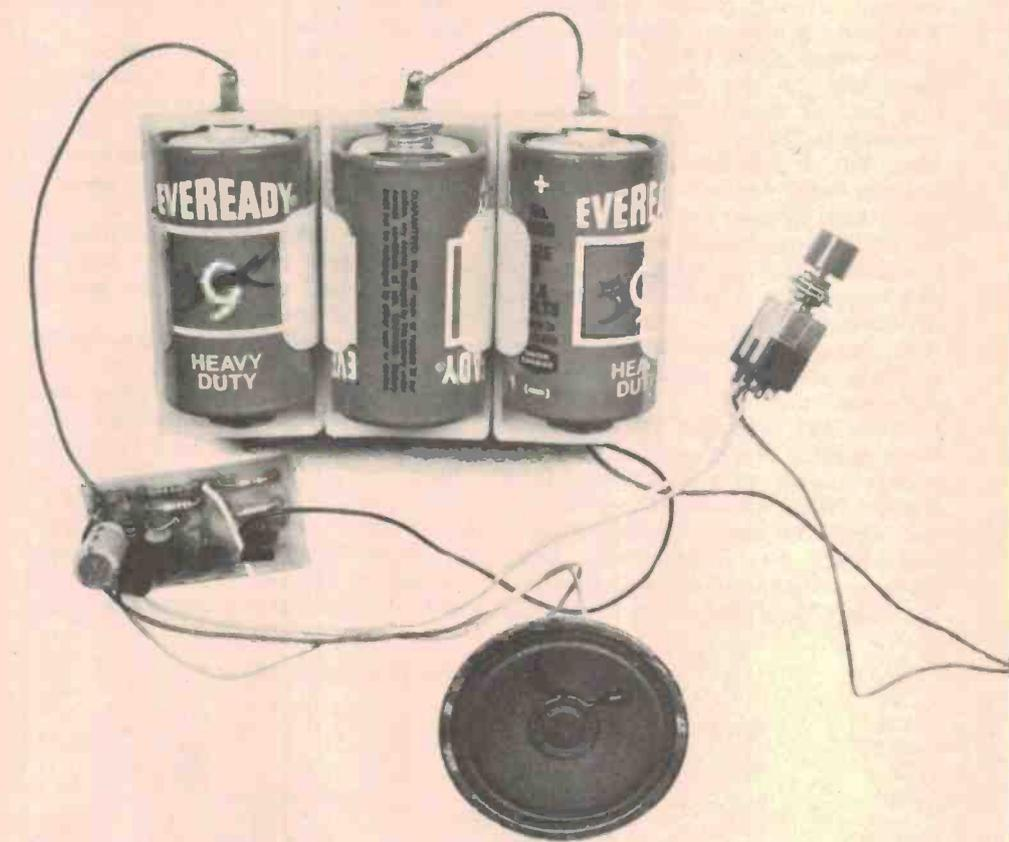
A small loudspeaker serves as both microphone and speaker in this intercom. Housing the project we have left up to you. It is quite possible to fit the components in a palm-sized box, such as one of the small 'zippy' boxes available inexpensively from a number of suppliers. The intercom may be powered from a 3 Vdc plugpack if you wish.
