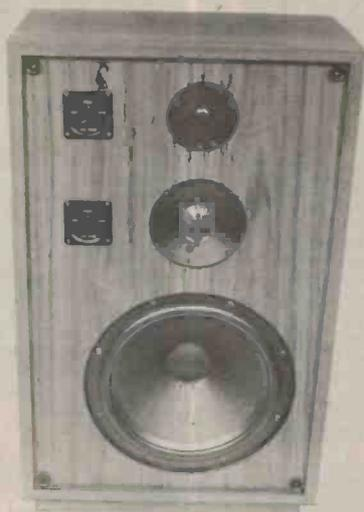
The Sirius System 1400 is a three-way pressure-box design using the AD12100/W8 woofer, AD0210/SQ8 mid-range and the AD160/T8 drivers.
