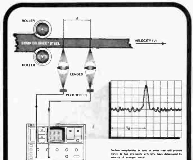
Surface irregularities in strip or sheet steel will provide signals to two photocells with time delay determined by velocity of emergent metal.
