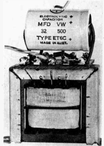
Fig. 3: Check that unused transformer tags are disconnected (maintain electrical continuity).
