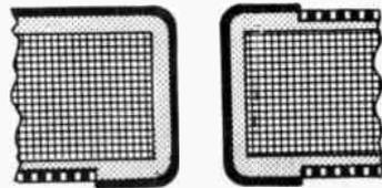
Exposed copper surfaces, tin, tin/lead or gold plated for etch stop-off.
