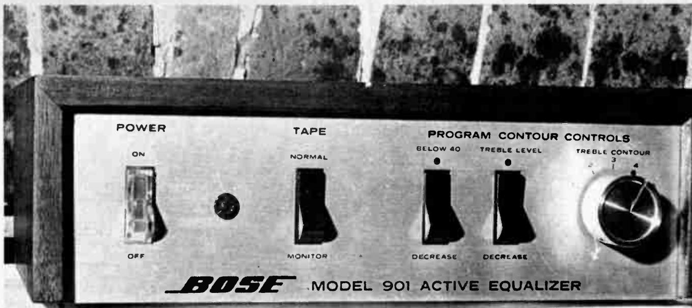
Control panel of active equaliser. The equaliser is inserted between the existing pre-amplifier and main amplifier.
