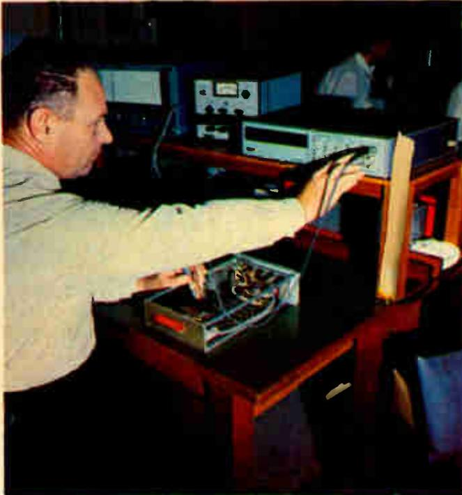
Modular construction is a feature of Natronics' Australian-made range of digital instrumentation; this frequency counter becomes 0.02% dvm by interchanging function units (test report next month).
