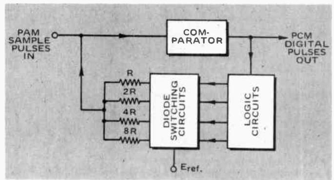
FIG. 5. Functional block diagram of a linear coder that uses the 'successive-approximation' technique to determine the digital number representing the amplitude of a PAM sample value.
