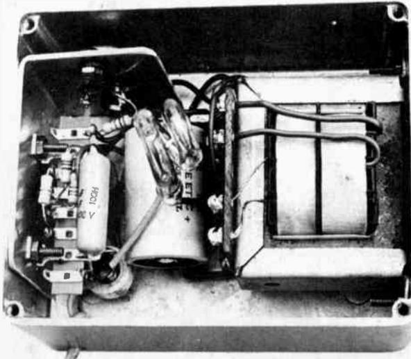
Fig. 4: All remaining components are mounted on tag strip located on transistor heat sink.
