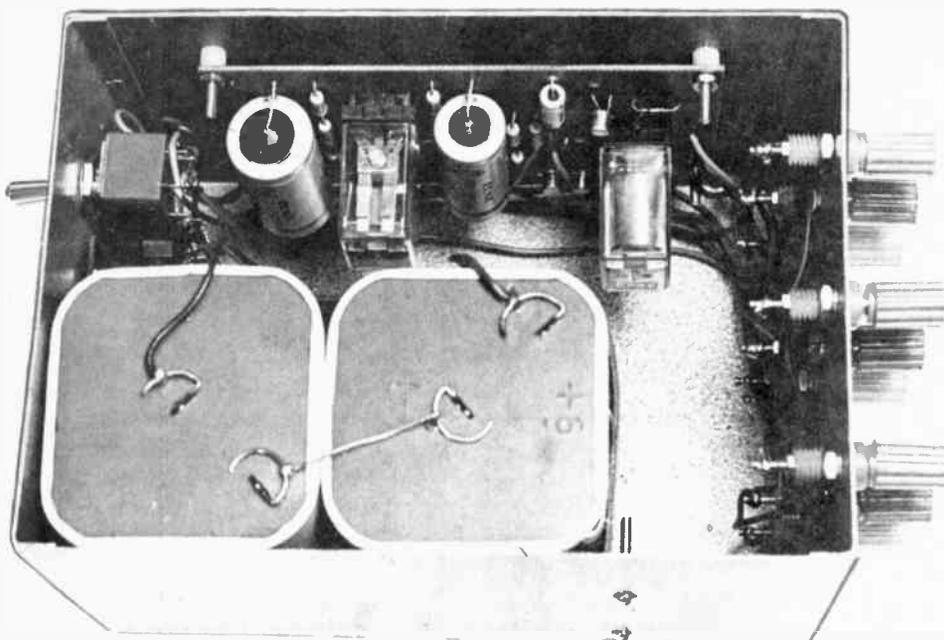
Suggested layout of components in alarm housing.
