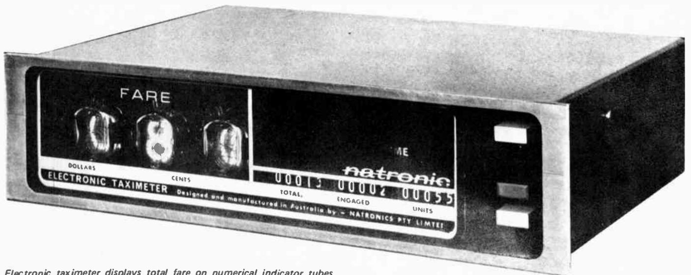
Electronic taximeter displays total fare on numerical indicator tubes.
