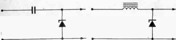
When zener diodes are used in ac applications, power loss can be reduced by using a reactive element in place of the conventional series resistor.
