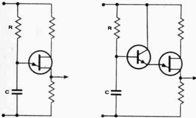
The maximum time delay obtainable from a simple unijunction timing circuit (Fig. 1) is limited by the maximum values of R and C; R cannot generally be increased beyond 3 Megohms, and space, cost and leakage limit the practical size of C.
