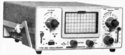
seconds after turn-on. A 6 x 10 div (1/4-inch div) internal non-illuminated graticule permits parallax-free measurements.
