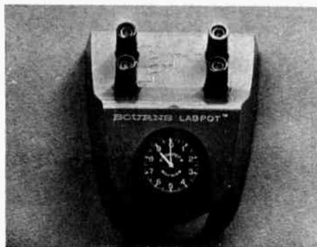
A ten-turn precision potentiometer mounted in a rugged plastic case is now available from Bourns Inc. Intended for circuit development or educational use, the units are available with a choice of analogue or digital readout.
