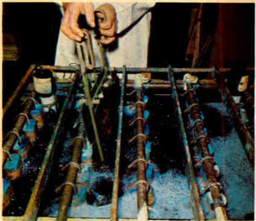
Unwanted section of copper is removed by etching in acid bath.
