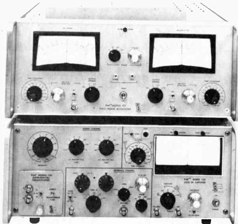
PAR model 126 Lock-In amplifier (bottom) and model 127 two-phase accessory.
