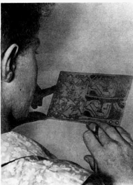
Finished circuit board is checked for faults.
