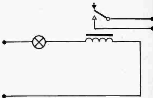
Relay closing times can be substantially reduced by overdriving the relay coil.
