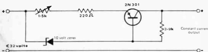
A series transistor is used as a variable resistor in this simple constant current regulator.
