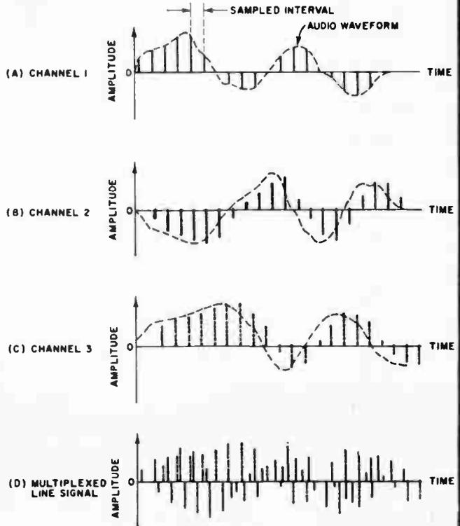
FIG. 3. Sample of time-division multiplexing using pulse-amplitude modulation showing how three (A, B and C) signal voice channels are (D) interleaved in time to form a single, higher-speed pulse train and fed to common line for encoding.
