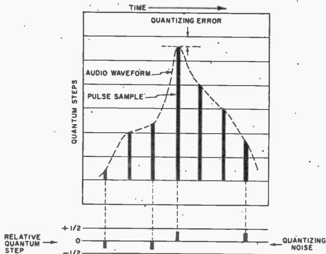
FIG. 4 (LEFT). Quantizing noise, or the difference between actual and measured value of each pulse, is produced only in presence of voice signals whose amplitudes do not coincide with an exact quantum step. Maximum error per sample can't exceed one half size of quantum step.
