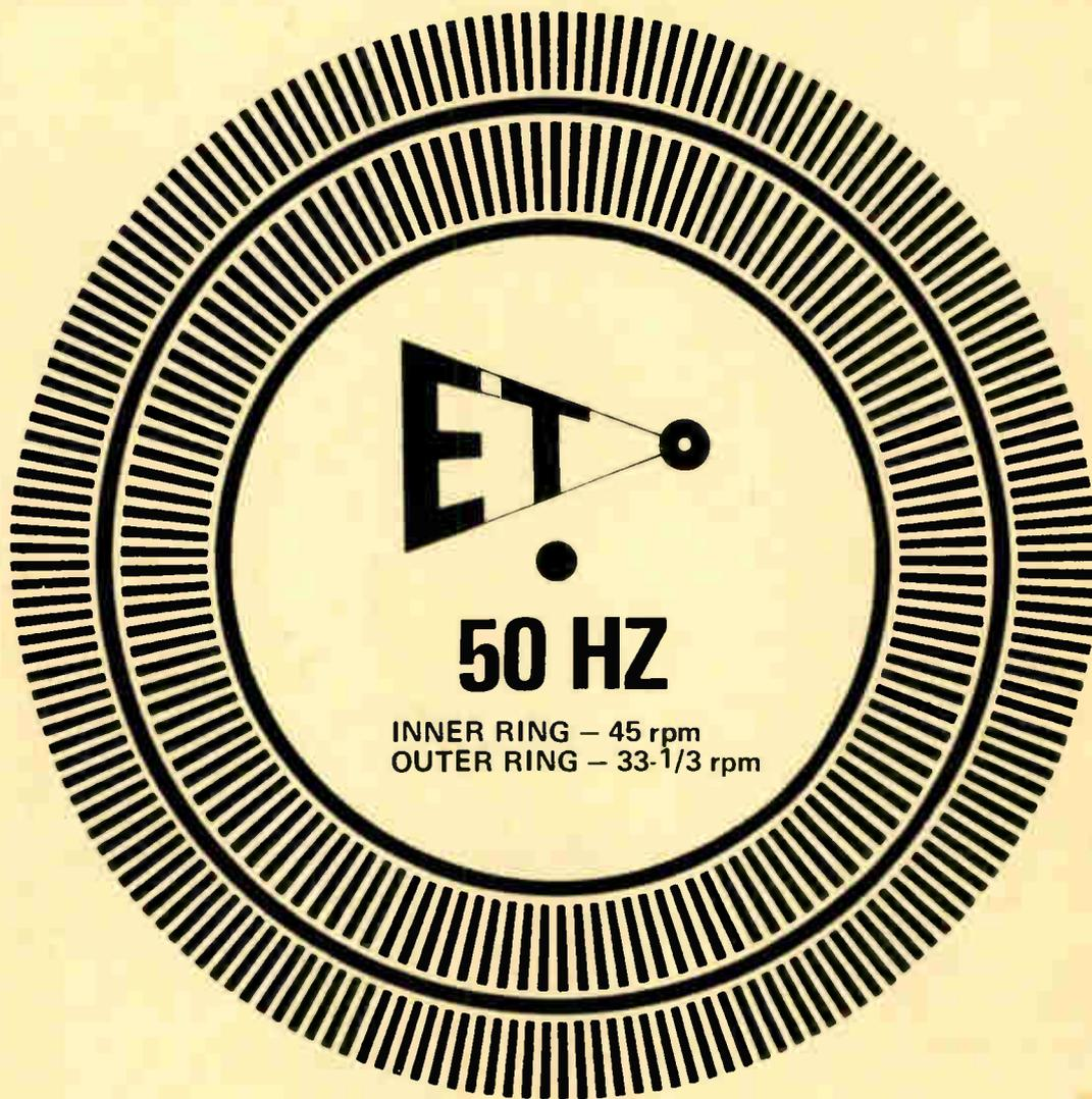
ELECTRONICS TODAY's stroboscopic disc enables the 50 Hz mains to be used as a reference for checking turntable speed.
