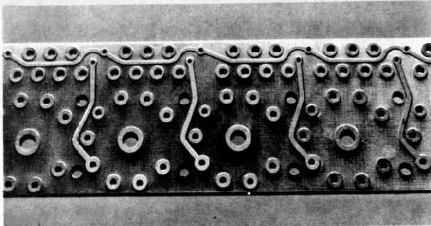
Plated through holes allow component location on both sides of a circuit board.
