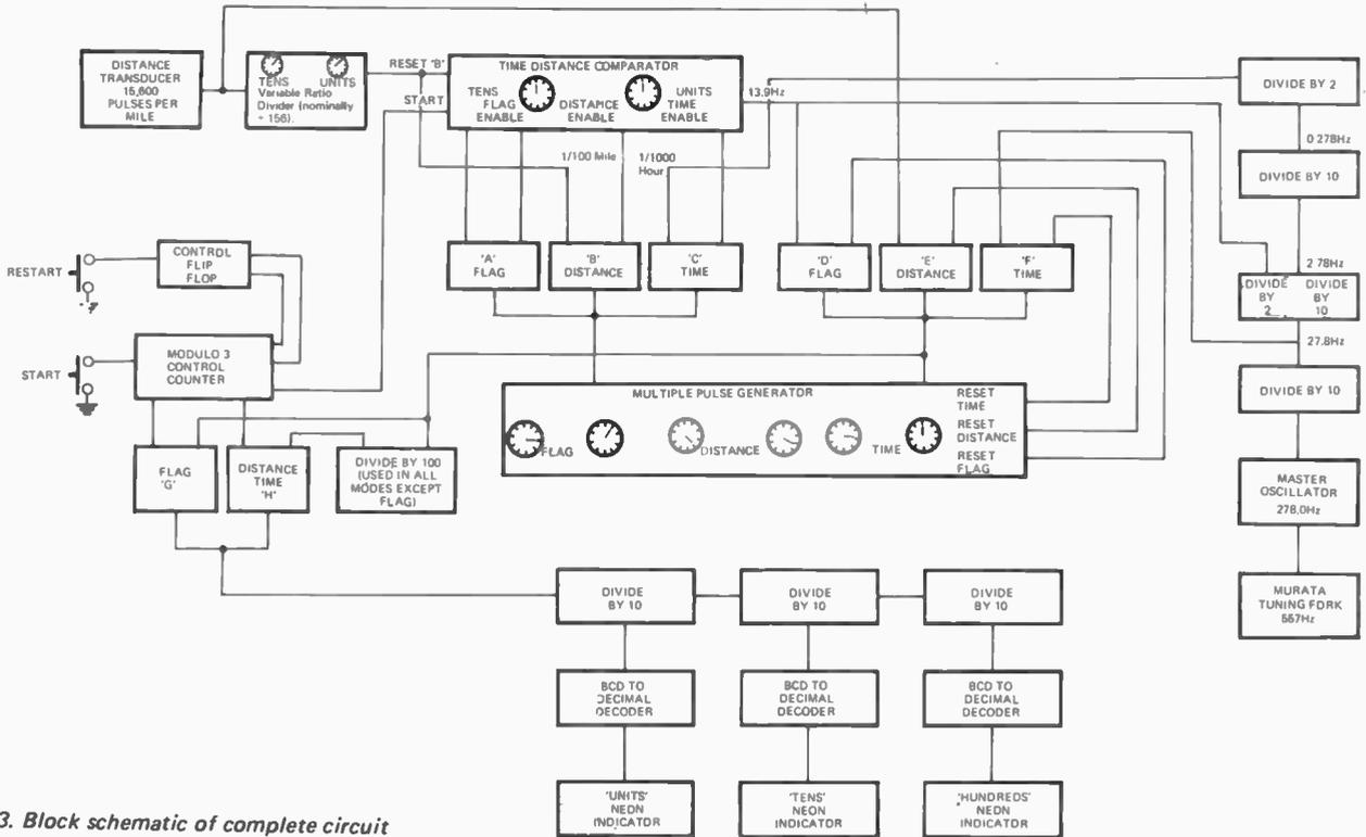
Fig 3. Block schematic of complete circuit
