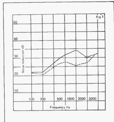
To reduce sound transmission to acceptable levels we must (on average) provide a further 25dB attenuation.
