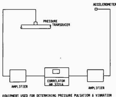
EQUIPMENT USED FOR DETERMINING PRESSURE PULSATION & VIBRATION
