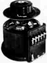
ensuring low magnetising current is covered in a toroidal winding, one face of which is prepared for the self aligning brushgear. Berco Regavolts give a smooth continuous variation of AC voltage from zero to 110% of input line voltage. They are available in ratings from 25VA to 31.5 KVA and can be used singly or in ganged combinations.
