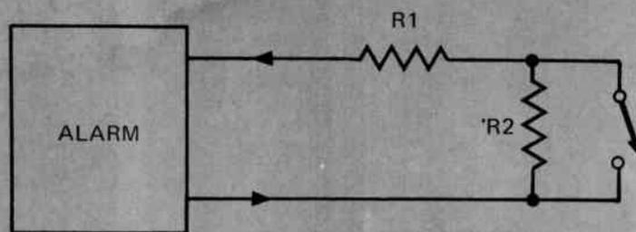
FIG. 2. Resistance R2 represents leakage path across alarm contacts.
