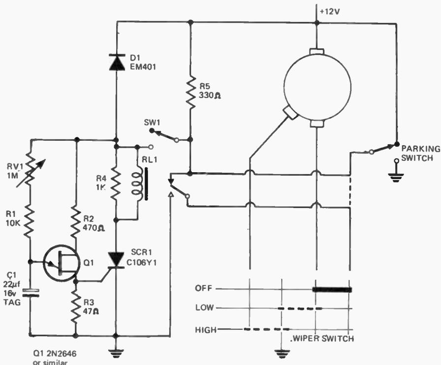
Fig.2. Vari-wiper basic circuit.
