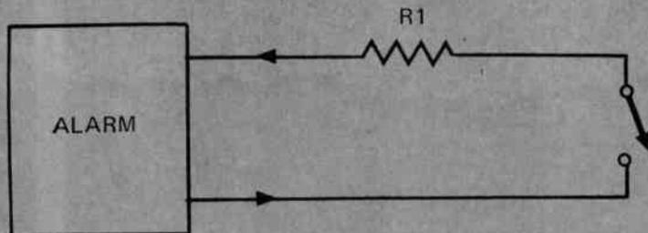
FIG. 1. Resistance R1 represents series resistance of loop (see text).
