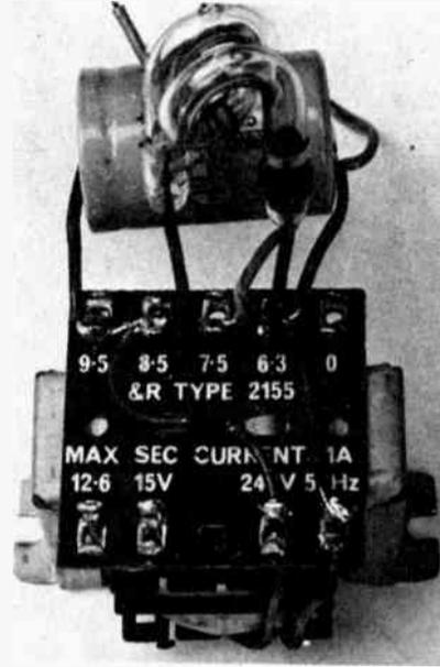
Fig. 2: Xenon flash tube and capacitor C1 mounted on mains transformer.
