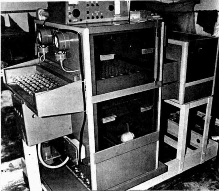
*Spray cleaning machine speeds up manufacturing process.*
