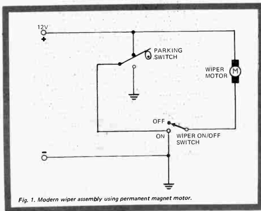
Fig. 1. Modern wiper assembly using permanent magnet motor.
