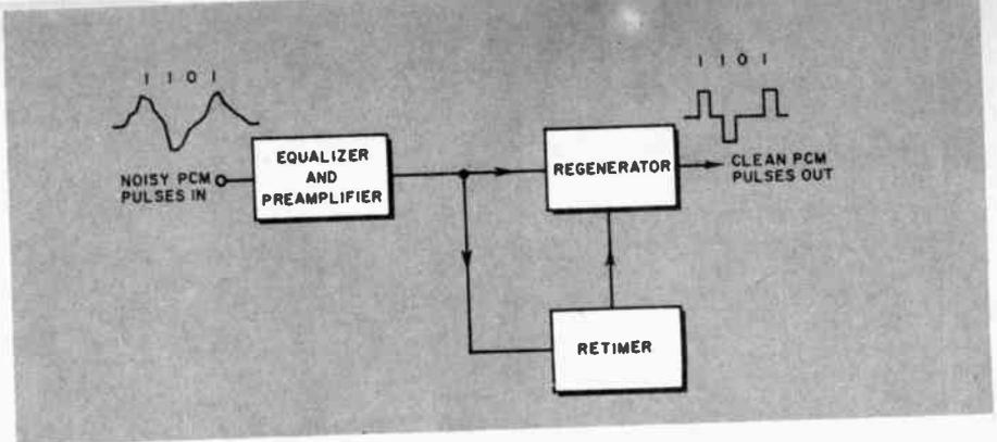
FIG. 9. Simplified block diagram of a digital repeater.
