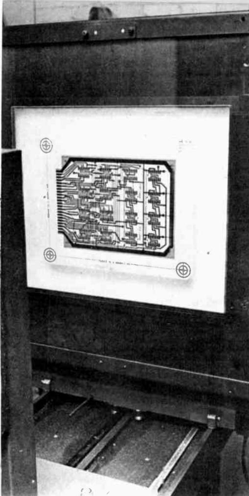
Precision camera reduces master pattern to required final size.
