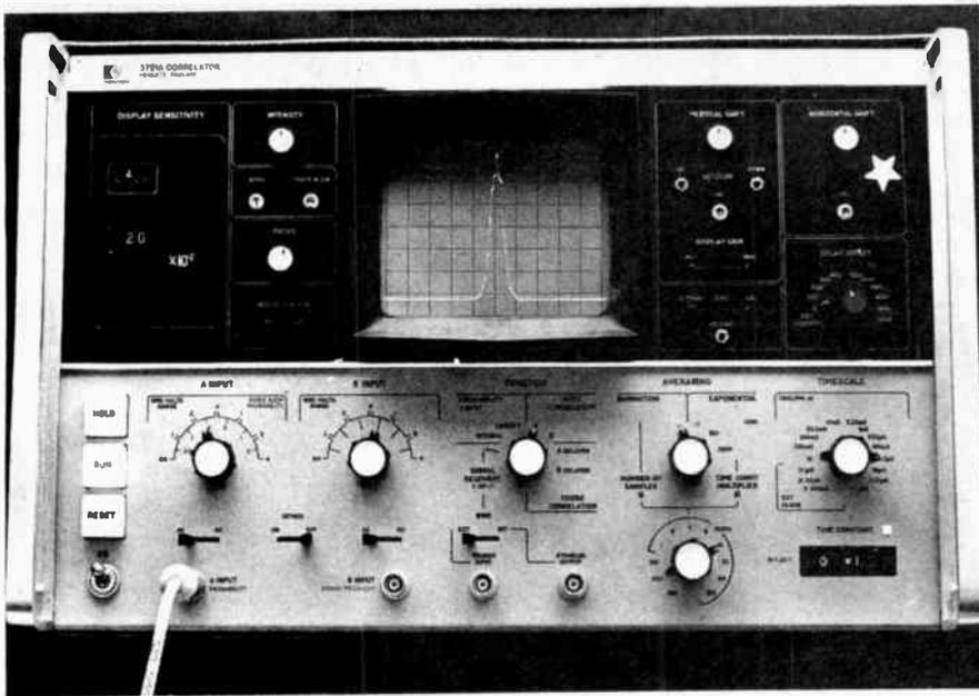
USE OF CROSS CORRELATION TO DETERMINE THE TRANSMISSION LOSS OF A PARTITION
