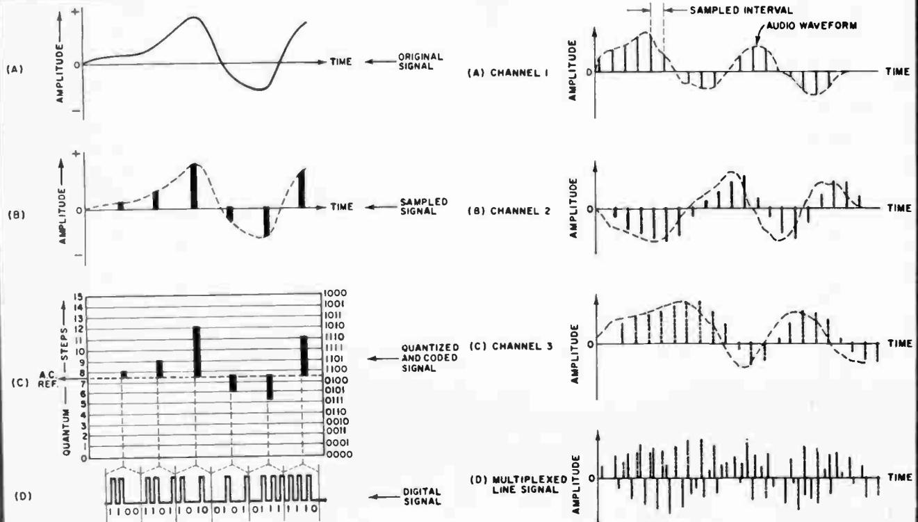
FIG. 2. Basic steps. (A) Original speech signal is (B) sampled to produce pulses corresponding to instantaneous voltage amplitude of audio waveform which is then (C) quantized into incremental levels and (D) encoded into equivalent digital signal.
