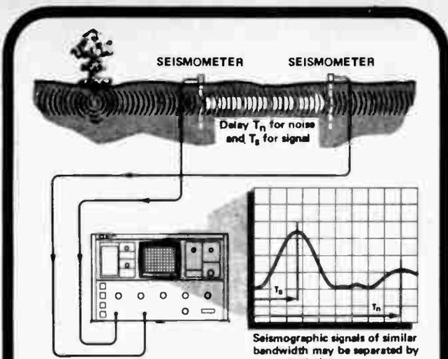
Seismographic signals of similar bandwidth may be separated by crosscorrelation.
