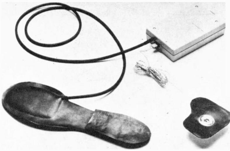
Complete kit consists of a rubber inner sole with small air chamber (left), connected by a tube to a pneumatic switch in a pulse generator (top right) which in turn is connected to an electrode (bottom right).
