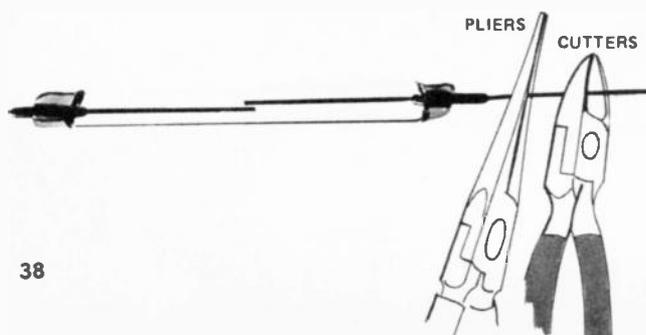
Fig. 12. Care must be taken if the reed switch connecting leads needs shortening. Hold wire tightly with pliers (as shown) to prevent breaking the glass seal.
