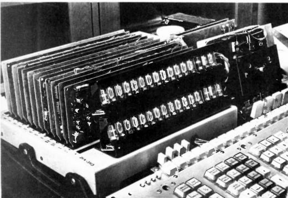
Readout is displayed on this bank of neon indicator tubes.
