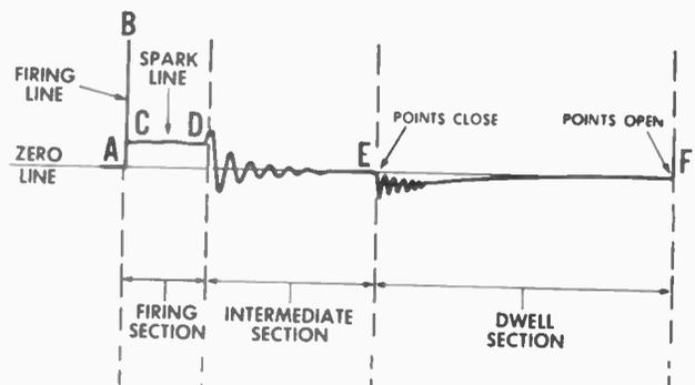
**FIG. 1 — BASIC SECONDARY WAVEFORM**
