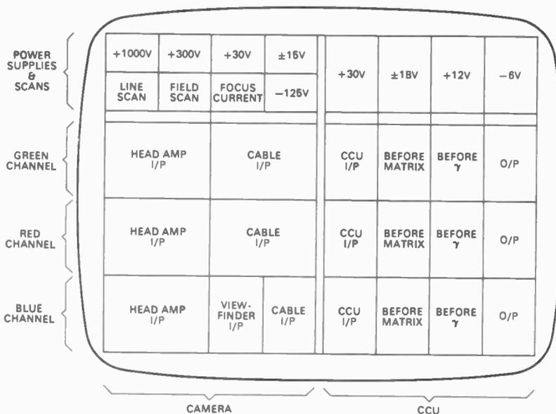
*Automatic test display offered with the automatic colour camera. The screen remains white except when there is a fault, the area at fault being indicated as shown on the diagram.*
