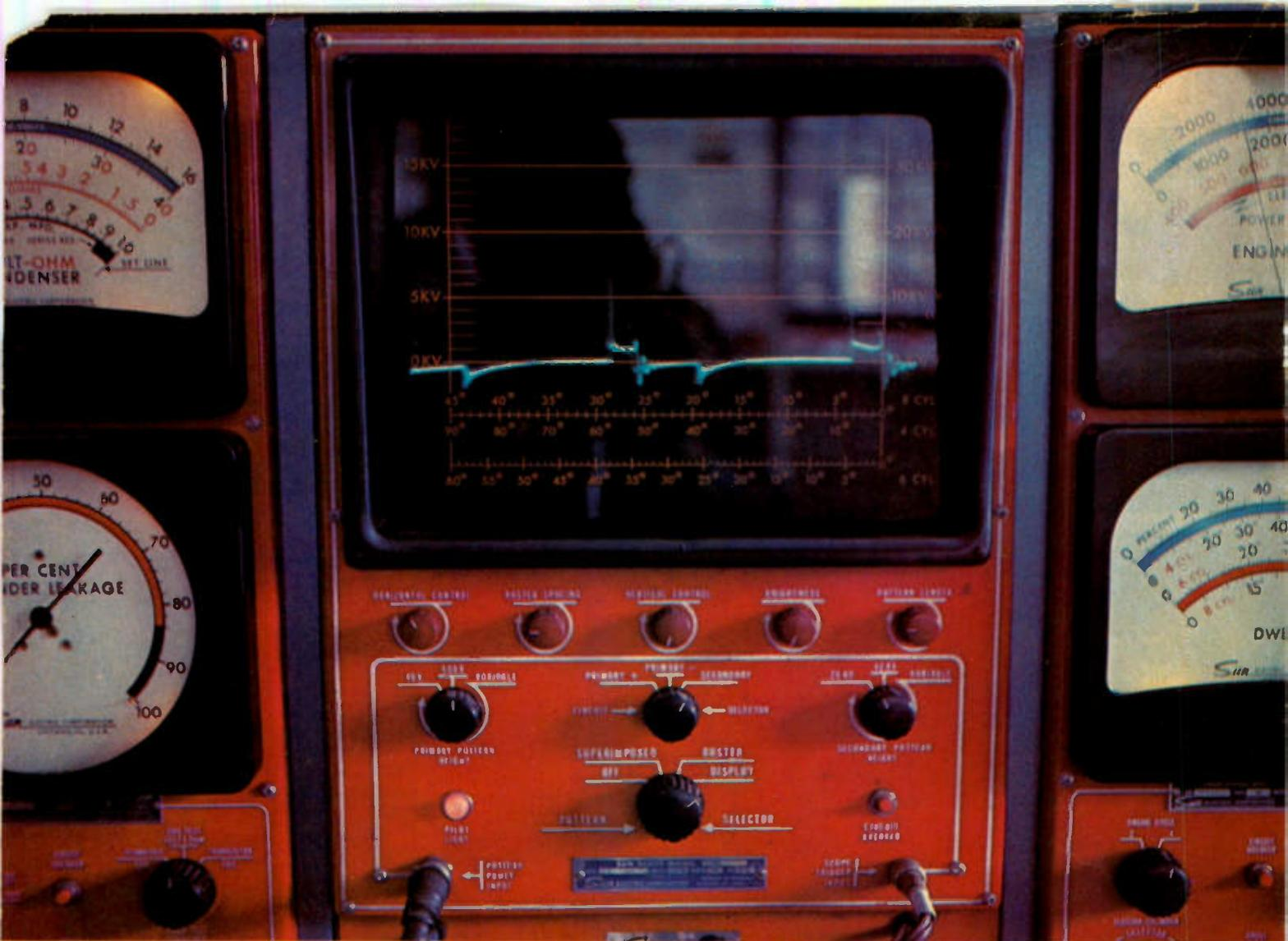
ABOVE: One complete cycle of ignition is displayed on screen of Sun oscilloscope — compare this picture with Fig. 1 in main text.
