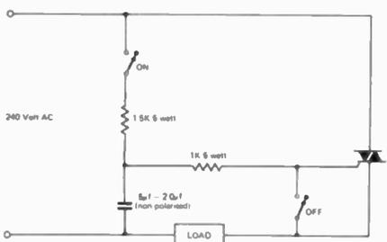
**Fig. 10. This triggering circuit provides latching action.**
