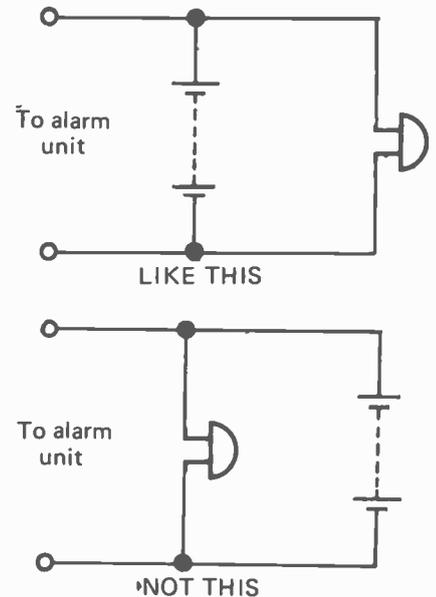
Fig. 14. It is preferable to power the bell from a separate battery — if the main alarm battery is used, the power to the bell must be taken directly from the battery.
