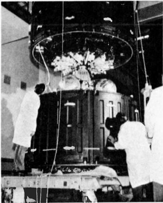
*With sensitive solar cells clad in protective metal covers, engineers at Hughes Aircraft Company carefully fit together the top and bottom halves of a full-scale thermal model of the Intelsat-IV communications satellite during thermal testing. The satellite was equipped with more than 300 sensors to record temperature variations during the test which simulated the heat and cold to be encountered in orbit.*
