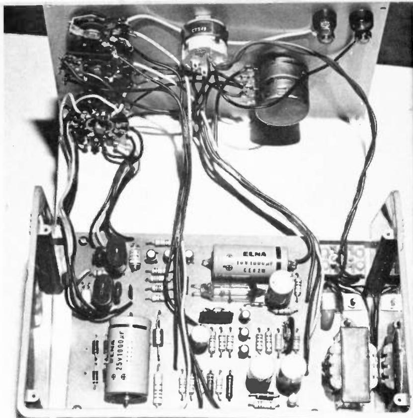
Fig. 4. General layout of components, in our final version we found it was desirable to use screened signal leads between the circuit board and the panel mounted switches.
