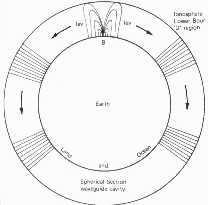
Fig. 3 illustrates a two dimensional view of the propagation of the electric field vector  $fe_v$  omnidirectionally, with vertical polarisation. Note that to a first approximation the ray path illustrated by the arrow is substantially tangential. (For higher frequencies it zig-zags in the familiar series of hops).
