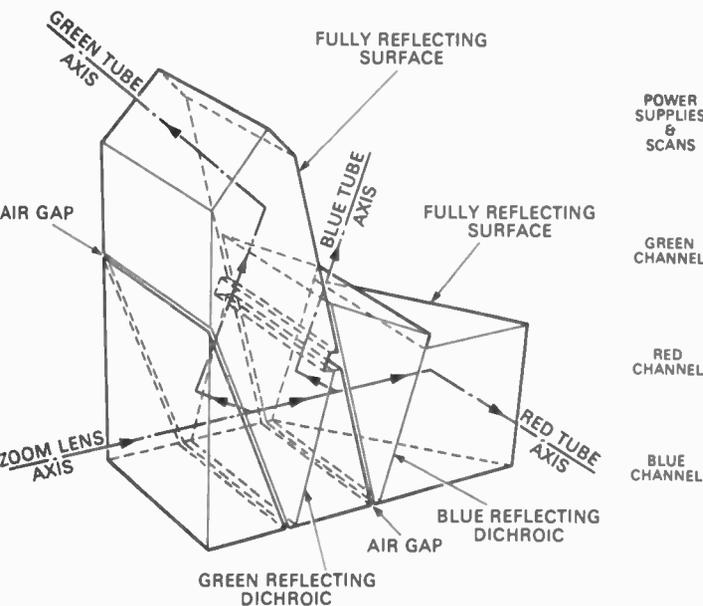
*Simplified diagram of prism system used in the Marconi mark-VIII automatic colour camera.*
