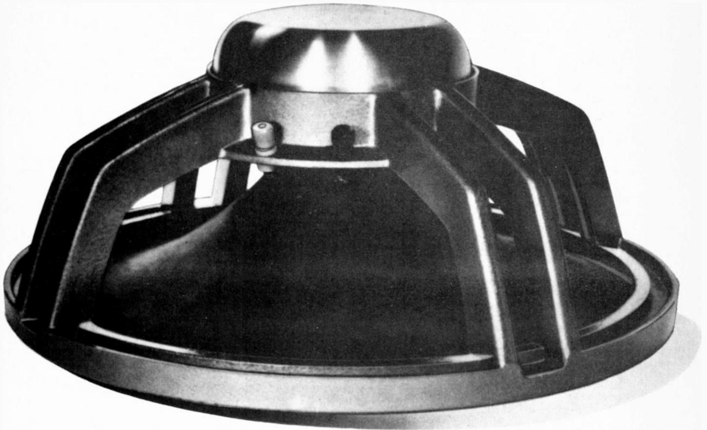
MSP 15" Woofer model 15VAC fulfils a requirement where high power handling and quality reproduction of bass frequencies are of prime importance. It features a nominal 35Hz resonance and this coupled with an exponential cone form allows smooth frequency coverage from 30Hz to 6kHz.
