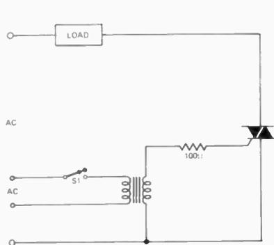
Fig. 7. Isolated ac provides triggering.
