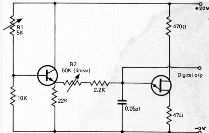
R2 is a low friction potentiometer used as angular position indicator.
