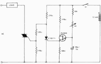
**Fig. 11. Time delay circuit — power is disconnected from load after pre-set time.**
