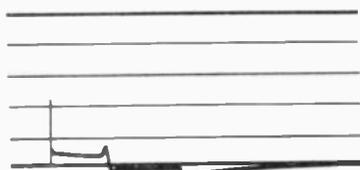
Fig. 7. Lack of oscillations in intermediate section indicates faulty coil or condenser.
