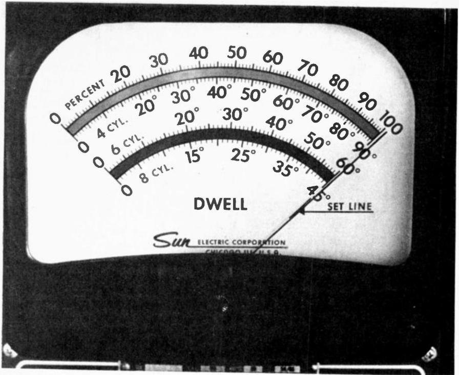
Dwell meter measures angle through which distributor cam turns while the contact breaker points are closed.
