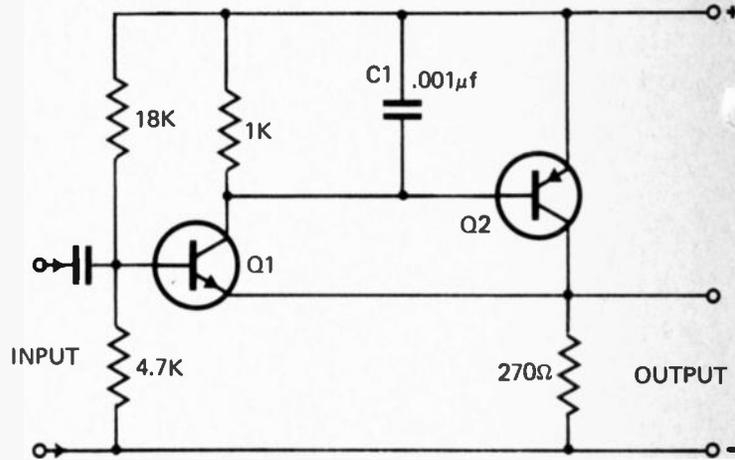
Output impedances as low as 0.05 ohm can be obtained by using this configuration.
