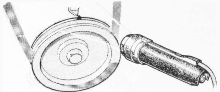
Ignition timing is set using strobe light triggered by firing of number one spark plug. Fig. 13.
