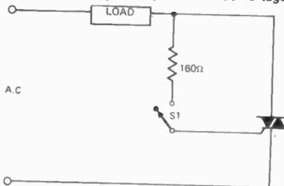
Fig. 3. Triac is triggered by input ac, in this application switch S1 will be 'live'.
