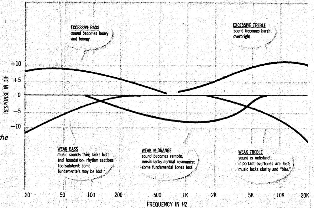
Importance of wide-range, linear response is shown by this graph of frequency response plotted against signal level in decibels. For accurate music reproduction, the entire 20-Hz to 20,000-Hz range should not vary by more than a decibel or two above or below the zero reference line.
