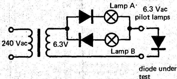
If lamp A or lamp B is illuminated the diode is serviceable. If both light the diode is short circuit. If neither light, diode is open circuit.
