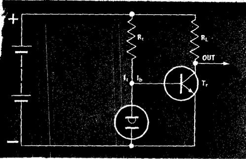
Fig. 4. The basic 'E' Cell device with a semiconductor interface. This circuit can be used as a basic timer and readout circuit.
