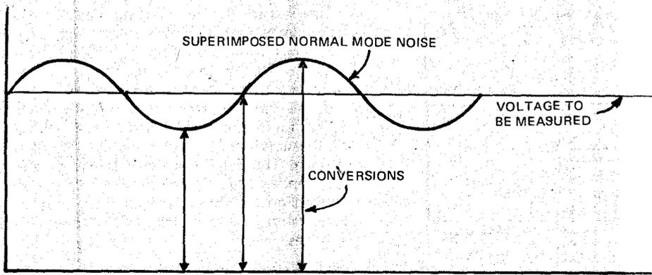
Fig. 3C. Effect of noise on ramp type A/D converter.
