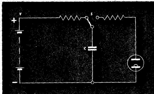
Fig. 6. Counting pulses with the 'E' Cell. Each time switch S is actuated, a charge  $Q=C_1 V$  is set in the 'E' Cell.
