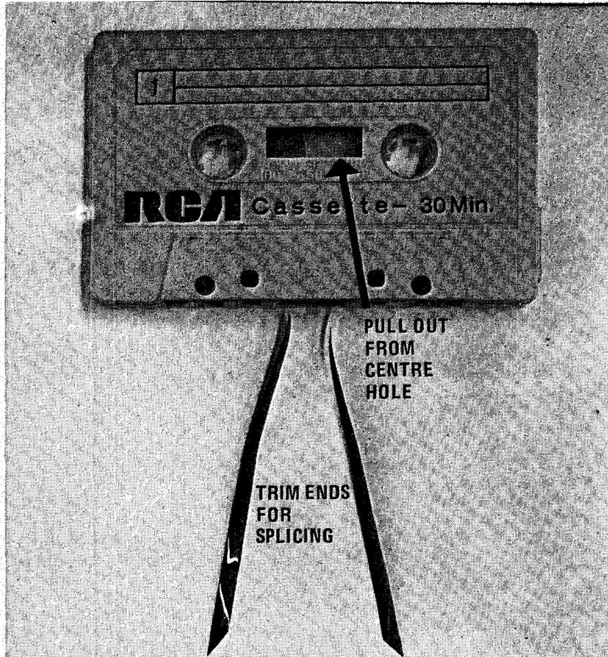
FIG. 3 — TO TRANSFER TAPE from jammed cassette to new cassette, start by pulling out tape leader end. See text for full description.
