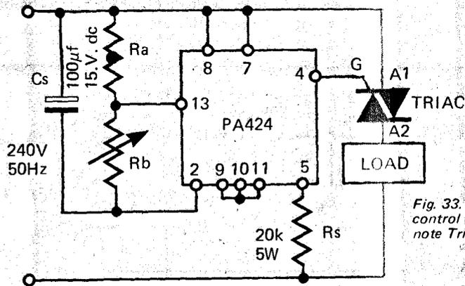
Fig. 33. Basic temperature control circuit uses PA 424. note Triac connections.
