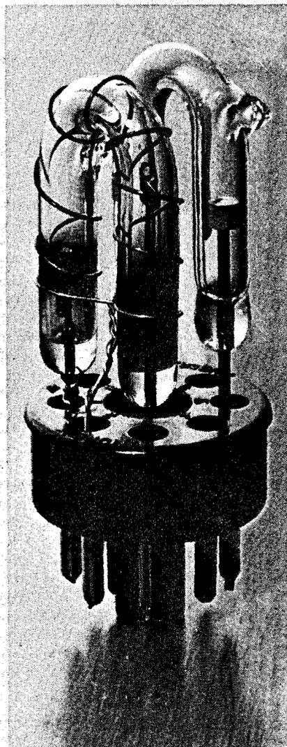
Fig. 4. Two strobe-tubes are mounted in one octal holder. The Circuit Components tube is on the left, and the Philips tube is on the right. Note that a triggering lead must be attached to the Circuit Components unit. The wire is simply wrapped around the tube as shown.
