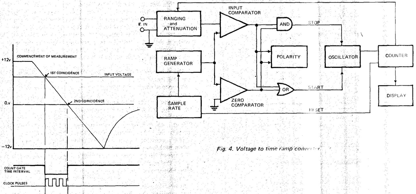
Fig. 4. Voltage to time ramp converter.
