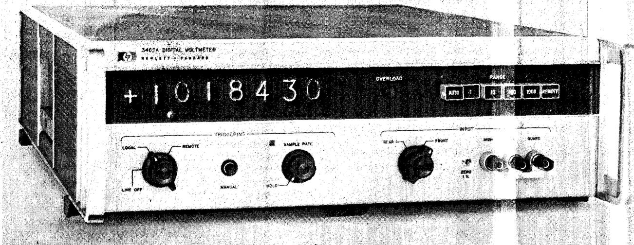
Hewlett-Packard's 3462A digital voltmeter uses potentiometric-integrating principle.
