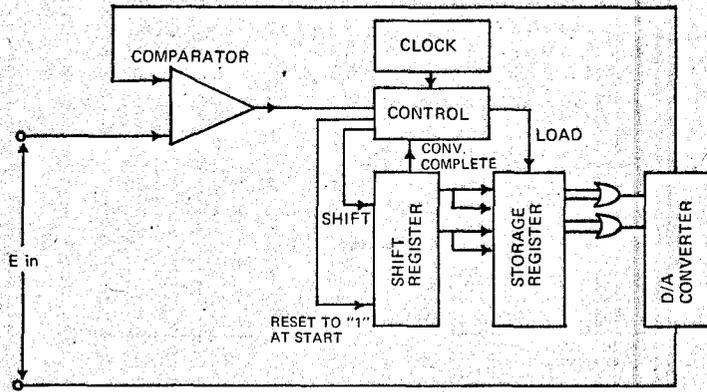
Fig. 6. Successive approximation converter.
