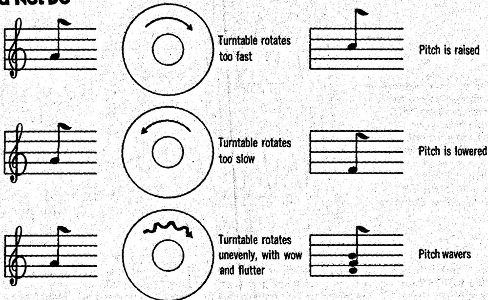
Music can be distorted if the medium playing it does not run at true speed. Examples shown here for turntables apply also to tape decks. Musical notation has been slightly exaggerated for clarity. See article for detailed explanations.
