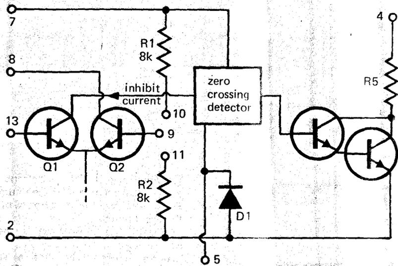
Fig. 32. Simplified schematic of PA 424 integrated circuit.
