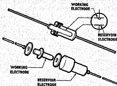
Fig. 1. Cross-sectional and exploded view of the 'E' Cell device, together with its electrical symbol.
