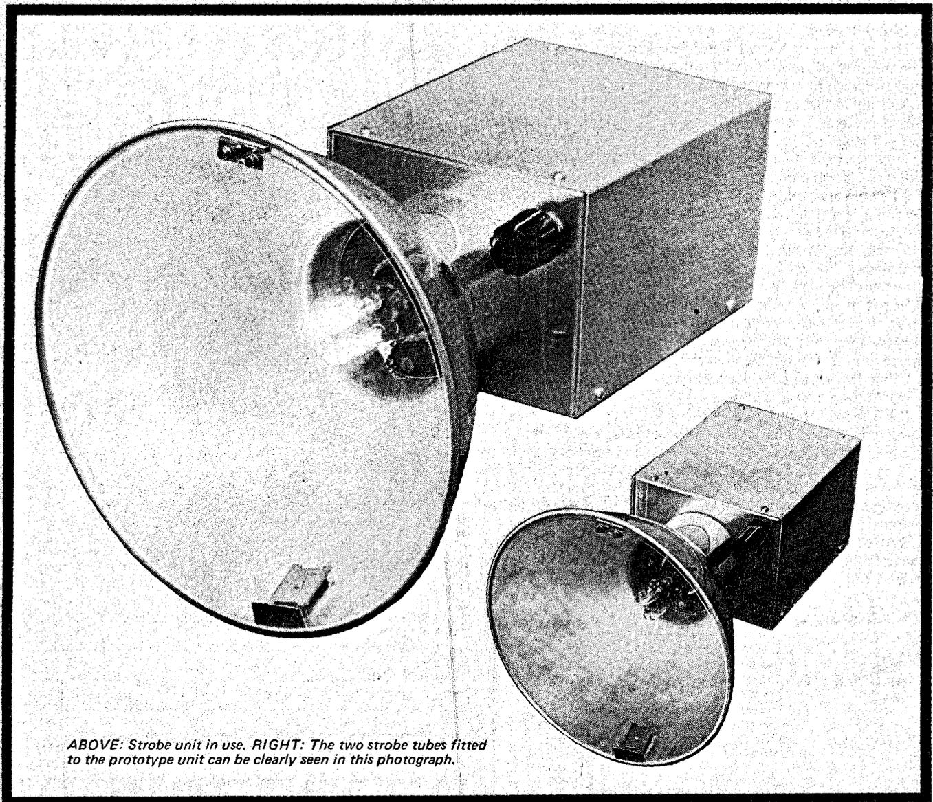
ABOVE: Strobe unit in use. RIGHT: The two strobe tubes fitted to the prototype unit can be clearly seen in this photograph.
