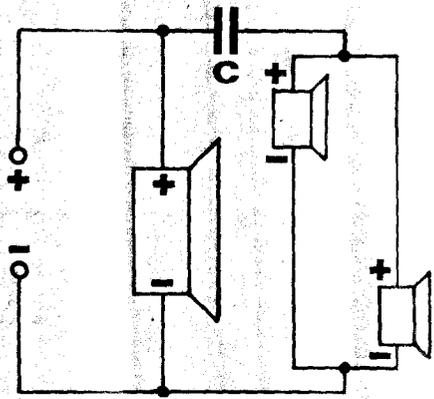
Connect speakers as shown in this drawing — observe polarity as indicated.
