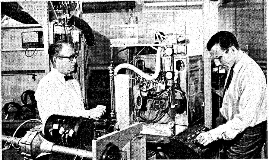
Experimental 14 kilowatt-hour prototype zinc-air battery operates drive train for a small electric-powered vehicle at General Atomic Division of General Dynamics in San Diego, California.
