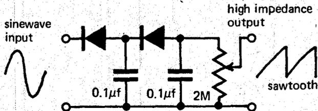
Here is a circuit that can be used in simple oscilloscopes or RF sweep generators. It works best with low frequency sinewave inputs.
