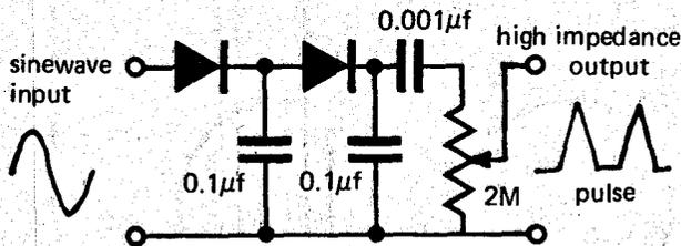
This circuit is useful in adjusting noise blankers for producing time marker pulses for a CRO or chart recorder. The high impedance output is adjustable by the two Megohm potentiometer. Peak inverse rating of the diode should be high enough for input voltage used.
