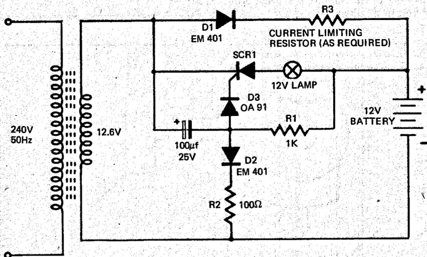
The 12 volt lamp shown in this circuit should be rated at 12 watts or less — this may be increased to 24 watts if the SCR is mounted on an adequate heat sink.
