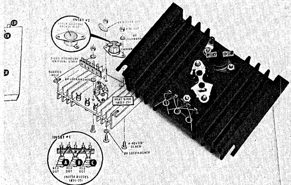
The partially completed heat sink assembly is shown here alongside the relevant instructions in the Heathkit manual.
