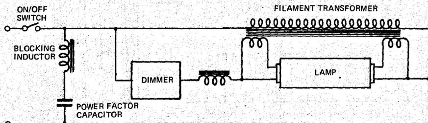
FIG. 5. FITTING OF P.F. CAPACITORS TO DIMMING FITTING
