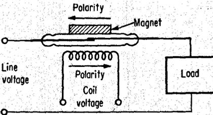
Fig. 14. Normally closed operation using magnetic bias.
