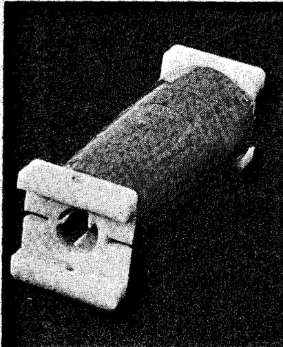
Fig. 11. Bobbin for standard sized reed switch.
