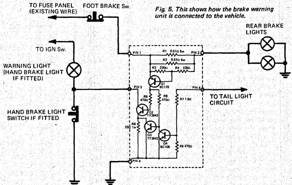
Fig. 5. This shows how the brake warning unit is connected to the vehicle.
