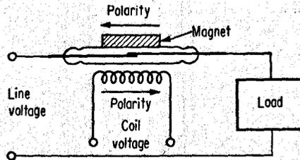
Fig. 14. Normally closed operation using magnetic bias.
