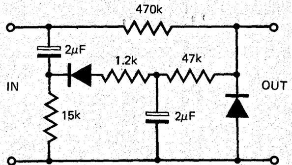
Here is a simple compressor that is very effective when recording from the speaker terminals of a receiver.
