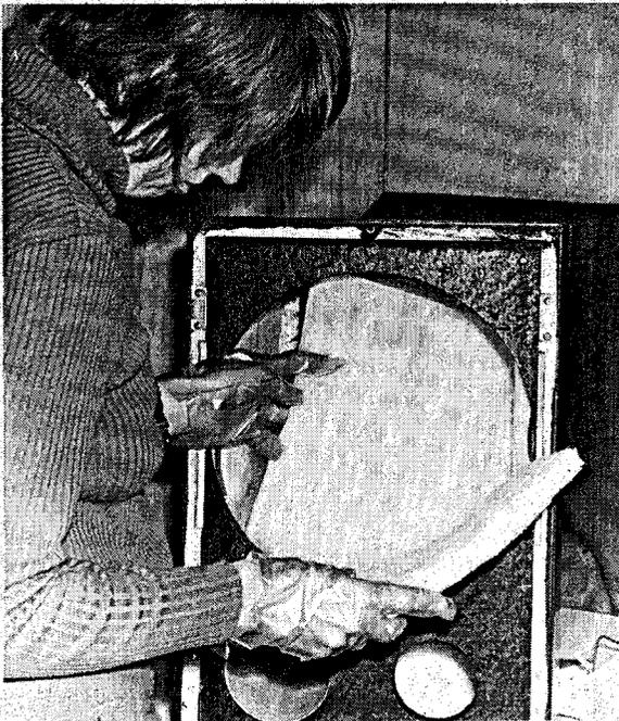
Installing the glass fibre lining in one of the loudspeaker enclosures — even the gloves were supplied.
