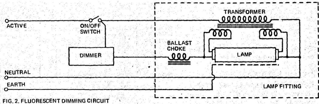
FIG. 2. FLUORESCENT DIMMING CIRCUIT
