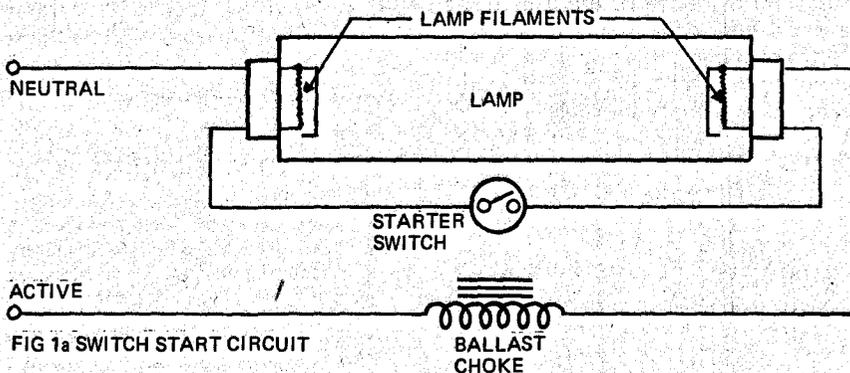
FIG. 1a SWITCH START CIRCUIT
