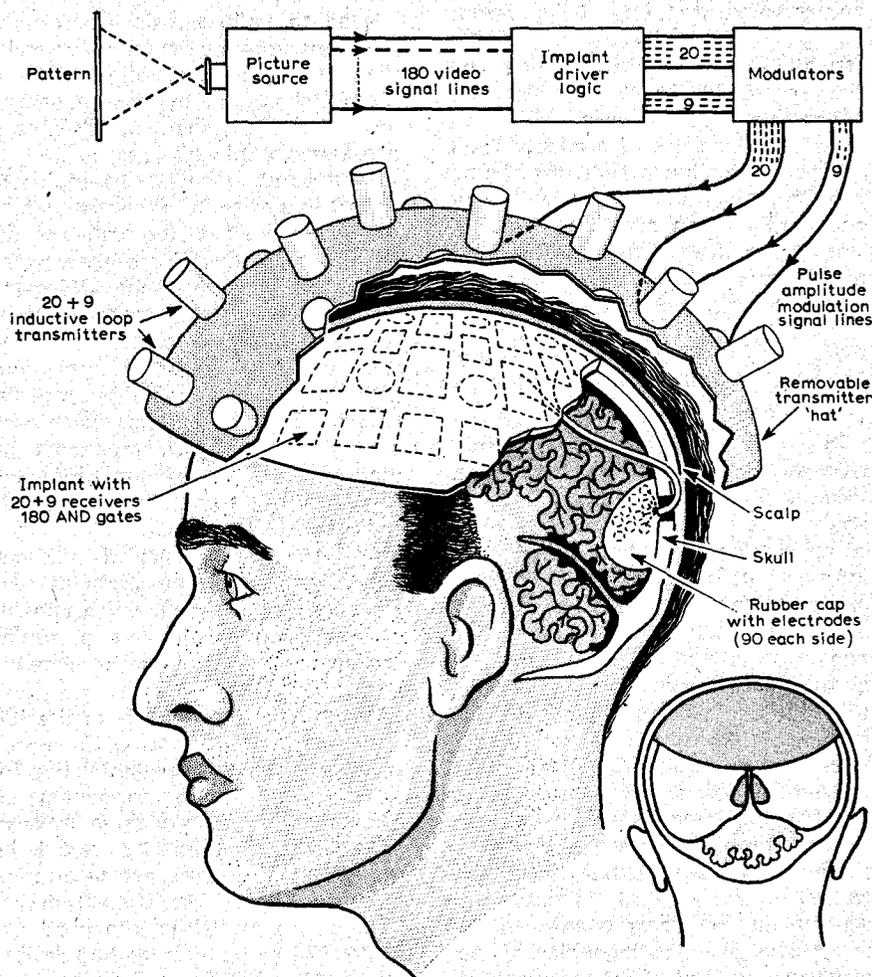
*Principle of the visual prosthesis. The visual cortex of the brain is stimulated by electrodes fed from microelectronic receivers in an implant between the brain and the scalp.*
