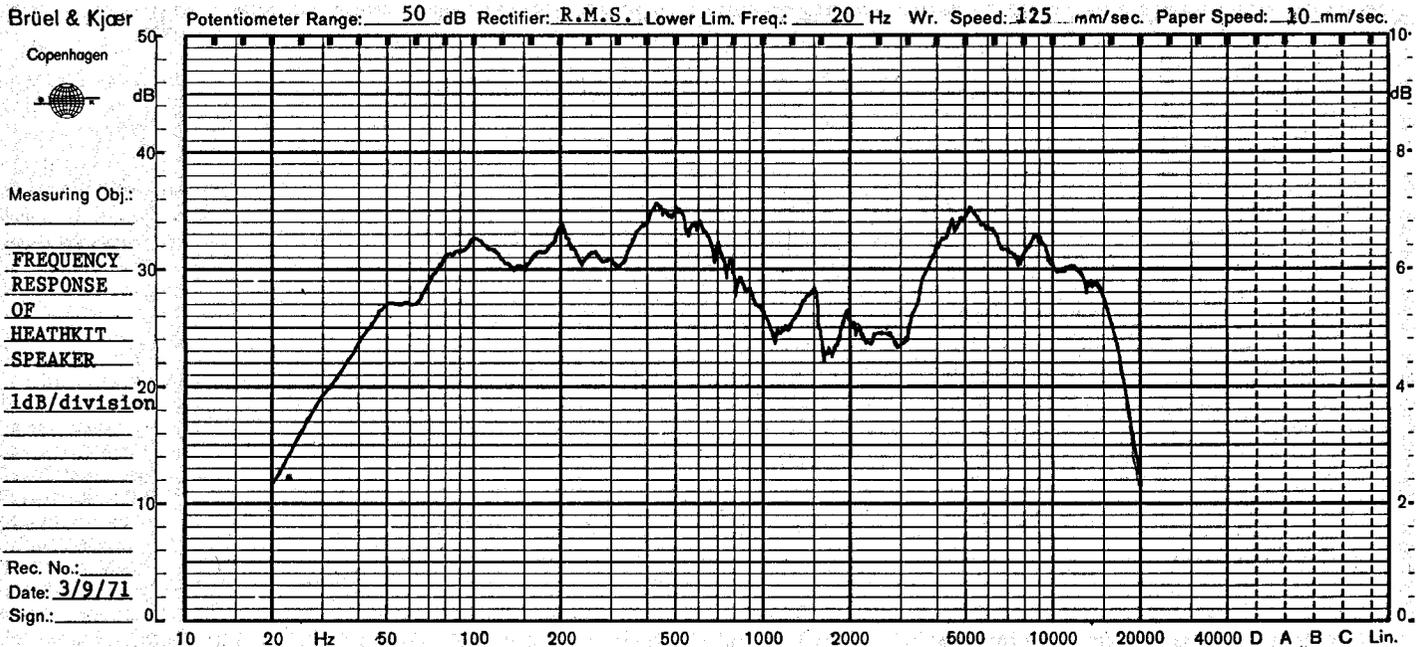
The components consisted of a 14" diameter JBL woofer and a 2½" diameter JBL tweeter, together with full LC crossover networks. All were housed in a vented enclosure finished in dark polished walnut veneer.
