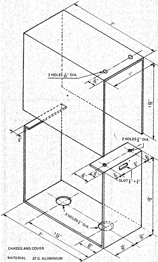
Fig. 4. Details of metalwork.
