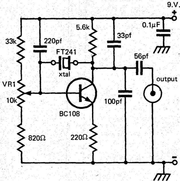
Surplus FT 241 crystals (340 to 580 kHz) are very useful in a variety of applications. But it is sometimes difficult to obtain reliable oscillation in many standard circuits.
