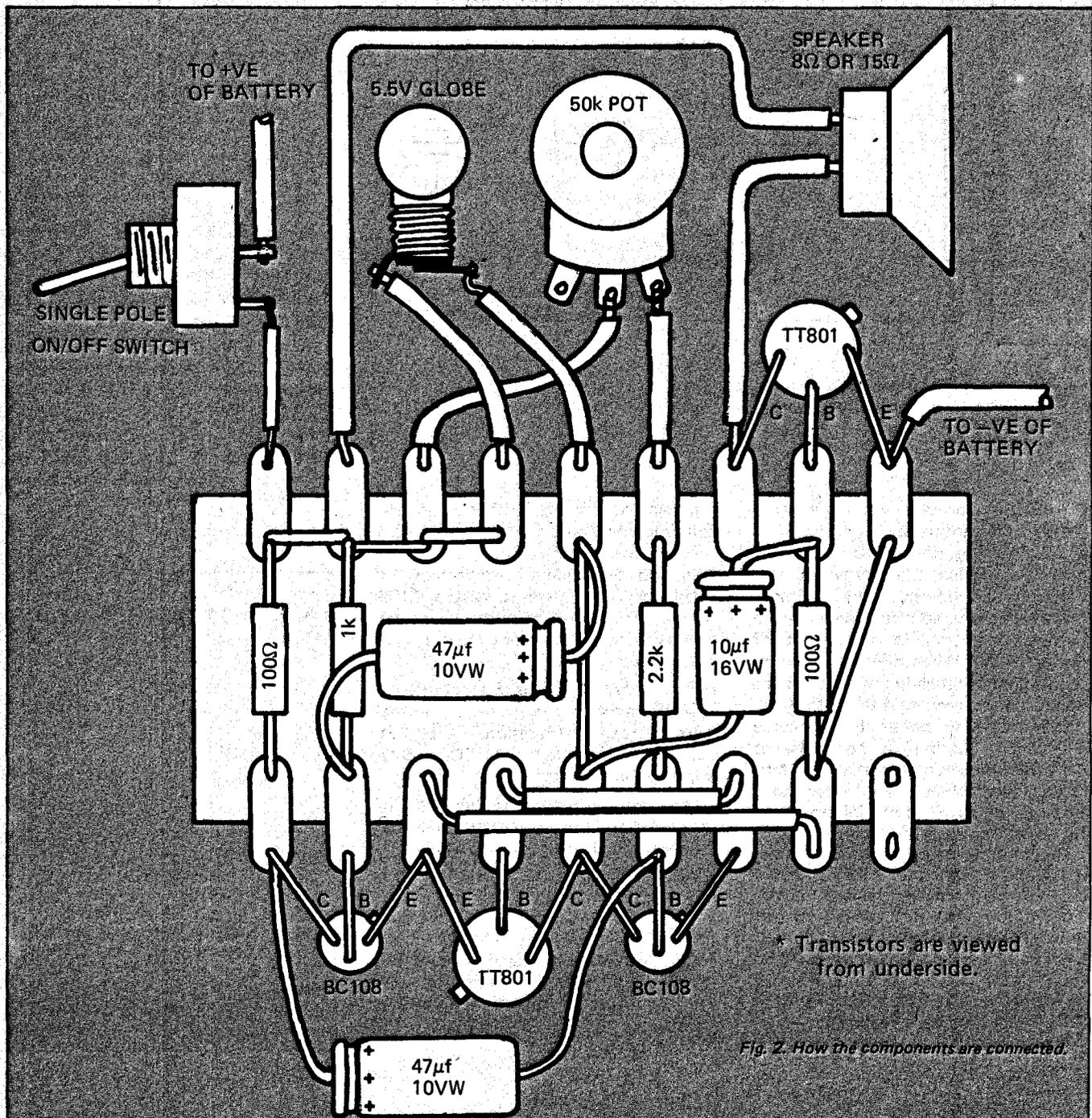
Fig. 2. How the components are connected.
