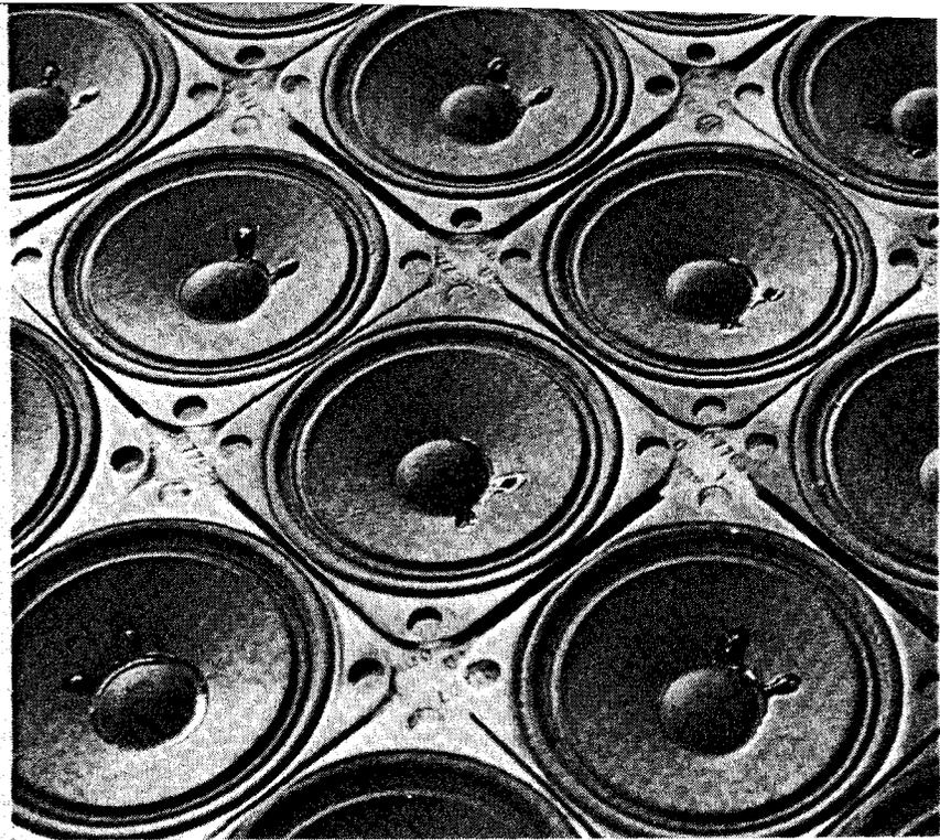
*In the magnetic speaker, amplifier signals energize a voice coil; the changes in its magnetic field cause the diaphragm to vibrate. In the electrostatic speaker, the changing field between a movable plate and one or two fixed pieces produces the motion needed for sound.*
