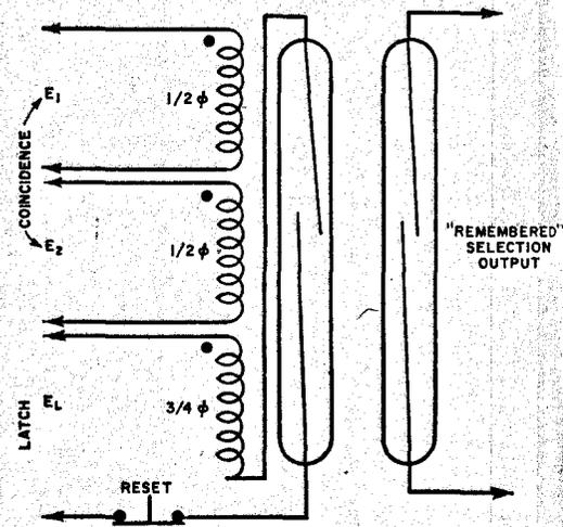
Fig. 22. How a 'memory' may be incorporated in a matrix element.
