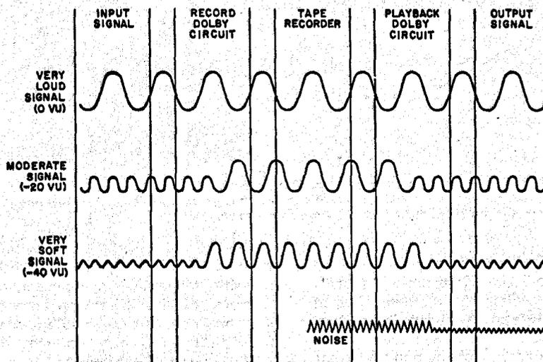
1. The signal being recorded passes through the record Dolby circuit first. The Dolby circuit operates on the higher ("hiss") frequencies in a predetermined manner, depending on their loudness level. The loudest signals (0vu) pass unaffected through the circuit. Signals of moderate intensity (-20vu) are boosted moderately, while the very soft signals (-40vu) receive maximum boost.
