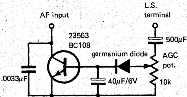
Audio derived automatic gain control is one of the simplest methods of obtaining signal compression in a radio receiver. It is of particular value with short wave receivers used in areas where deep fading is prevalent.
