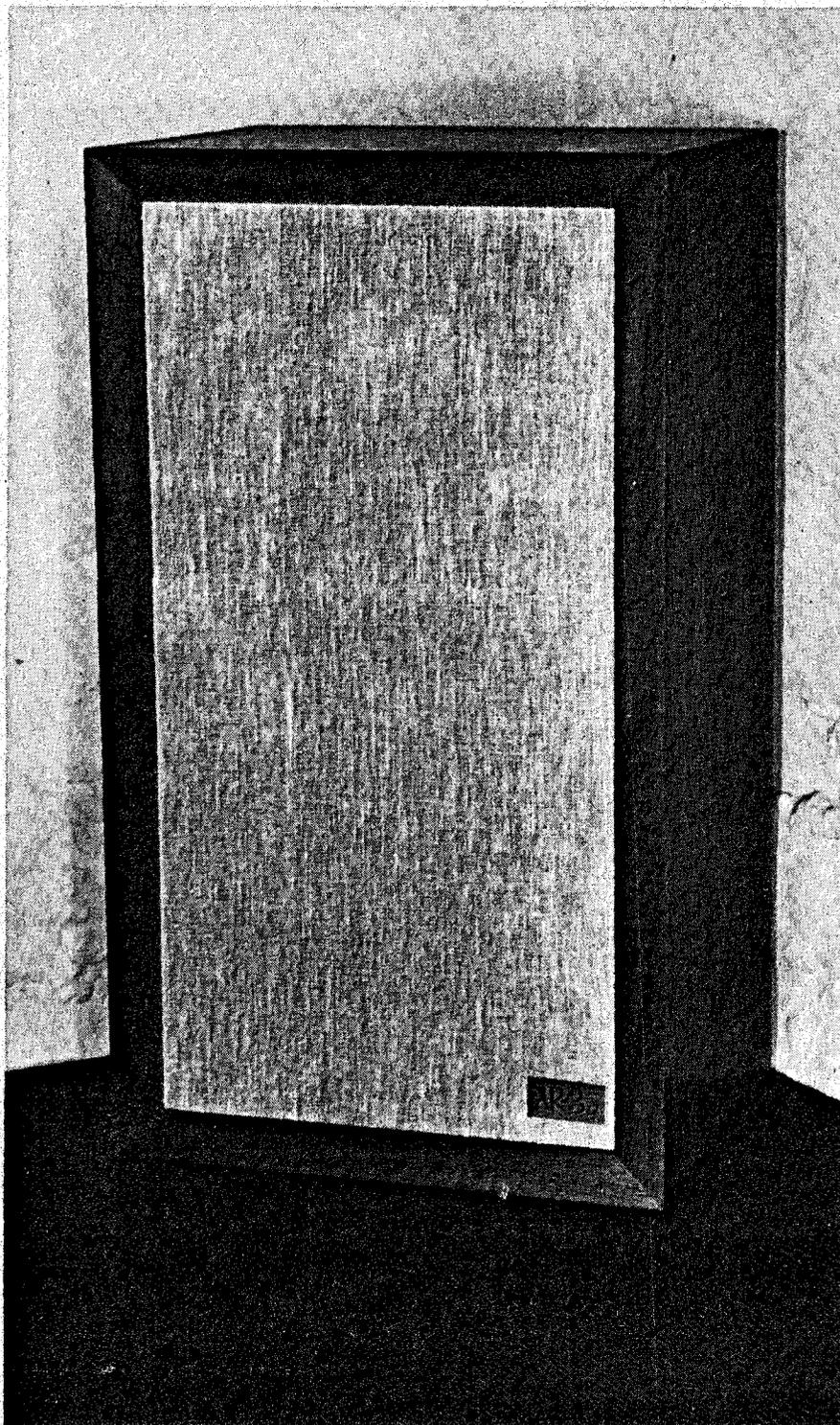
**T**HE Acoustic Research Inc. Model AR-3a speakers are the most sophisticated units that this company have ever produced. They incorporate a number of unusual design features, such as a  $\frac{3}{4}$ " diameter high frequency hemispherical dome tweeter, and a  $1\frac{1}{2}$ " mid-range hemispherical dome speaker. These have a dramatic effect on the radiation pattern at the higher frequencies.
