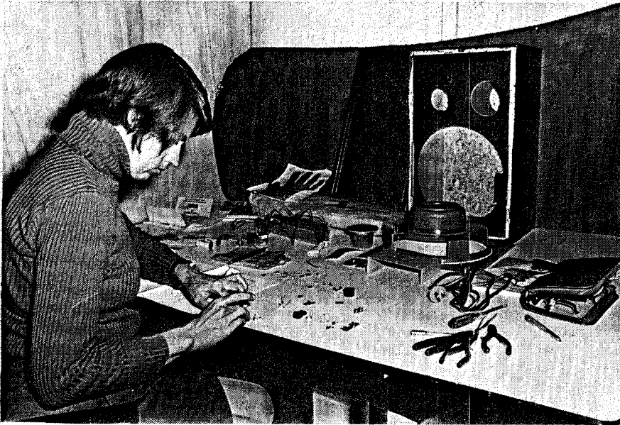
Jan commences assembly of the first of the two loudspeakers — note the massive 14" diameter JBL woofer.
