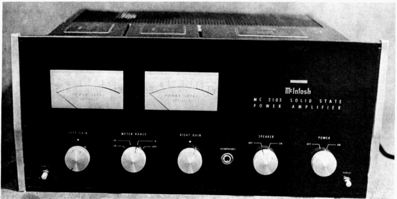
THE McIntosh MC2105 solid state power amplifier is very similar in appearance to the preamplifier. The external finish is identical, with a black glass front panel with chromed trims at each end and machined aluminium knobs.
