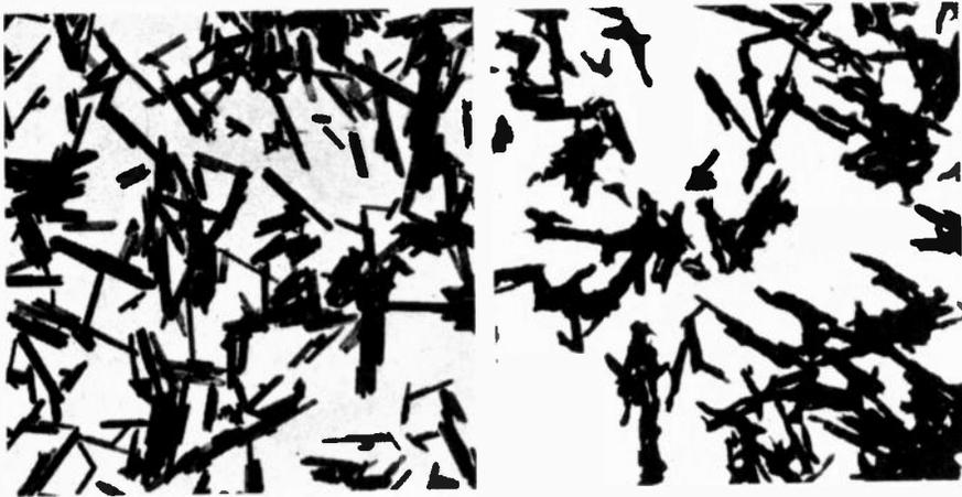
Figs. 1 and 2. Photo-micrographs of chromium dioxide (left) and conventional tape (x20,000)
