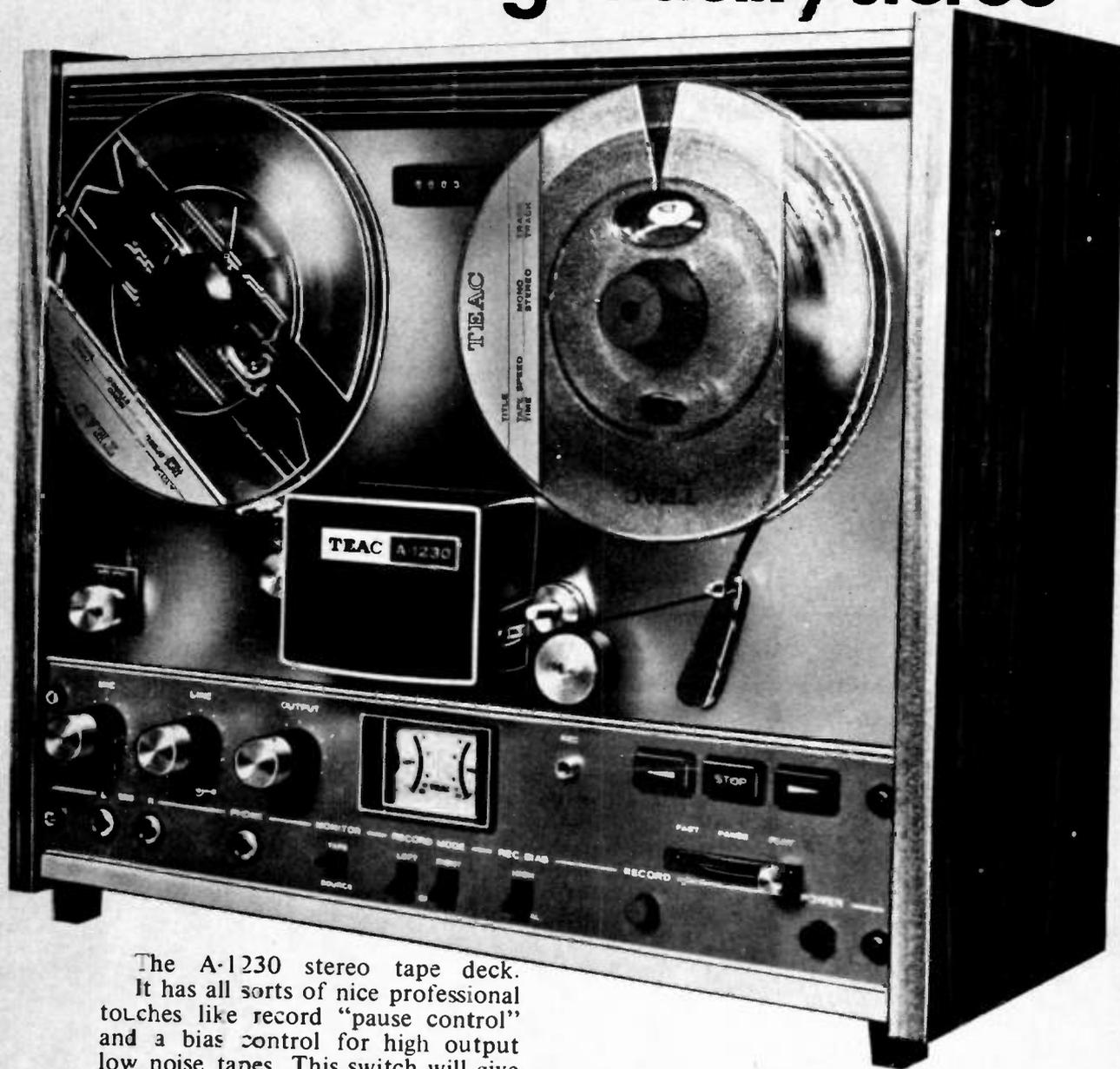
The A-1230 stereo tape deck. It has all sorts of nice professional touches like record "pause control" and a bias control for high output low noise tapes. This switch will give you a wider frequency range and a very impressive signal to noise ratio of 55 dB. Tape recordings "off the air" and from discs will take on a new dimension of fidelity with TEAC's bias control.
