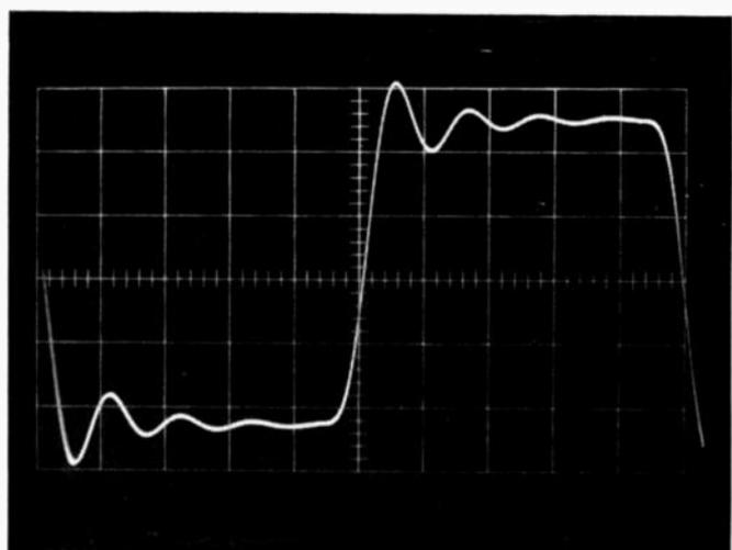
Fig. 4. Record/Replay Response of Bruel & Kjaer 7001 to 200Hz square wave.
