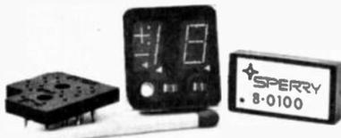
To fill the price gap between low-cost NIXIES and the more expensive LED displays, Sperry Information Displays Division have released its SP-730 series – a seven-segment display available in two-digit and three-digit packages.
