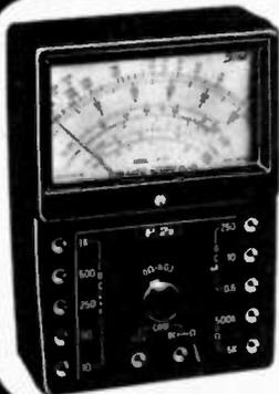
**P-2<sub>B</sub> — A versatile pocket multimeter**
