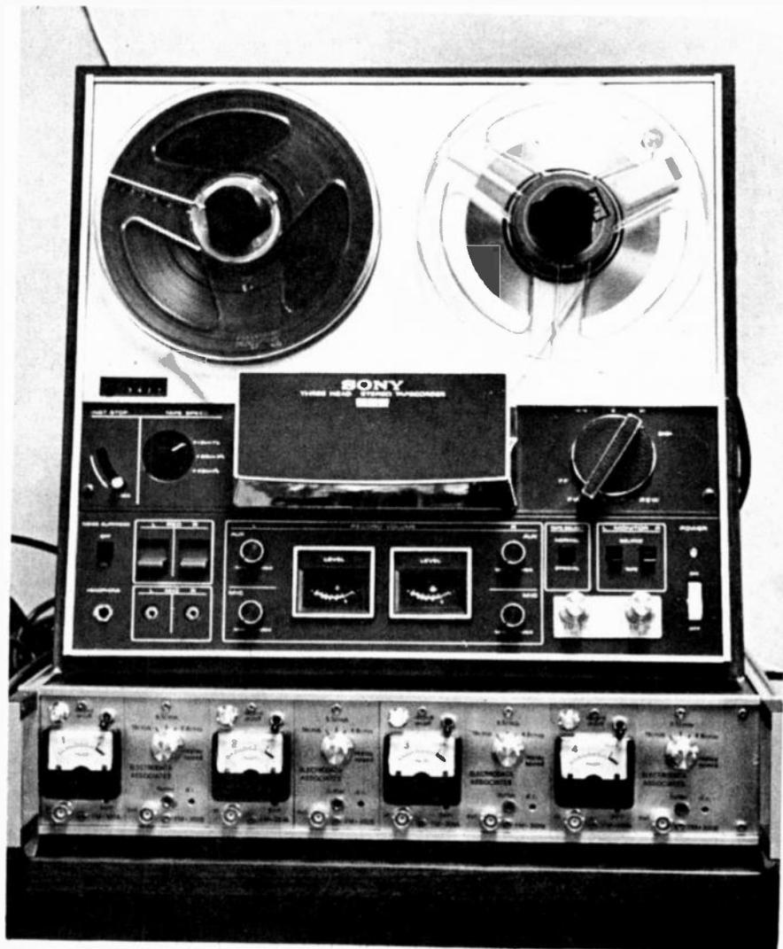
*The Sony TC 366 tape deck is fitted with a four-channel head.*
