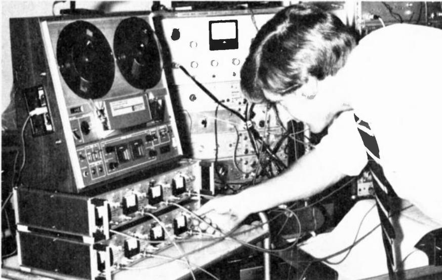
An Australian designed and built eight channel analogue recording system has recently been introduced by Electrodata Associates Pty. Ltd. The model MT465 system incorporates the use of multiplex techniques to record two analogue channels on each tape track. As a consequence, the system incorporates a four track,  $\frac{1}{4}$  inch tape deck thus enabling its cost to be held at less than one-half of other eight channel systems.
