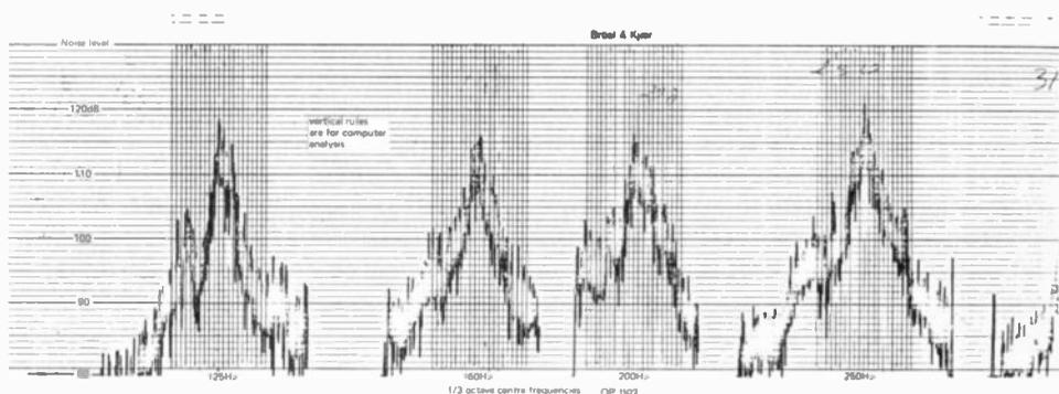
Fig. 7. Concorde 002: Approach Noise at 2 miles.
