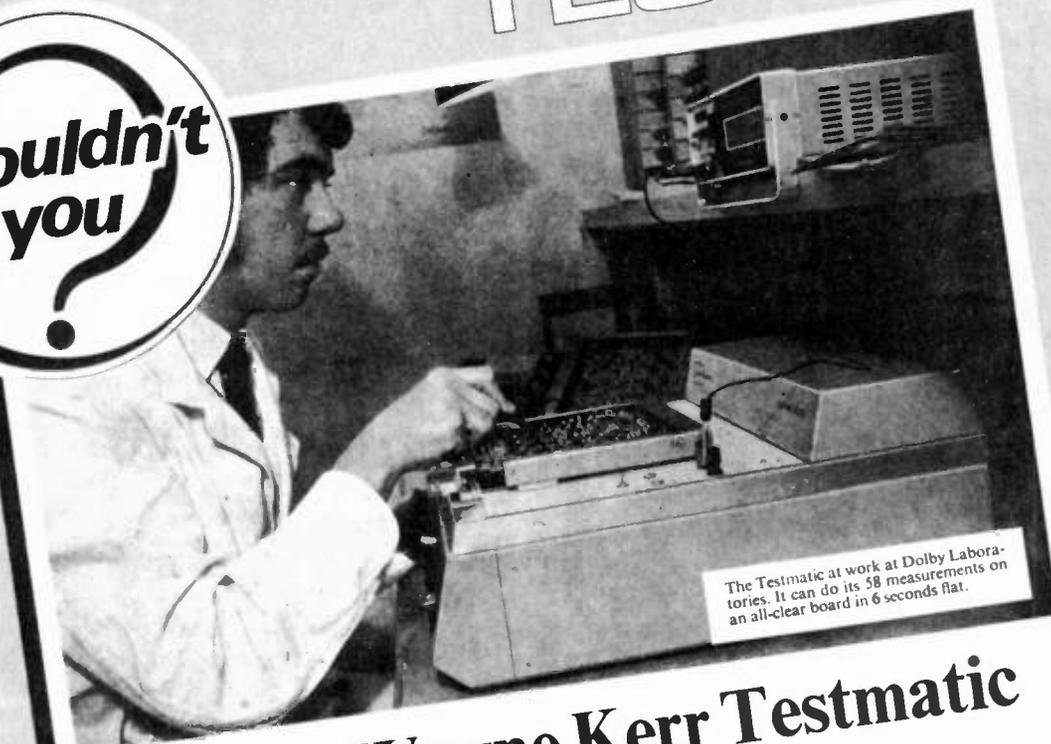
The Testmatic at work at Dolby Laboratories. It can do its 58 measurements on an all-clear board in 6 seconds flat.
