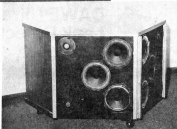
Fig. 1. First MARK I Quadreflect unit.
