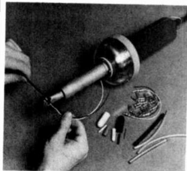
Shrink soldering with the LEISTER KOMBI Hot Air Gun which provides hot air up to 600°C. Variety of attachments, countless applications. Ask for brochure B1 from the Australian agents.
