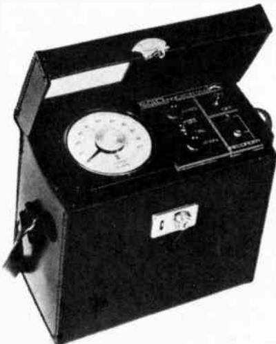
Transducers (CEL) have introduced a portable instrument for use with transducers based on the strain gauge principle for measuring pressure, load etc. Two versions of the instrument are available, one of which is powered from its own internal PP9 batteries and the other which uses the mains.
