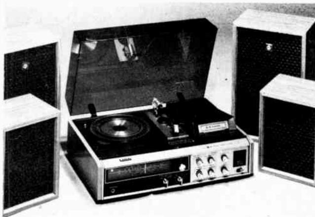
Typical of the British trend to 'unit/audio' is this 4-channel 'music centre' from Sanyo. Unit combines MW/FM stereo radio; 3-speed turntable, cartridge and stylus suitable for CBS SQ 4-channel discs; 8-track cartridge player capable of playing 4-channel discrete cartridges. Also included are two sets of speakers. (Model GXT 4731K).
