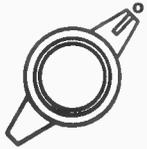
BATTERY CHECK. Shows operating hours remaining. When battery is low, automatic shut-off prevents wrong reading or battery damage.
