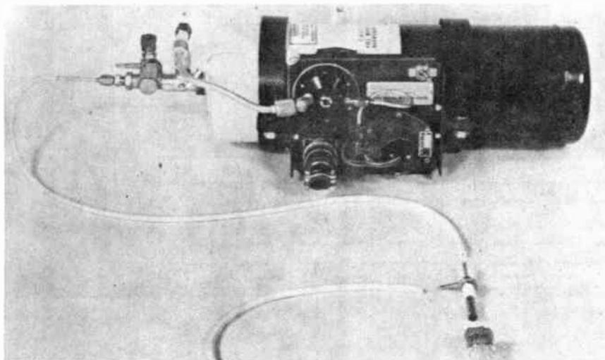
Fig. 4(a) Liquid nitrogen transfer system of SBRC. The standby time is 60 hr enabling a detector to be used virtually on demand.
