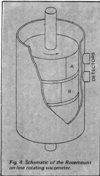
Fig. 4. Schematic of the Rosemount on-line rotating viscometer.
