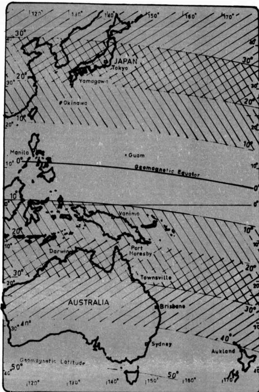
Fig. 2. Australasian sector of the world showing terminal zones for class I TEP (20° to 40° geomagnetic latitude) and class II TEP (10° to 30° geomagnetic latitude).
