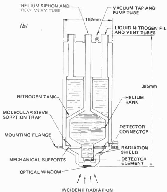
Fig. 3. Dewars used to cool infrared detectors: (a) A style 60A glass dewar made by SBRC. (b) Cross section of a Mullard stainless steel unit using helium.
