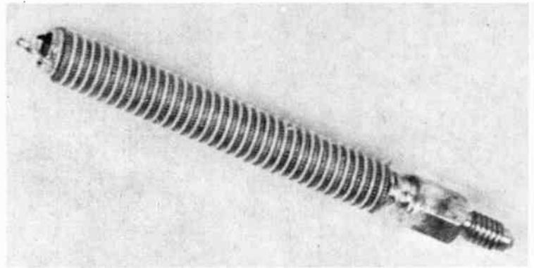
Fig. 4(b) A Joule-Thomson cryostat head. Cooling is by pressure release of argon or nitrogen gas.
