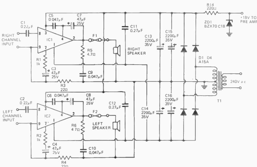
Fig. 1. Circuit diagram of main amplifier.
