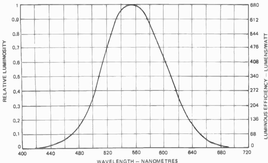
Fig. 1. Response curve of 'standard eye'.
