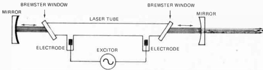
Fig. 8. Construction of a typical helium-neon laser. The gas mixture is contained in a glass tube and is excited by RF at 28 MHz or by a high voltage dc supply.
