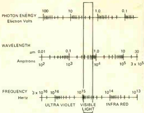
Fig. 1. Comparison of units used for electromagnetic radiation at optical frequencies. For example an energy change of 10 electron volts (ie  $V = 10^{-19}$  joules) produces radiation at 0.1 μmetres or 1000 angstrom, which is equivalent to a frequency of  $2 \times 10^{15}$  Hertz. Another SI preferred unit of wavelength is the nanometre = 1000 micrometres.
