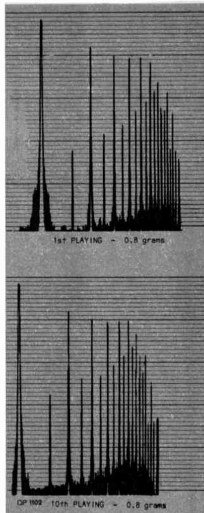
Fig. 1. Narrow Band Spectra of Square Wave Test Record on 1st playing and 10th playing with tracking weight of 0.8 grams.
