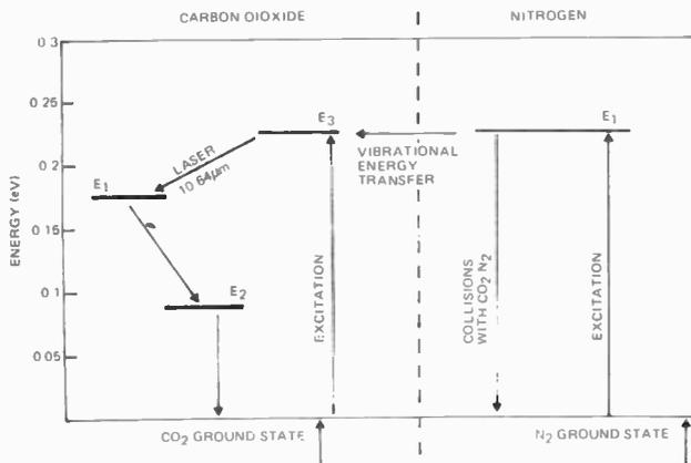
Fig. 10. Energy levels of a CO<sub>2</sub> laser.
