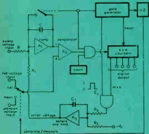
Fig. 1. Block diagram of A-to-D converter
