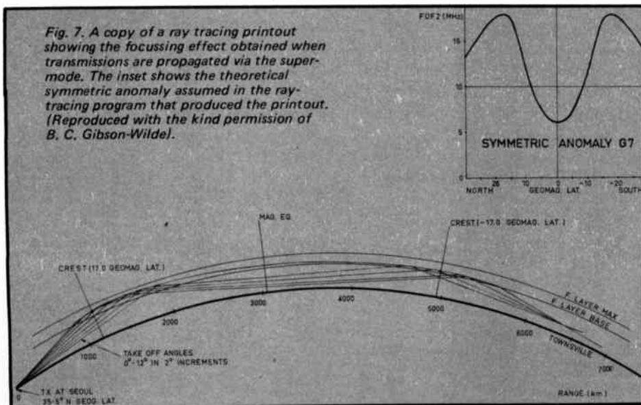
Fig. 7. A copy of a ray tracing printout showing the focussing effect obtained when transmissions are propagated via the supermode. The inset shows the theoretical symmetric anomaly assumed in the ray-tracing program that produced the printout. (Reproduced with the kind permission of B. C. Gibson-Wilde).
