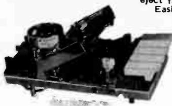
'VORTEX' Stereo Cassette Deck mechanism with Tape eject facility and resettable counter. Easily operated by 5 push-button (Piano key) controls, and includes High Quality "ALPS" recording or play-back head and erase head. Tape speed 4.75cm (1-7/8") sec. Plus or minus 1.5% Wow and flutter less than 0.25%. Operates on 250VAC. Fantastic value at only \$28.00 post free.
