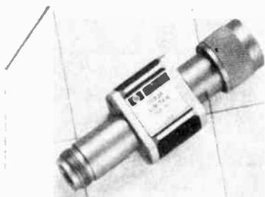
Sensitive microwave instruments can be protected from overload damage with a new limiter (Hewlett-Packard Model 11693A) which nonetheless has minimal effect on lower-level measurements. The 11693A typically introduces frequency response variations of less than  $\pm 0.5$  dB across the range 100 MHz to 12.4 GHz.
