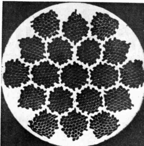
*Fig. 7. Cross section of Imperial Metals Industries superconducting cable. It has 1045 filaments held in a copper matrix.*
