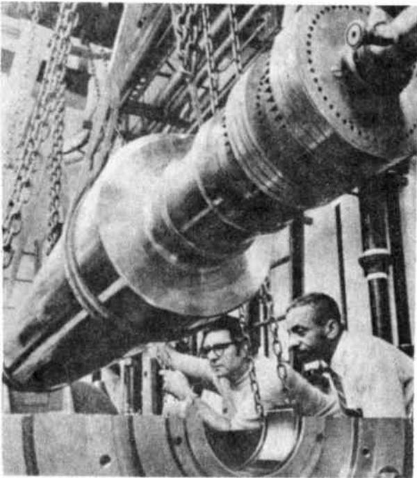
Fig. 8. Prototype 5MW superconducting rotor of a power generator made by Westinghouse.
