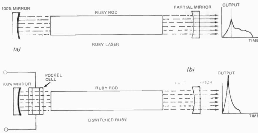
The "Q" switching technique prevents emission of laser pulses until higher population levels have been achieved. (a) shows conventional ruby laser and its typical output pulse shape. (b) shows method of inserting Pockel cell and the resulting increased peak power of the pulse.
