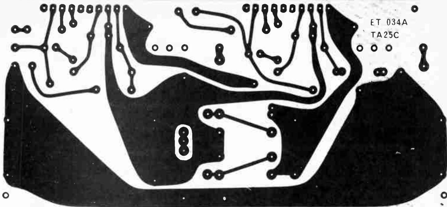
Fig. 2. Printed circuit board for main amplifier (shown full size).
