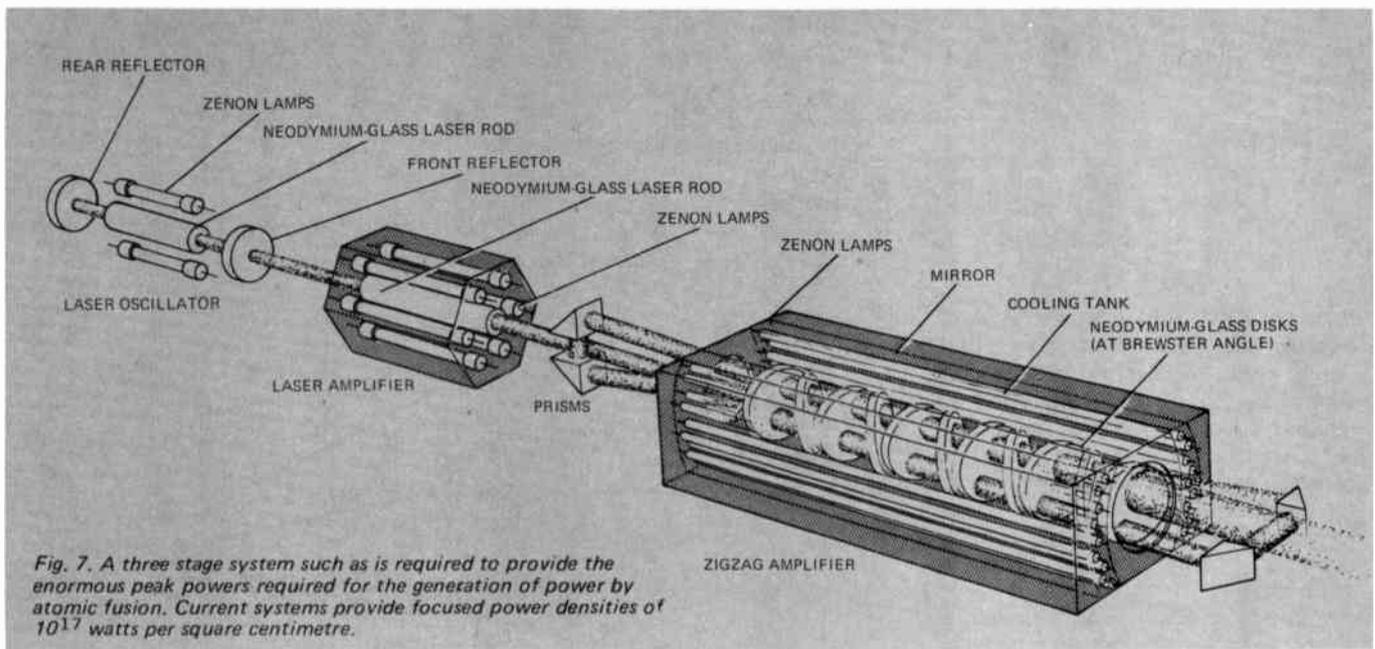
base material in rod form containing up to 2% of another impurity material which produces the laser action.
