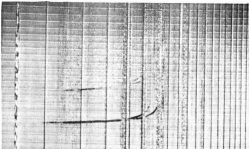
Fig. 5. (a) Vertical incidence ionogram from Cocos Island, 1900 hrs LMT, 5th August 1970, showing typical F-layer trace without range-spreading.
