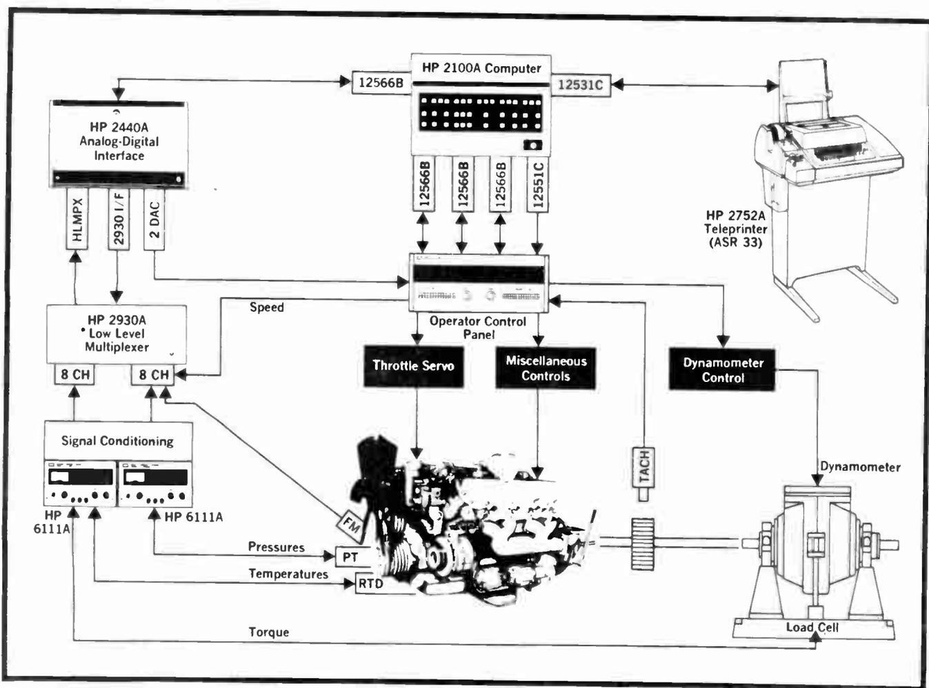
Fig. 7. HP9600 data acquisition and control system applied to engine testing.
