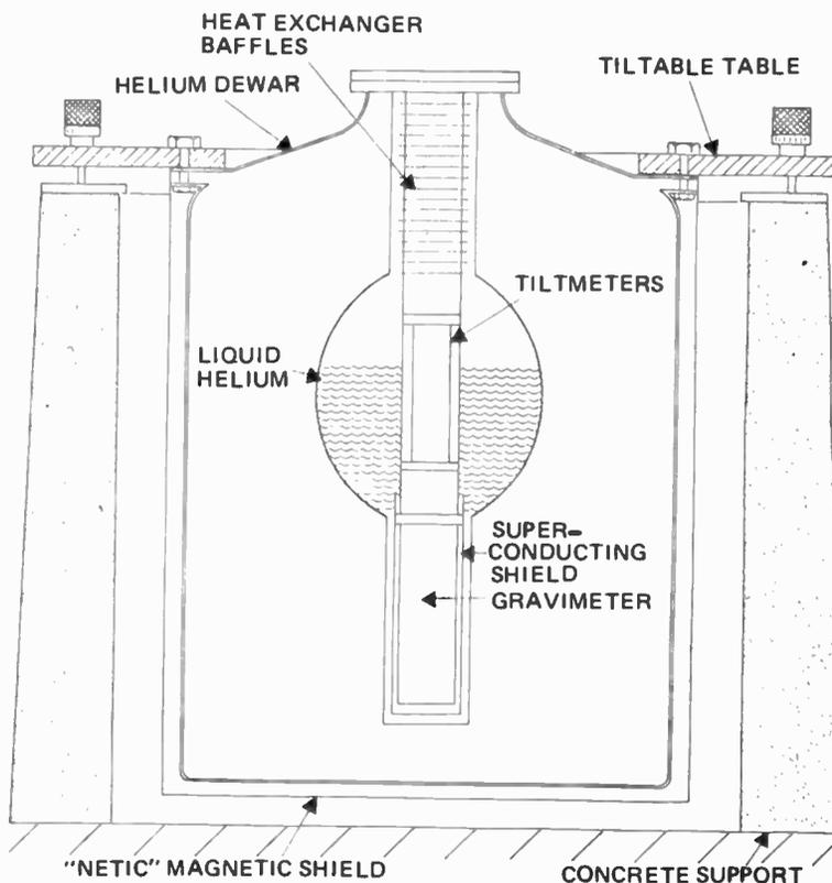
Fig. 10. Cross-section of a superconducting gravity meter installation. The tilt meters are used to correct records for inclination.
