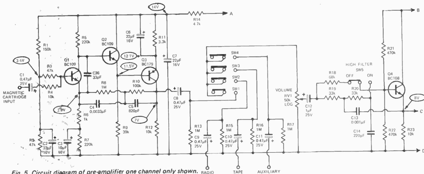
Fig. 5. Circuit diagram of pre-amplifier one channel only shown.
