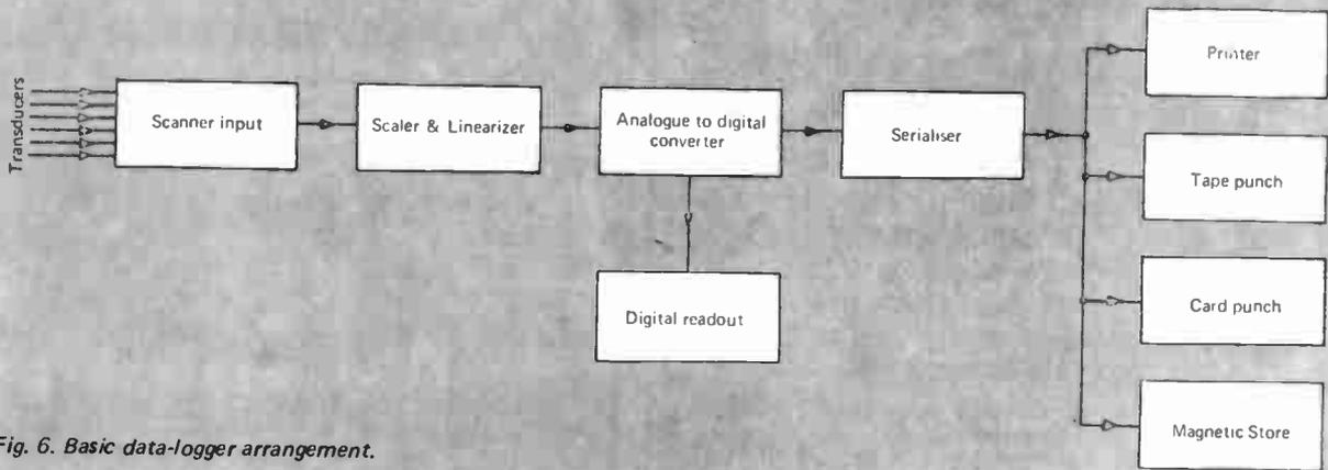
Fig. 6. Basic data-logger arrangement.
