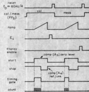
Fig. 4. Circuit waveforms.
