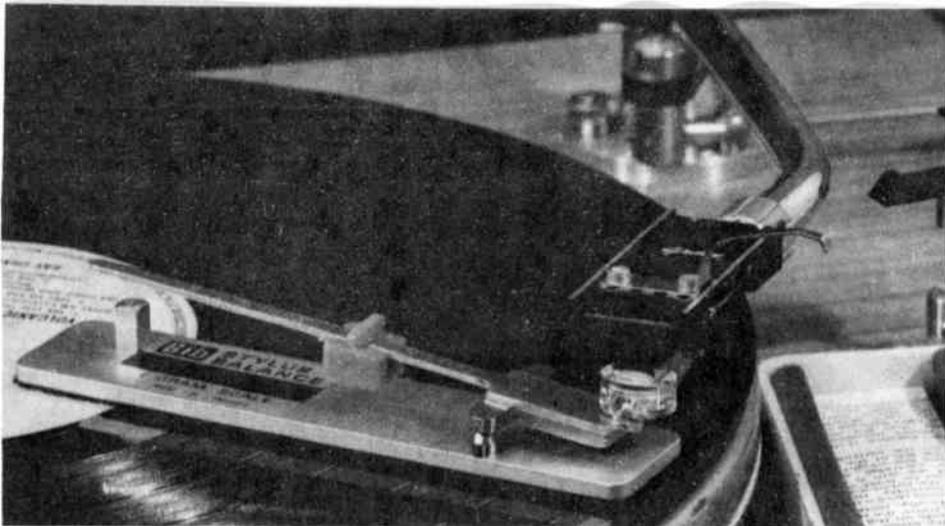
Tracking weight may be set very accurately using stylus balances such as shown here.
