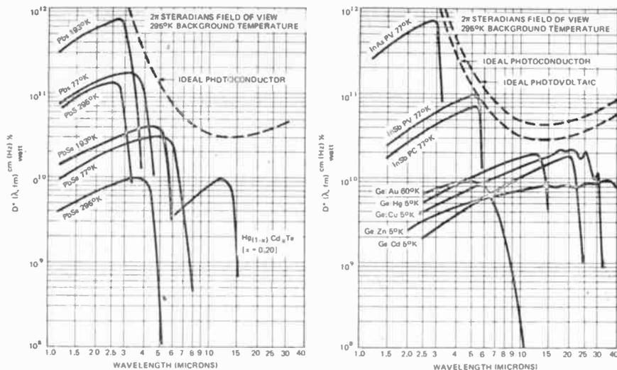
Fig. 2. Sensitivity of infrared detectors depends upon the temperature of the element as shown by these curves of Santa Barbara Research Centre (SBRC) devices.
