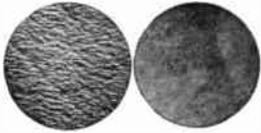
TDK particles are densely and uniformly packed into the tape coating. Mirror-smooth lubricated surface means less wear on the recorder head.
