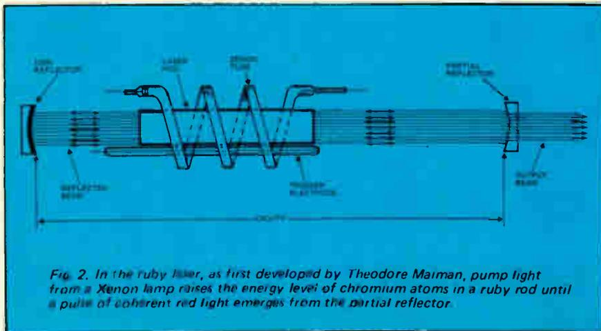
Fig. 2. In the ruby laser, as first developed by Theodore Maiman, pump light from a Xenon lamp raises the energy level of chromium atoms in a ruby rod until a pulse of coherent red light emerges from the partial reflector.
