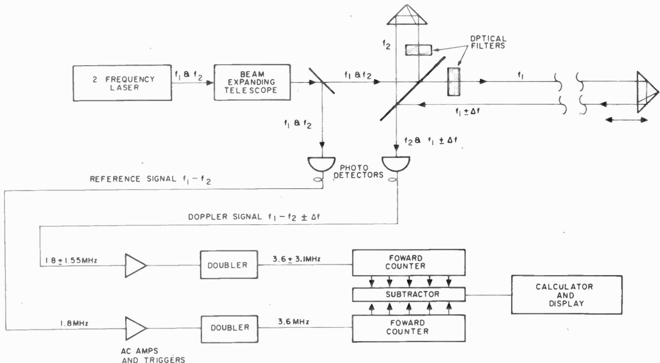
An important application of helium-neon lasers is in distance and velocity measurements by interferometric techniques. This system, the Hewlett Packard model 5525A is capable measuring length with an accuracy of  $\pm 0.000\ 001$  inch over 200 feet.
