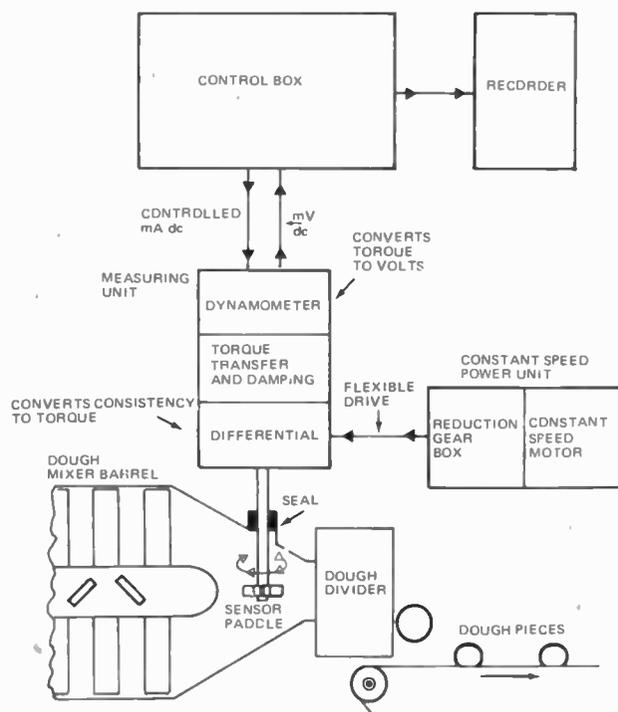
Fig. 5. Basic system components of consistency measuring instruments used in automated bread making.
