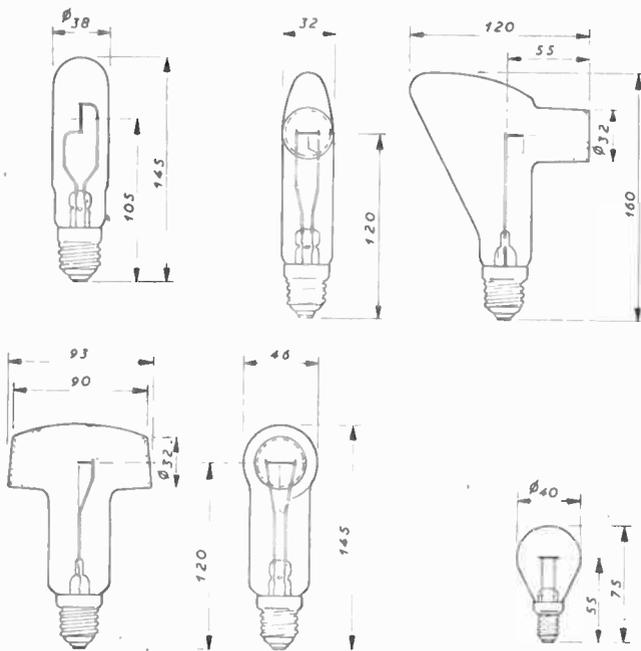
Fig. 2. Tungsten ribbon lamps especially designed to produce a uniformly radiating surface. The windows are ground plane-parallel from quartz or heat-resisting glass and must have their spectral energy transmission calibrated before manufacture.
