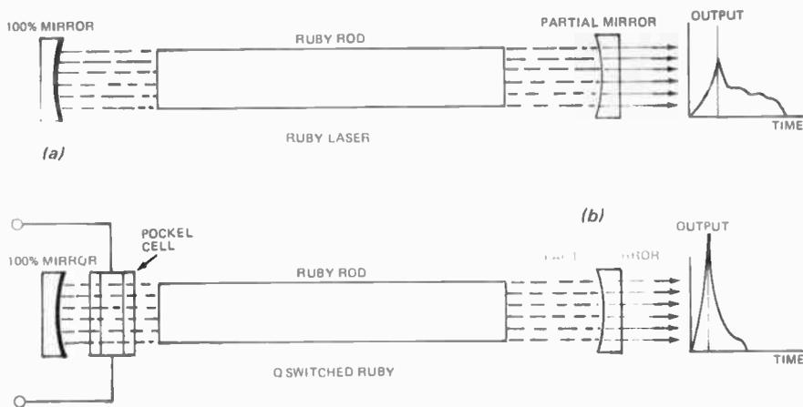
The "Q" switching technique prevents emission of laser pulses until higher population levels have been achieved. (a) shows conventional ruby laser and its typical output pulse shape. (b) shows method of inserting Pockel cell and the resulting increased peak power of the pulse.
