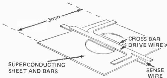
Fig. 11. The Crowe superconducting memory cell. The main disc is lead and all elements are superconductors.
