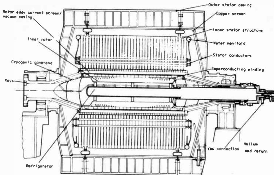
500 MW superconducting AC generator designed at IRD.
