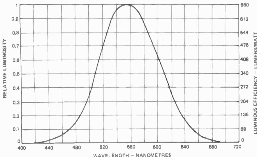
Fig. 1. Response curve of 'standard eye'.
