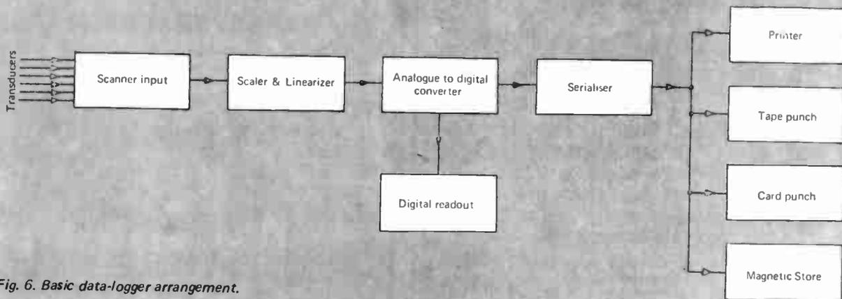
Fig. 6. Basic data-logger arrangement.
