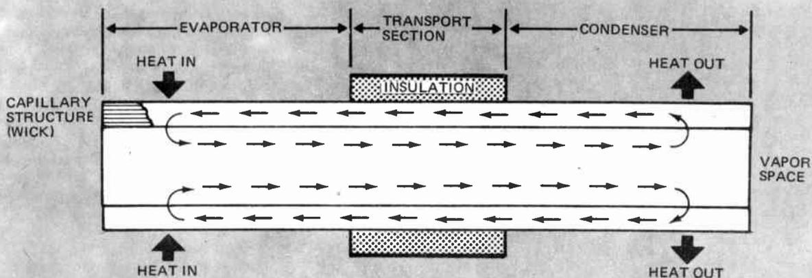
Fig. 6. Schematic of a two-phase heat pipe.
