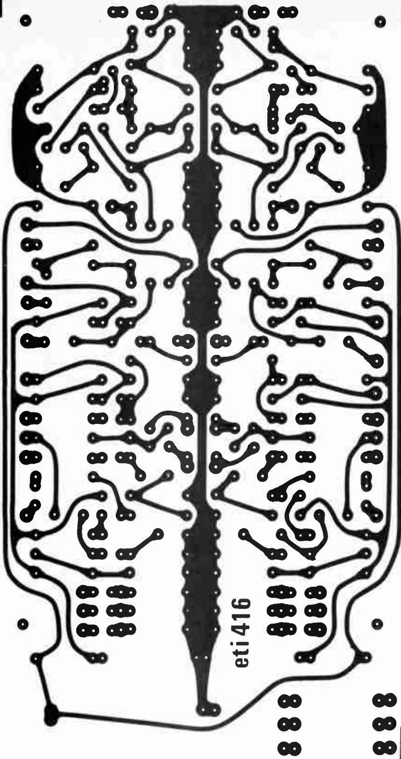
Fig. 6. PC board for pre-amplifier (both channels)
