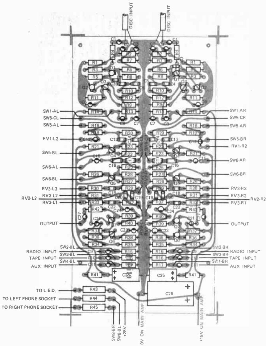
Fig. 7. Component overlay — pre-amplifier
