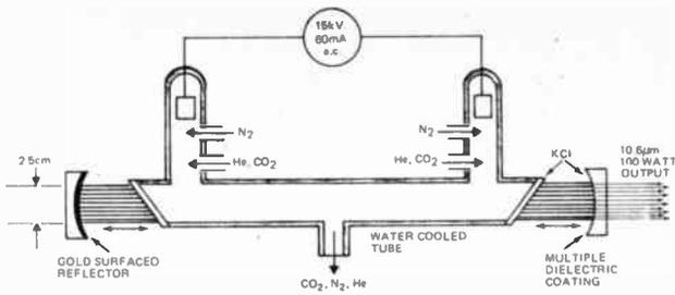
Fig. 11. Typical 100 watt CO<sub>2</sub> laser removes heat by flowing gases through the laser tube.
