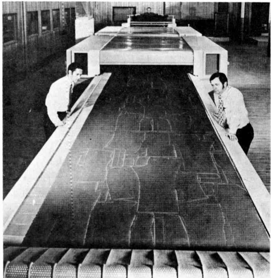
*Cloth being cut at high speed to complex patterns by a computer controlled laser beam.*
