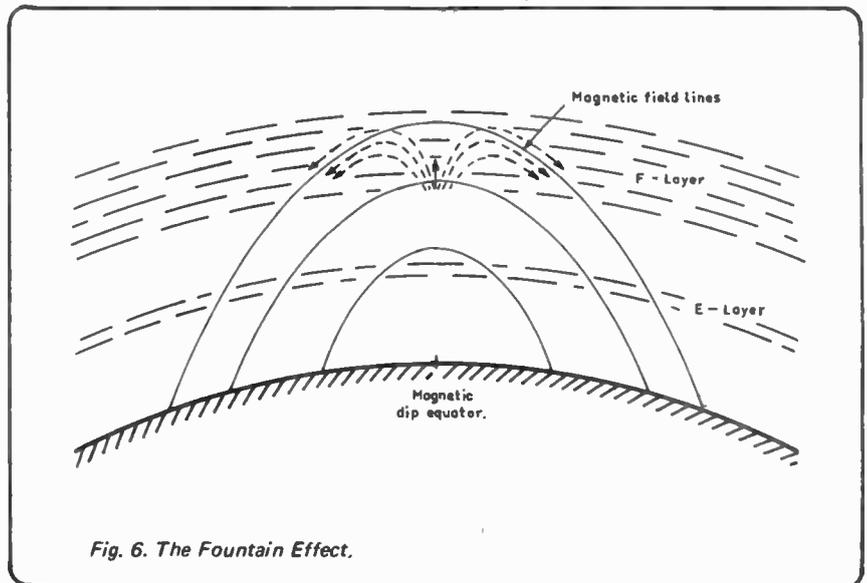
considerable amount of flutter. The flutter rate is mostly between 5 and 15Hz and Doppler shift is mainly between  $\pm 40$ Hz. This means that, at times, A3 (DSB or SSB) signals will be seriously degraded. The effect on wideband systems (FM or PM) would be much less but TV would suffer owing to the spread of time delays experienced.
