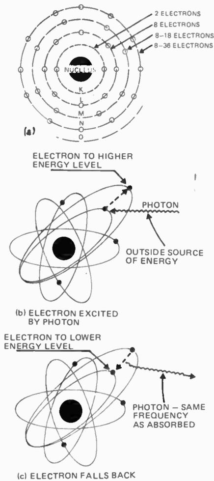
Fig. 3. (a) Simplified diagram (not typical of any particular element) of orbital levels of an atom. These levels are known as shells and are the only possible orbits.
