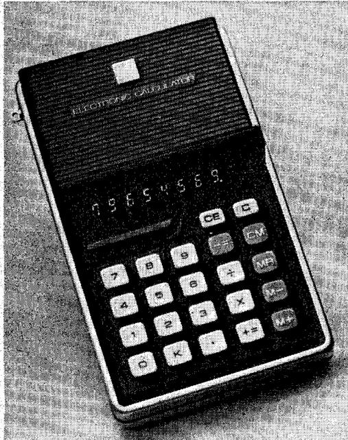
Sharp's ELS1 814 has full memory 8 digit display and very low battery drain due to the use of CMOS logic.
