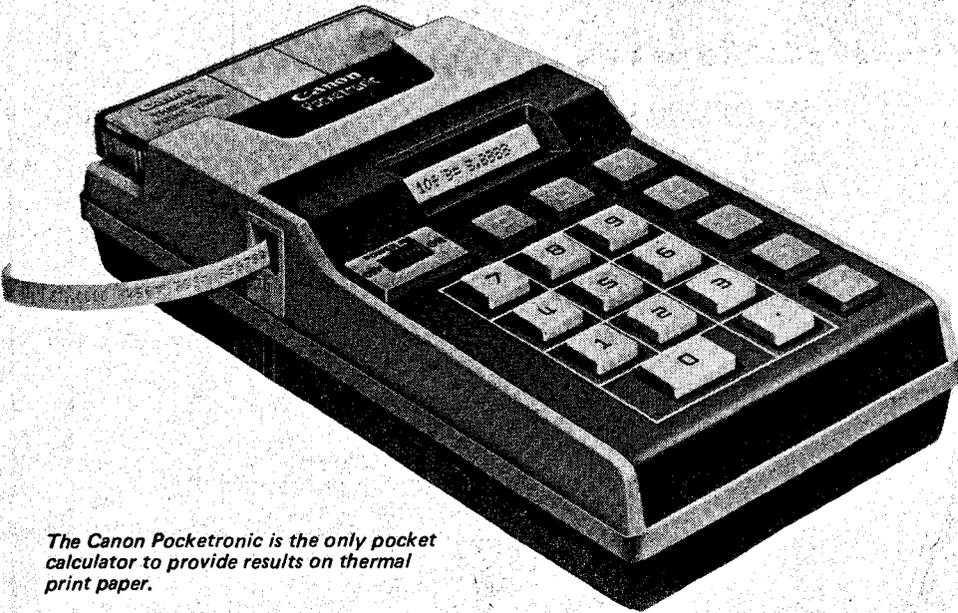
The Canon Pocketronic is the only pocket calculator to provide results on thermal print paper.
