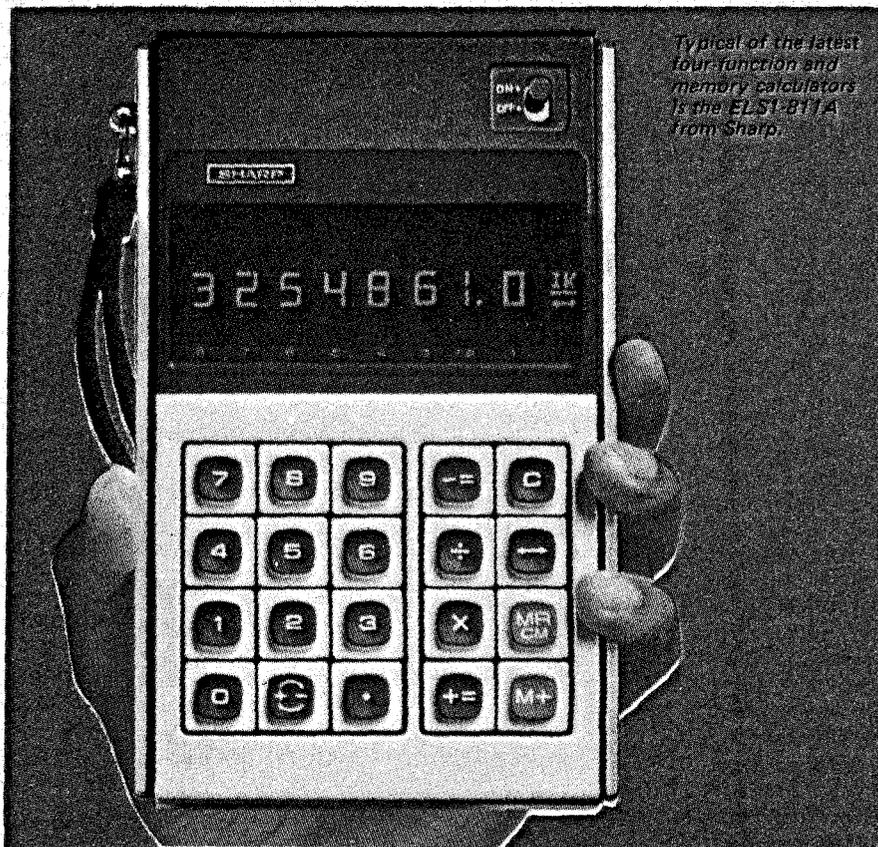
Typical of the latest four-function and memory calculators is the EL51-B11A from Sharp.
